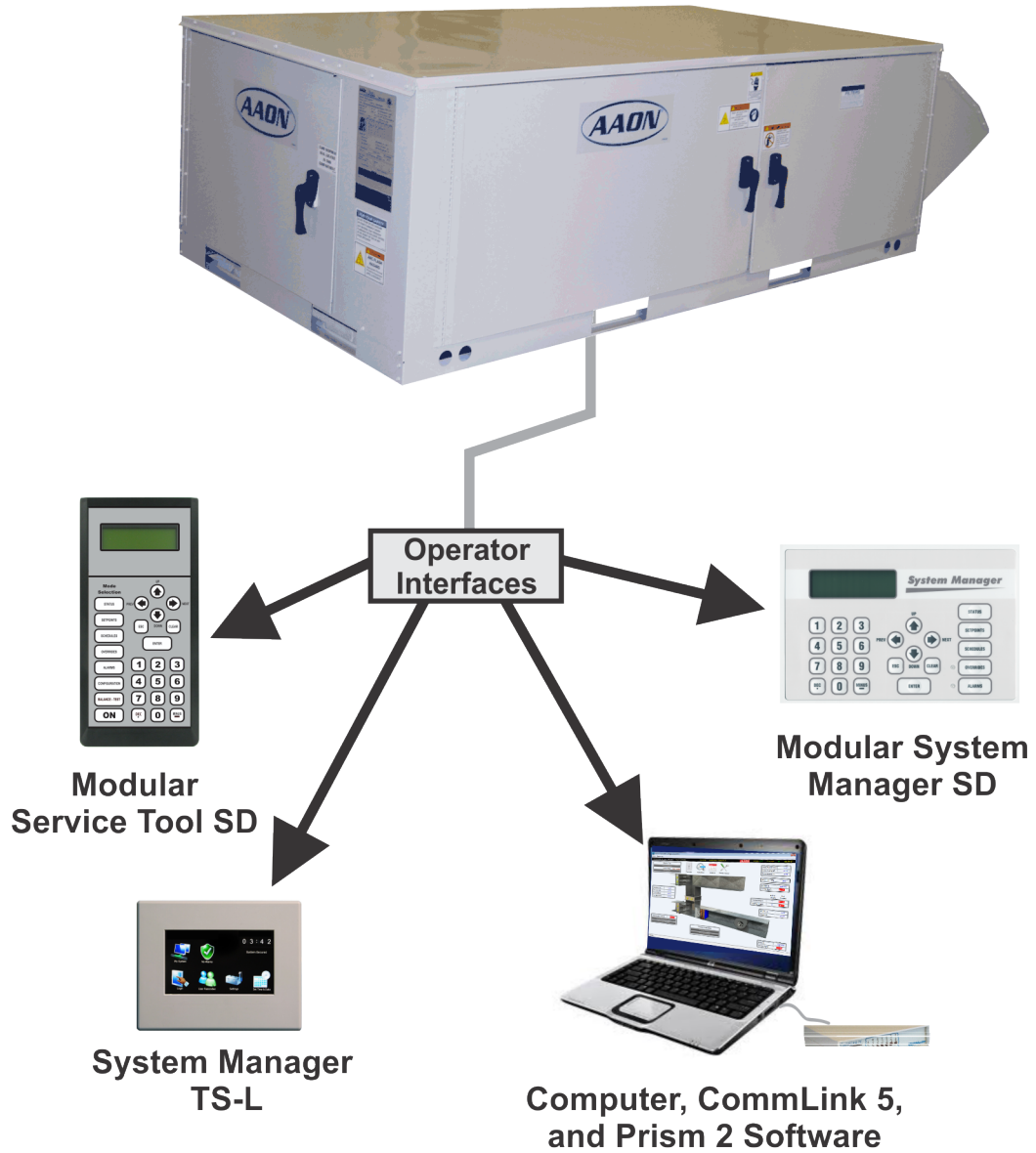
Figure 21: Typical Stand-Alone System Layout
