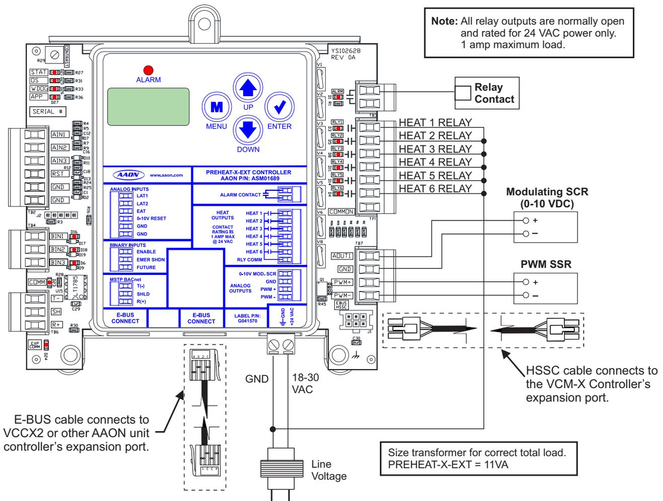
**Figure 3: PREHEAT-X-EXT Outputs Wiring**
