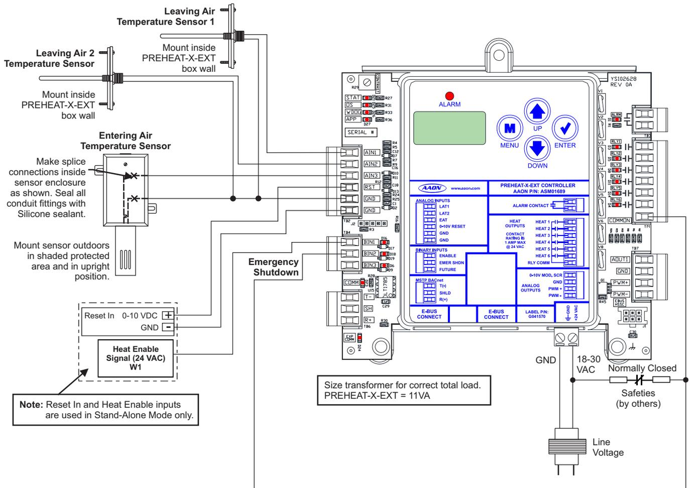
**Figure 2: PREHEAT-X-EXT Inputs Wiring Diagram**
