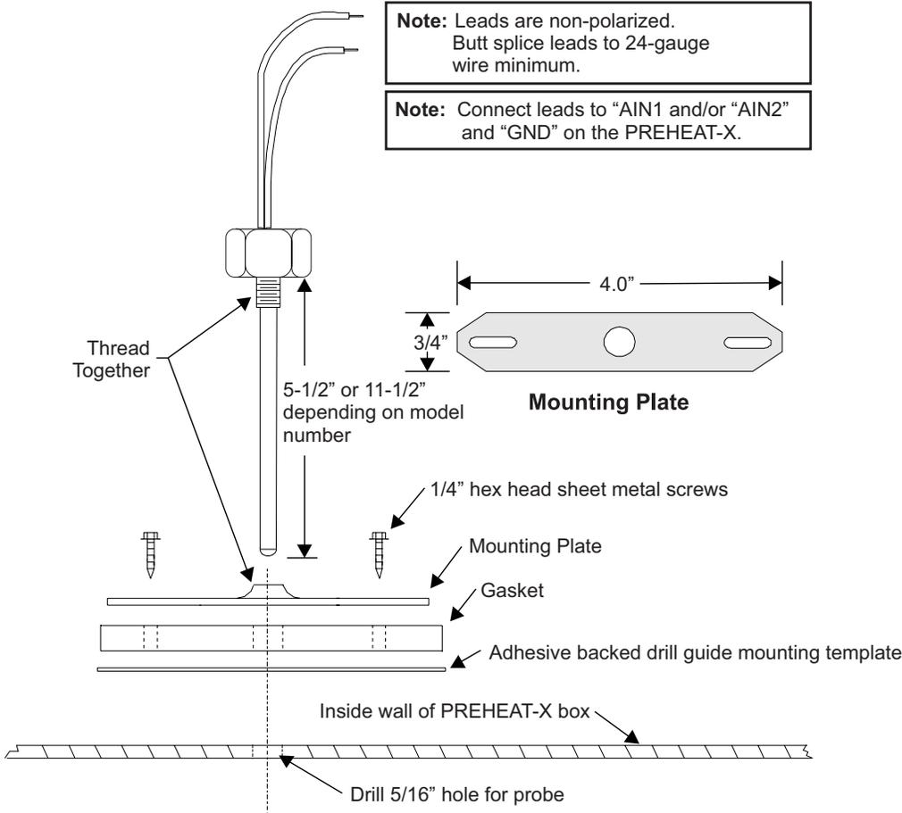
**Figure 7: Leaving Air Temperature Sensor Installation**
