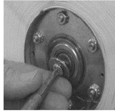
Figure 52: Remove Center Screen from Wheel Shaft
