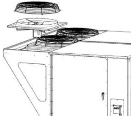
Figure 49 — Removal of a Condenser Fan Assembly
