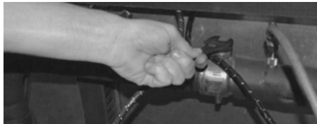
Figure 51 — Remove bolts from suction filter
