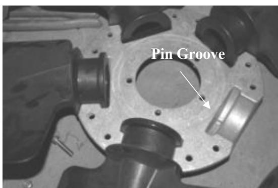
Figure 34 — Pin Groove Location
