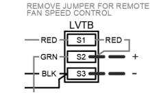
Figure 20 - Shows the jumper that is to be removed (jumped between S1 and S2).
