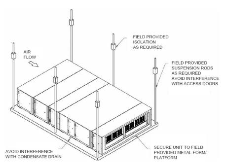
Figure 4 - H3 Series Platform Suspension Installation
