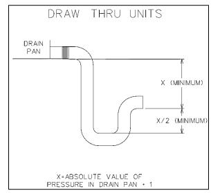
Figure 17 - Drain Trap
