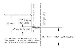
Figure 26 - Hot Gas Purge Circuit
