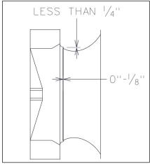
Figure 18 - Plenum Fan Gap Tolerances
