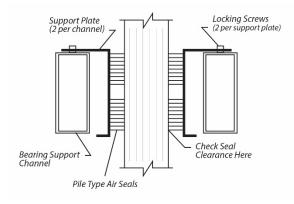
Cross Section of Air Seal Structure
