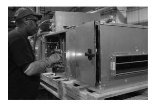
Apply 13 mm (½") thick, 16 mm (5/8") wide adhesive gasket around the edges of the box without the flanges.
