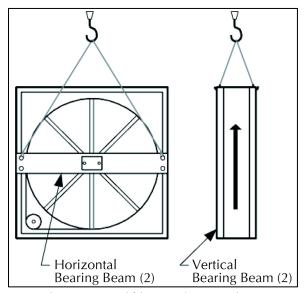
Figure 28 - Lifting Hole Locations
