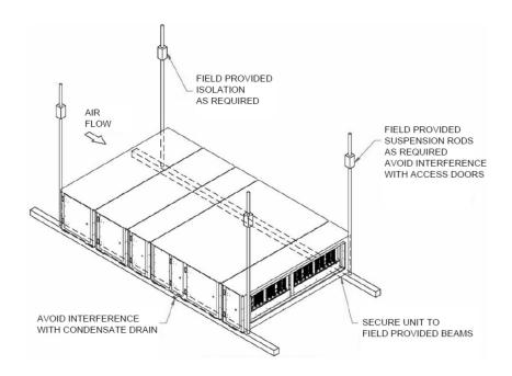
Figure 5 - H3 Series Parallel Beam Suspension Installation
