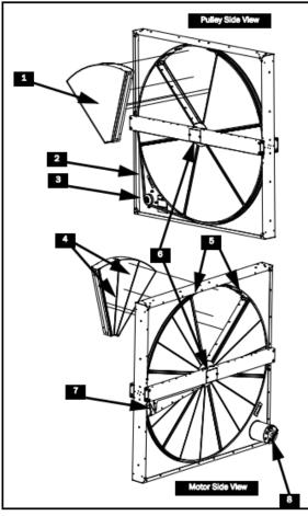
Figure 29 - Polymer Energy Recovery Wheel
