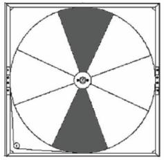
Figure 30 - Wheel Segment Removal Pattern
