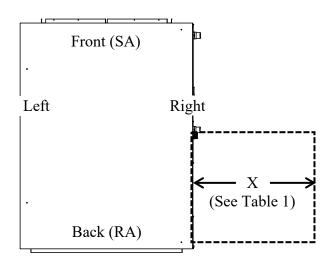
Figure 2 -Minimum Clearance Required for Access to Unit (H3 Series plan view)
