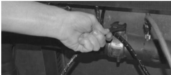
Figure 26: Close the Isolation Valves around the Suction Filter
