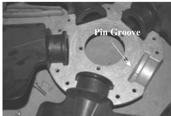
Figure 34 — Pin Groove Location
