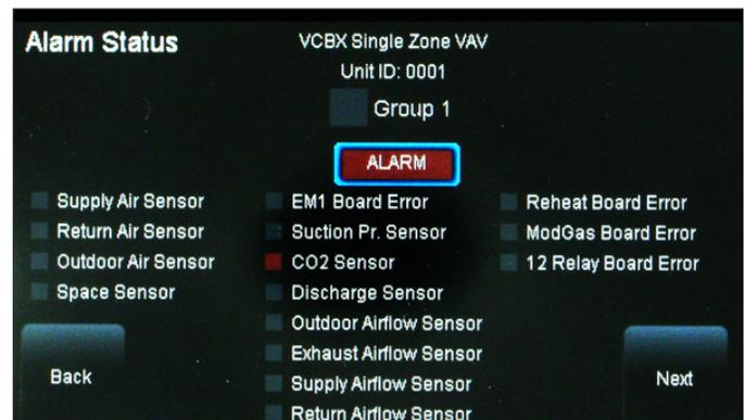
**Figure 25: VCB-X Controller Alarm Screen**
