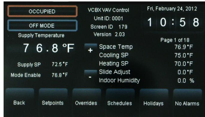
**Figure 19: VCB-X Controller Status Screen 1**
