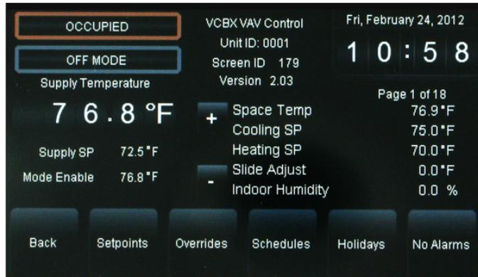
**Figure 33: VCB-X Controller Status Screen**
