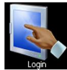
Touch the **<Login>** icon found on bottom left of the *Main Screen* and type the default Level 3 passcode of "3333" using the number keypad to gain access to all setpoint and configuration items. See **Figure 10**.
