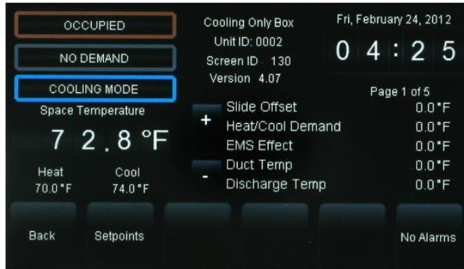
**Figure 40: VAV/Zone Controller Status Screen**
