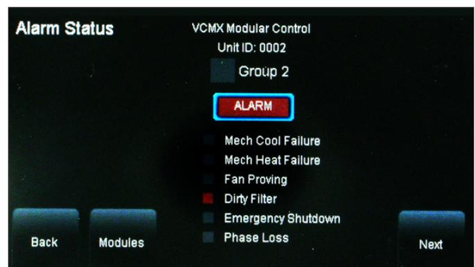
**Figure 22: VCM-X Controller Alarm Screen**
