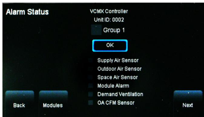
**Figure 21: VCM-X Controller Alarm Status Screen**
