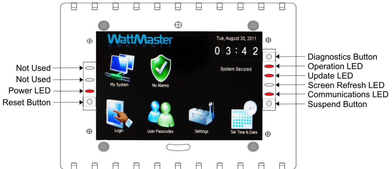
**Figure 44: System Manager TS II LEDs & Buttons**
