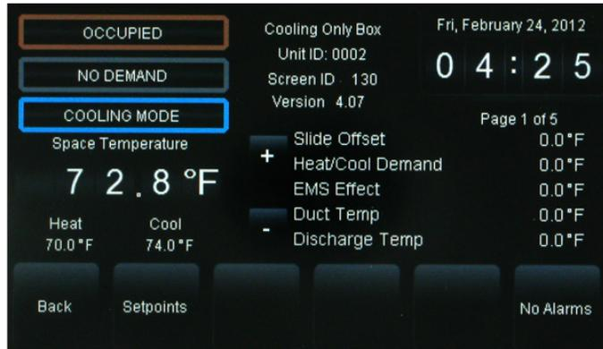
Figure 37: VAV/Zone Controller Status Screen
