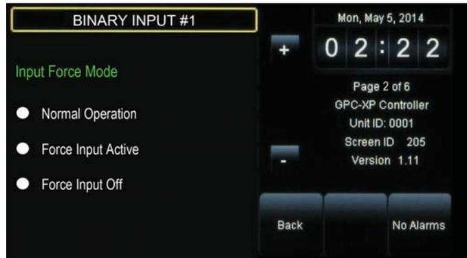
Figure 19: Binary Input Force Mode Screen
