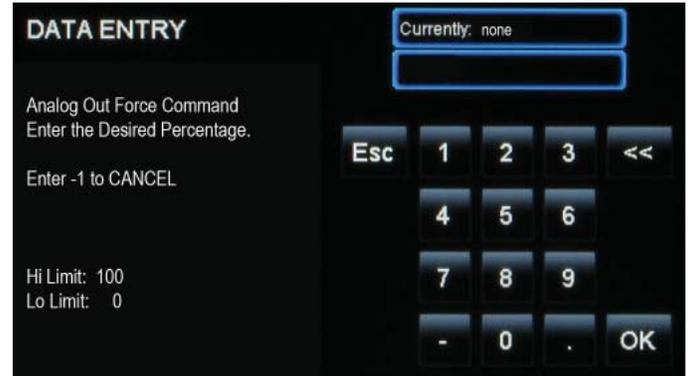
**Figure 25: Analog Output Force Screen**
