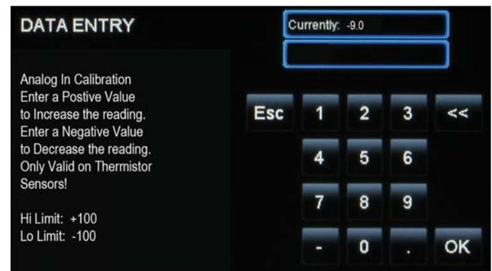
**Figure 16: Calibrate Sensor Data Entry Screen**
