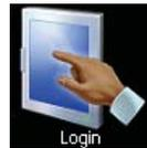
Touch the <Login> icon found on bottom left of the *Main Screen* and type the default Level 3 passcode of “3333” using the number keypad to gain access to all setpoint and configuration items. See **Figure 7**.
