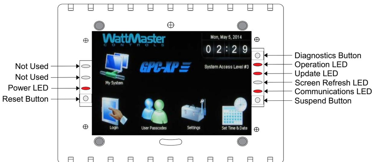
**Figure 36: System Manager TS II LEDs and Buttons**
