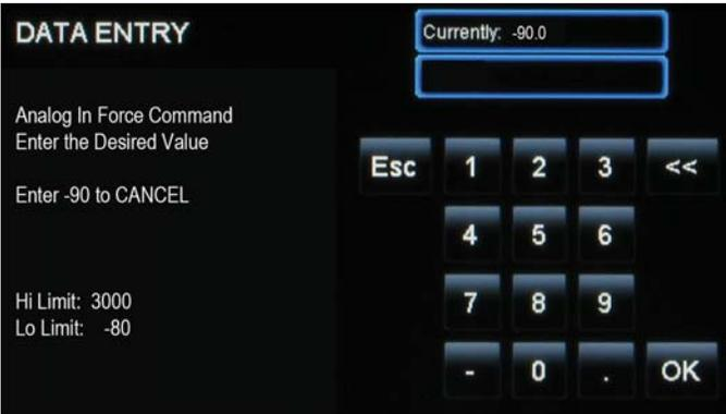
Figure 17: Sensor Override Data Entry Screen
