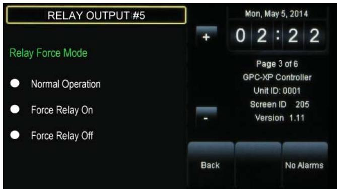
**Figure 22: Relay Output Force Mode Screen**
