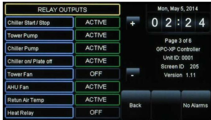
Figure 20: Relay Outputs Screen
