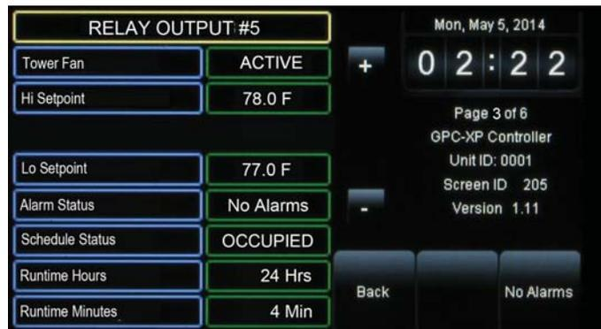
Figure 21: Relay Output Details Screen
