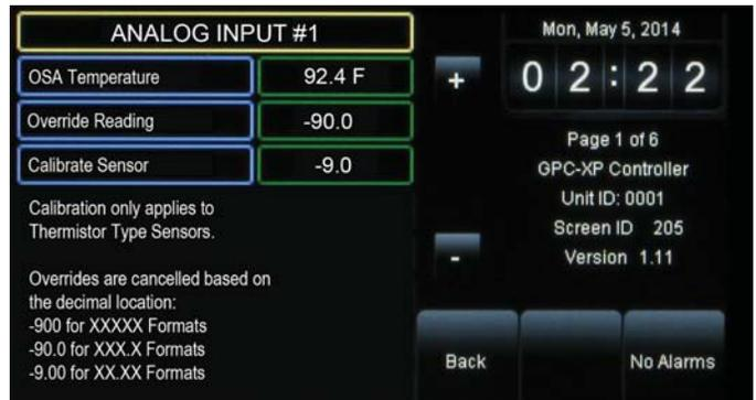
**Figure 15: Analog Input Details Screen**
