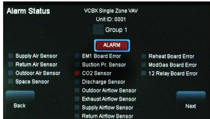
**Figure 25: VCB-X Controller Alarm Screen**
