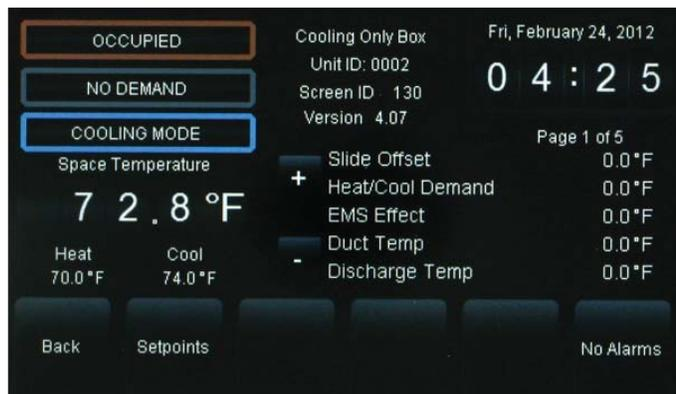
**Figure 40: VAV/Zone Controller Status Screen**
