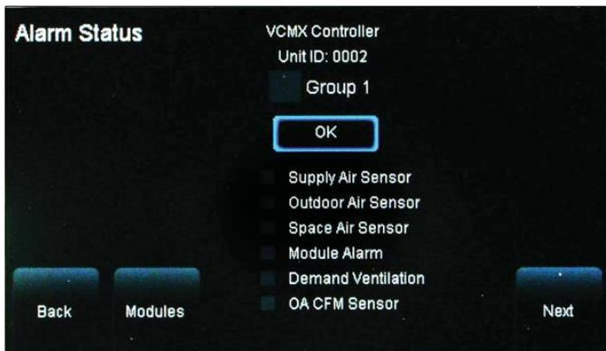
Figure 21: VCM-X Controller Alarm Status Screen
