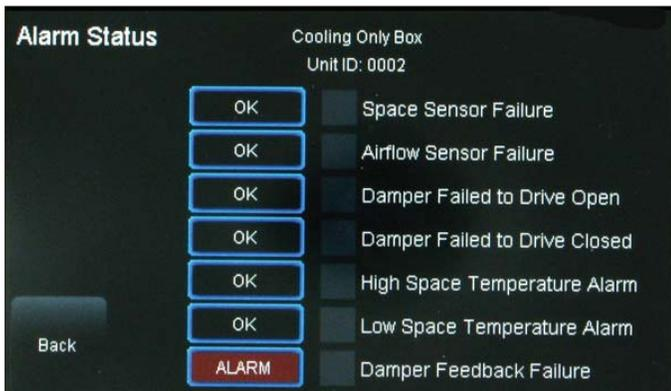
**Figure 38: VAV/Zone Controller Alarm Status Screen**
