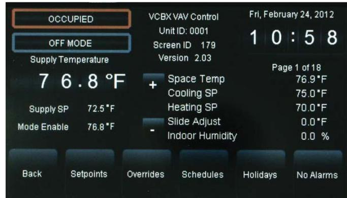
**Figure 19: VCB-X Controller Status Screen 1**
