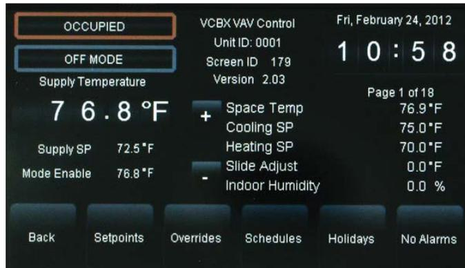
**Figure 33: VCB-X Controller Status Screen**
