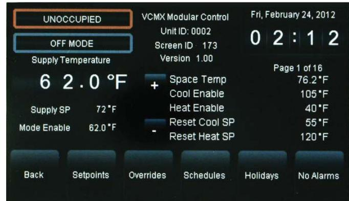
**Figure 18: VCM-X & VCM-X Modular Controller Status Screen 1**
