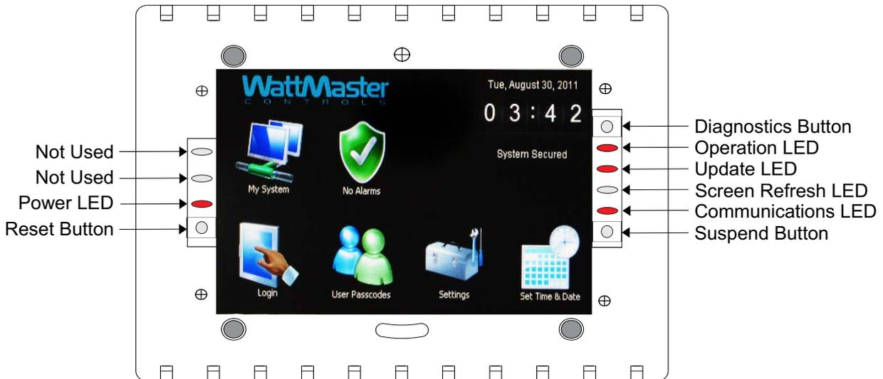
**Figure 44: System Manager TS II LEDs and Buttons**
