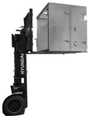
Figure 8: M2 Series Individual Module Top Tier Lifting
