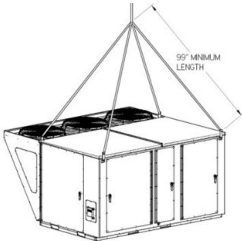
Figure 8 – Lifting Details of a 6-25 and 30 ton Standard or Power Exhaust Unit
