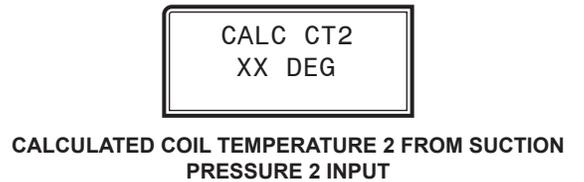
CALCULATED COIL TEMPERATURE 2 FROM SUCTION PRESSURE 2 INPUT
