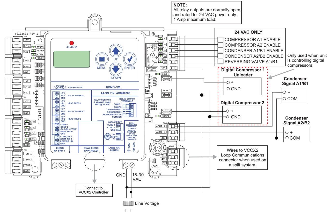
Figure 14: A1/B1 Wiring
