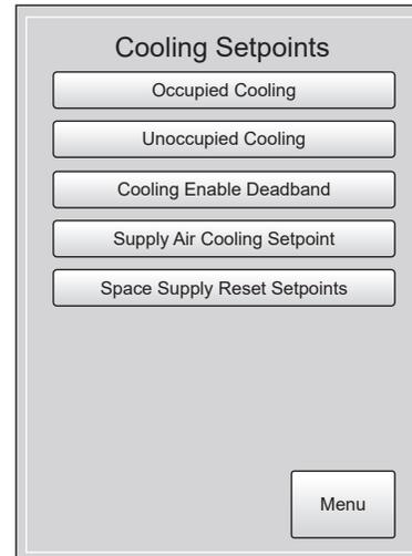
**Figure 2-14: Cooling Setpoints Screen**
