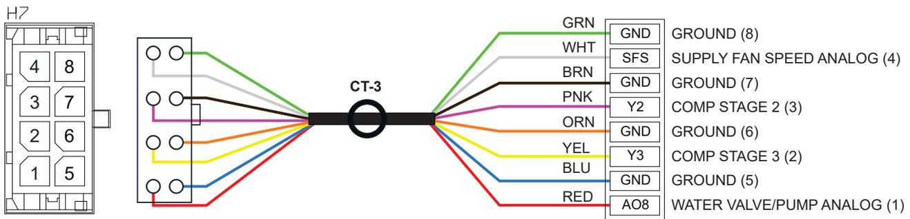
Figure 1-6: H7 Variable Capacity Harness Wiring
