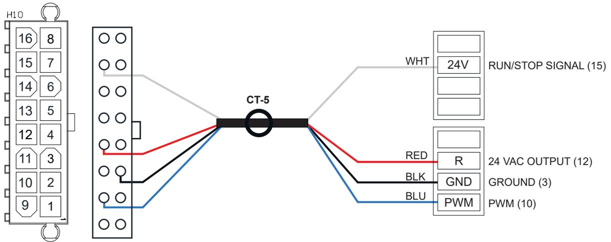
**Figure 1-8: H10 WSHP Harness Wiring**
