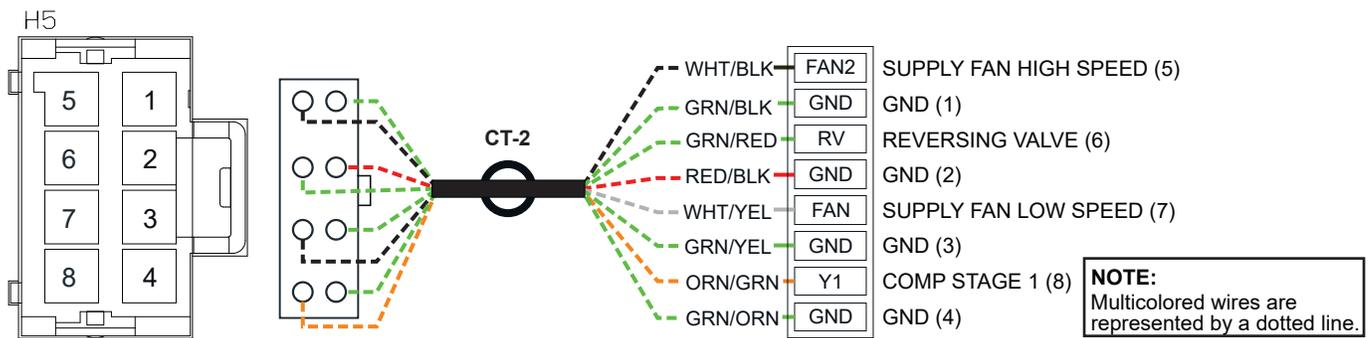
Figure 1-5: H5 Standard Output Harness Wiring
