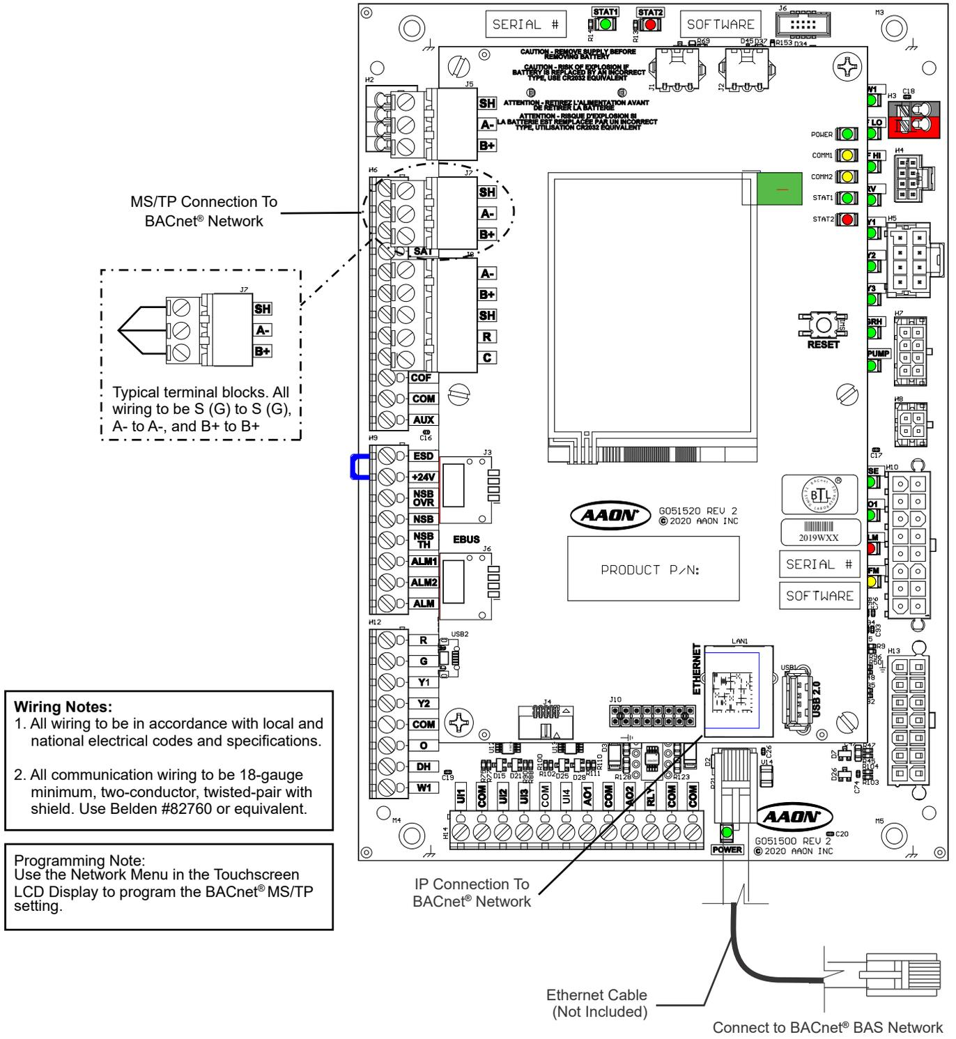
Figure 1-15: BACnet® Connection to MS/TP Network or IP BAS Network (ASM02323 Only)
