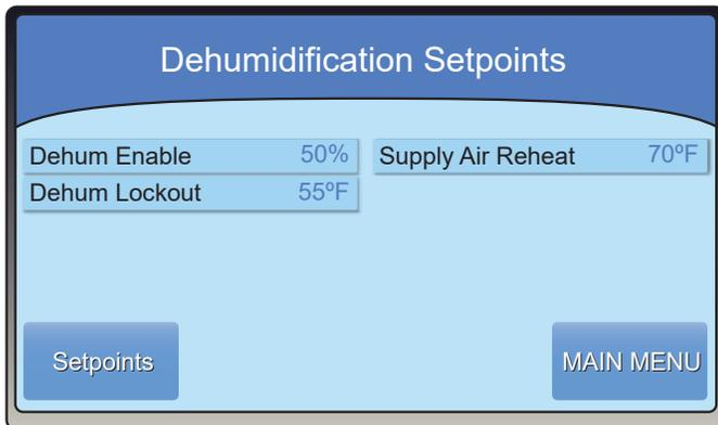
Figure 4-8: Setpoints - Dehumidification
