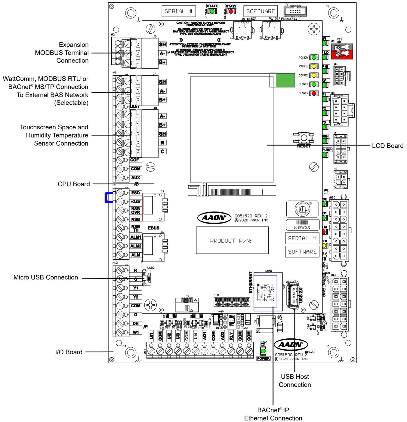
Figure 1-1: Pioneer Gold Controller Connection Components, Jumper and Switches
