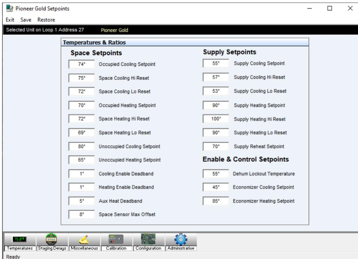
Figure 3-3: Temperature & Ratios Setpoints Screen
