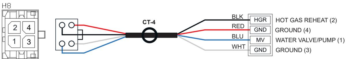
Figure 1-7: H8 Reheat and Water/Valve Pump Harness Wiring
