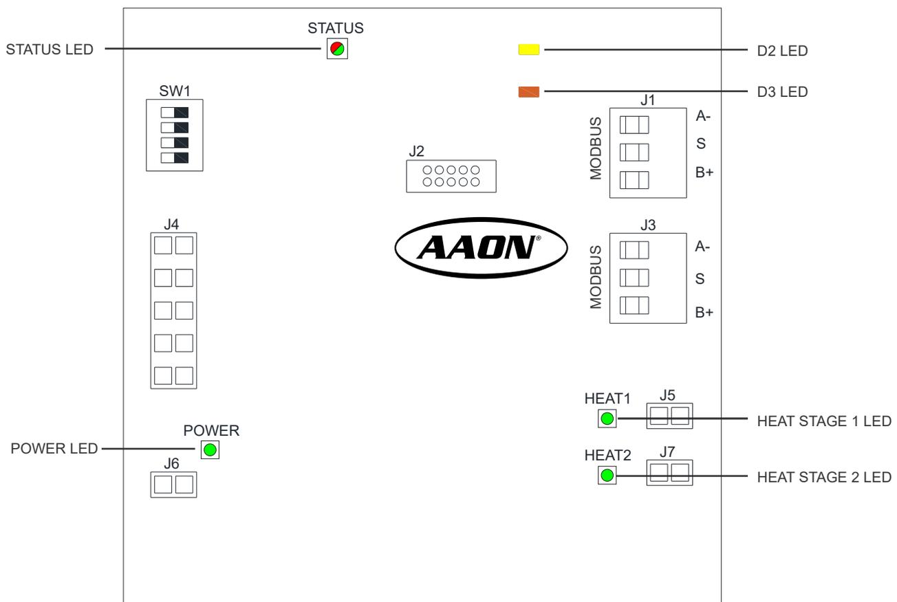
Figure 1-13: Pioneer Gold Electric Heat Board LED Locations
