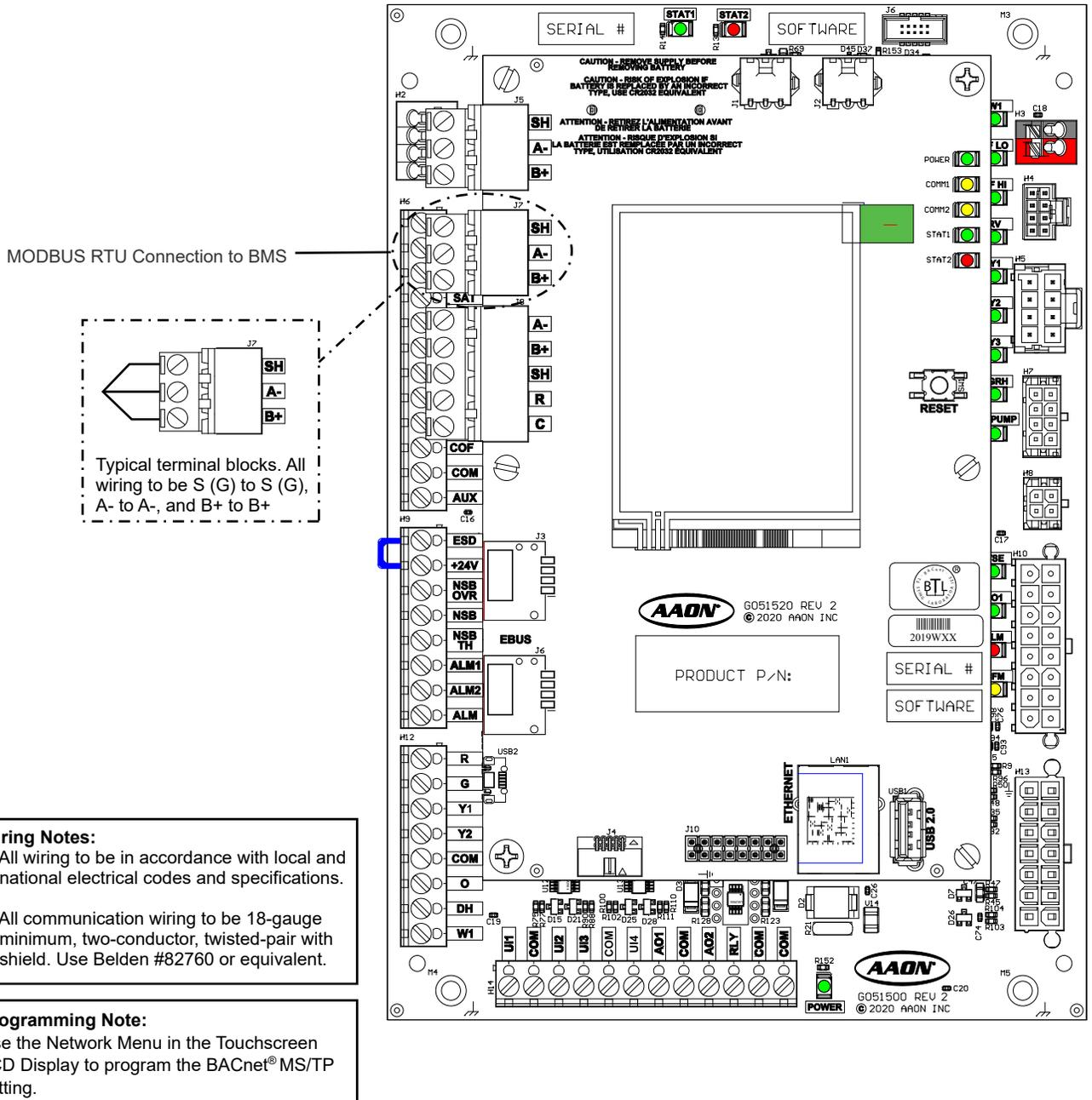
Figure 1-16: MODBUS TRU Connection to BMS
