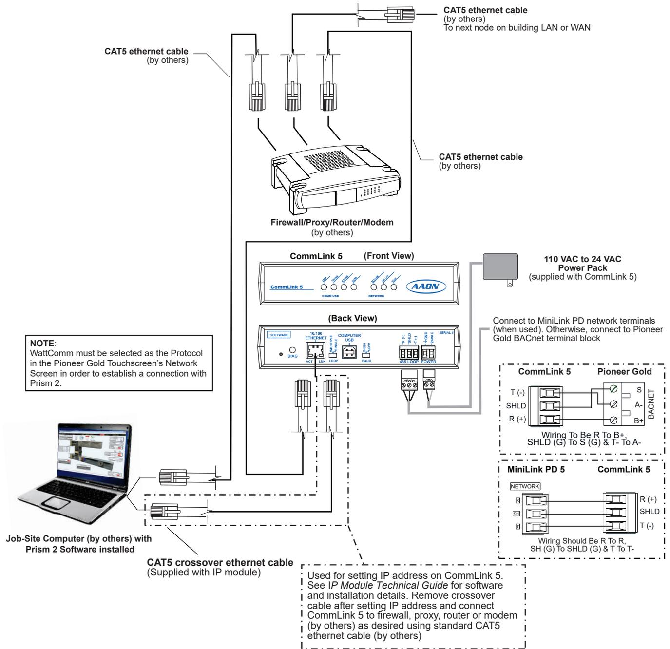
Figure 3-23: IP Module Connection
