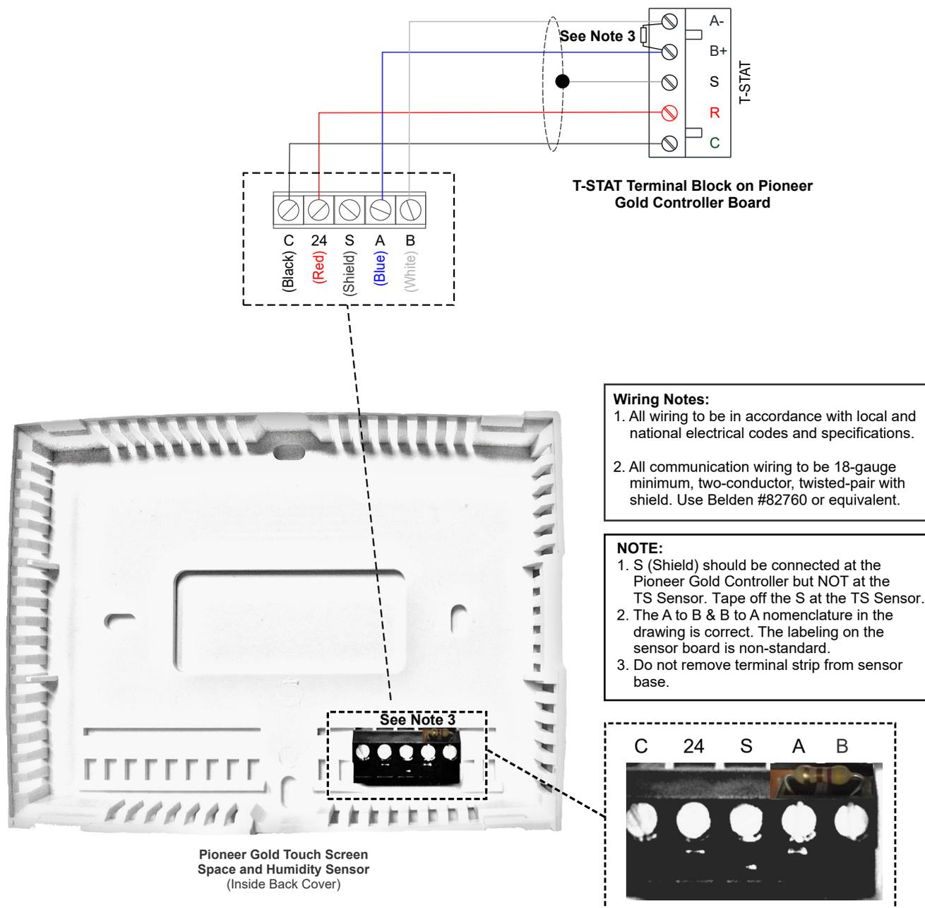
**Figure 1-11: Pioneer Gold Touchscreen Space and Humidity Sensor Wiring**
