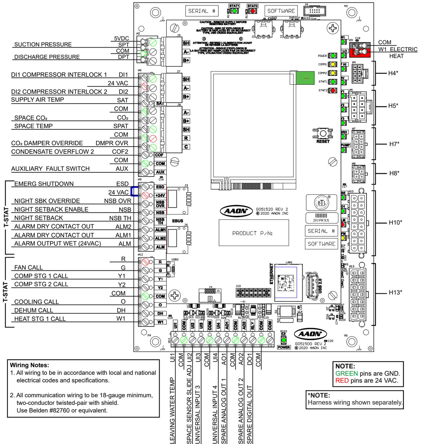
Figure 1-3: Pioneer Gold Controller Wiring
