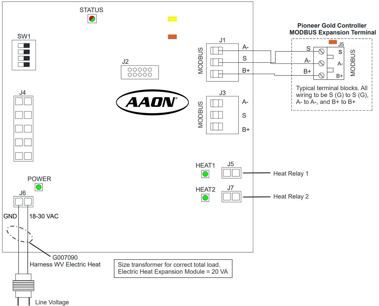
Figure 1-10: Pioneer Gold Electric Heat Board Components and Wiring
