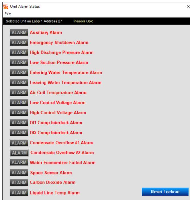
**Figure 3-18: Unit Alarm Status Screen**
