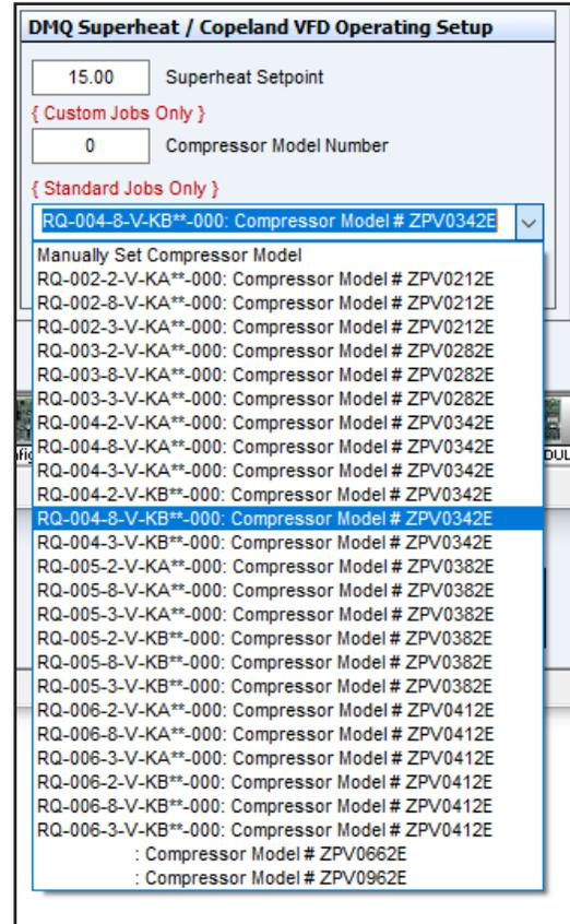
**Figure 13: Miscellaneous Setpoints Screen - Copeland™ Model Selection**
