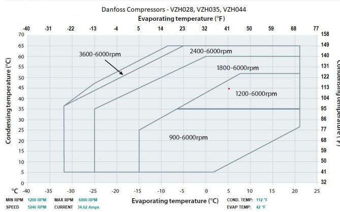
Figure 4: Danfoss VZH028, VZH035, VZH044 Envelope
