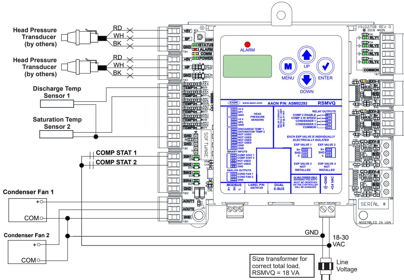
Figure 2: RSMVQ Inputs Wiring
