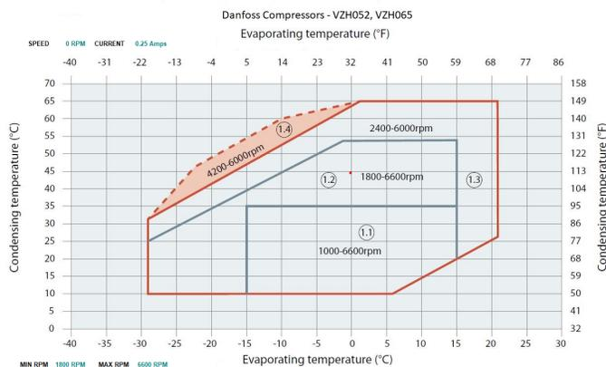
Figure 5: Danfoss VZH052 and VZH065 Envelope
