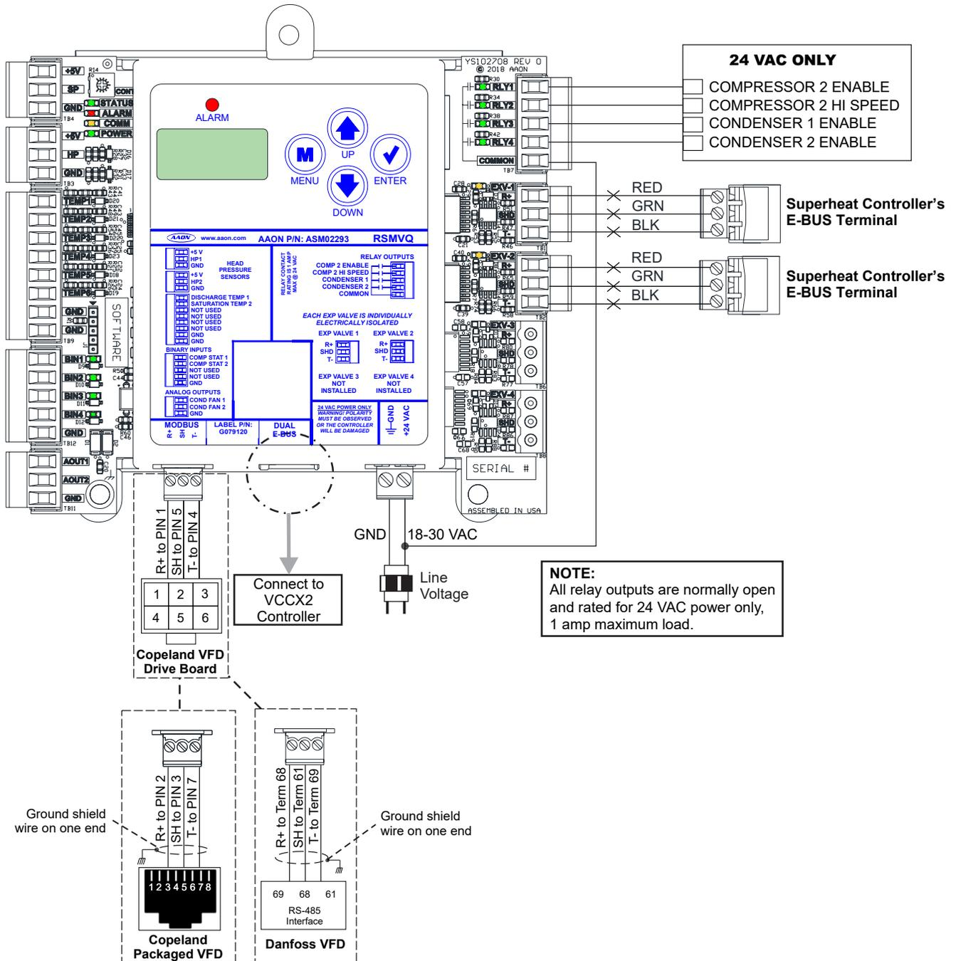
Figure 3: RSMVQ Outputs Wiring
