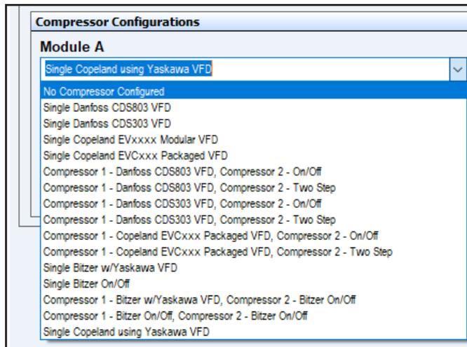
**Figure 12: RSMVQ Module A Compressor Type**
