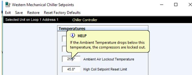
Figure 59: Prism 2 - Setpoints - Help Window
