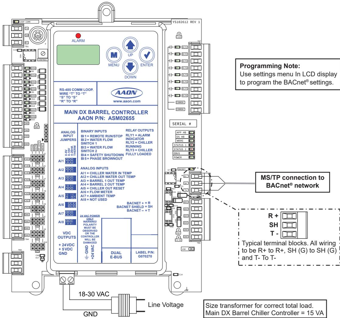
Figure 17: BACnet Connection to MS/TP Network
