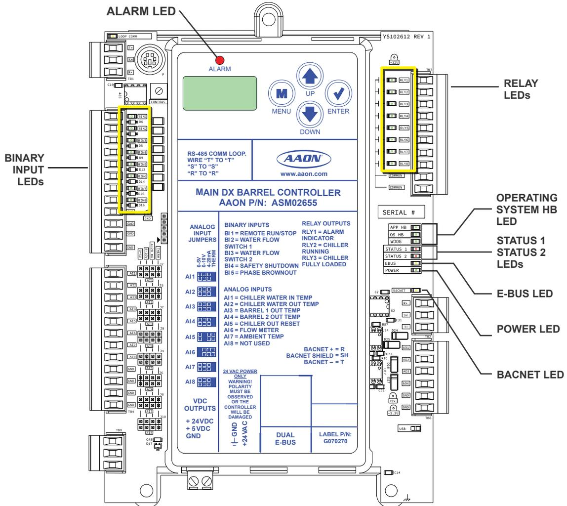
**Figure 11: Main DX Barrel Chiller Controller LED Locations**
