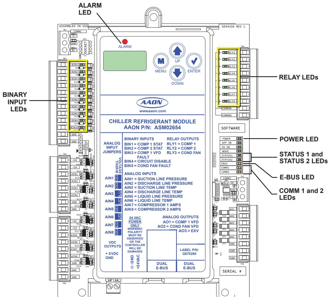
**Figure 12: Refrigerant Module LED Locations**
