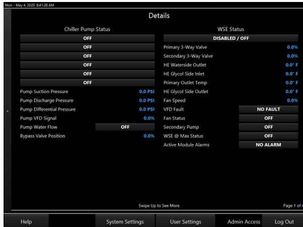
Figure 27: Chiller Pump Status and Waterside Economizer Status Details screen
