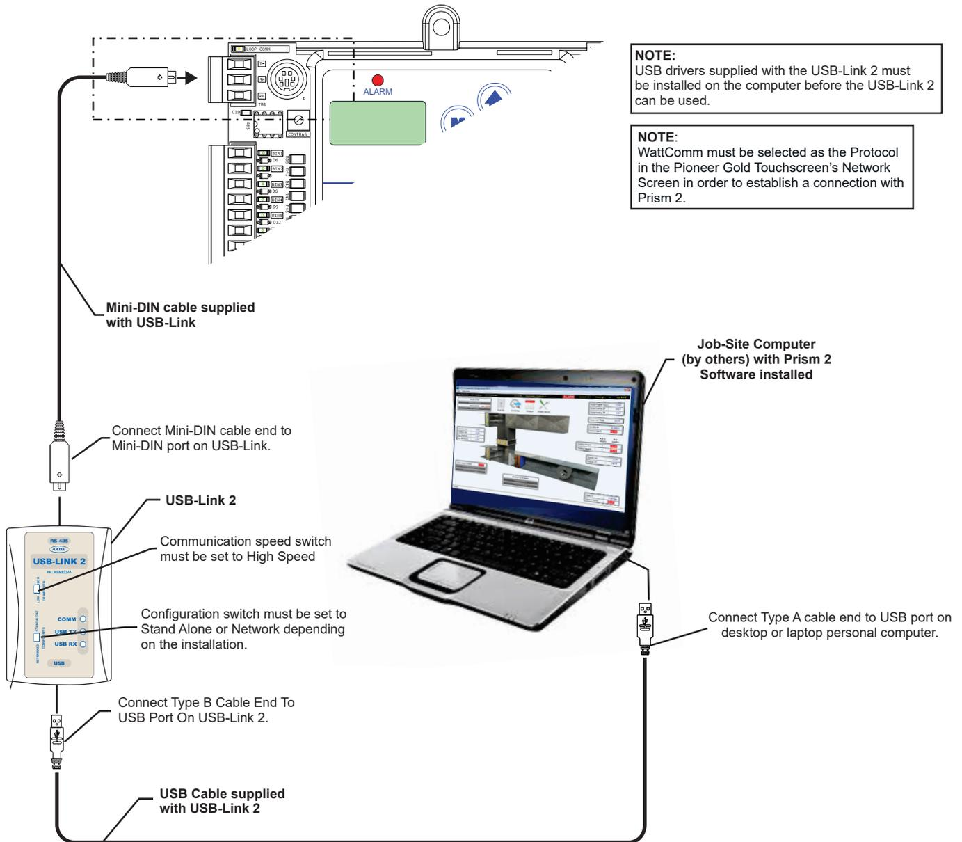
Figure 74: Prism 2 - USB-Link 2 Connection
