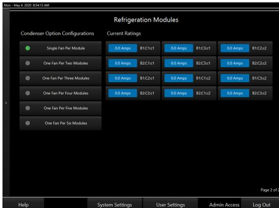
**Figure 41: Refrigeration Modules Screens**
