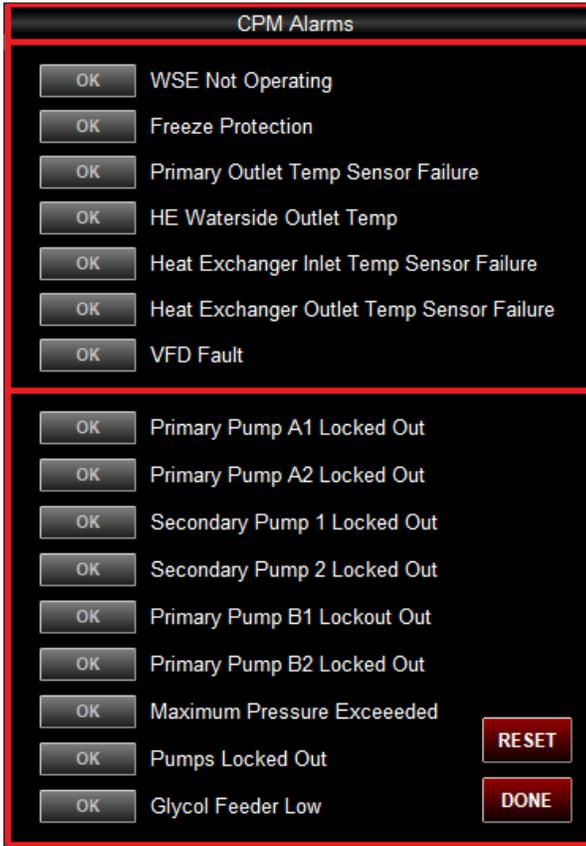
Figure 70: Prism 2 - CPM Alarms and Reset Screen
