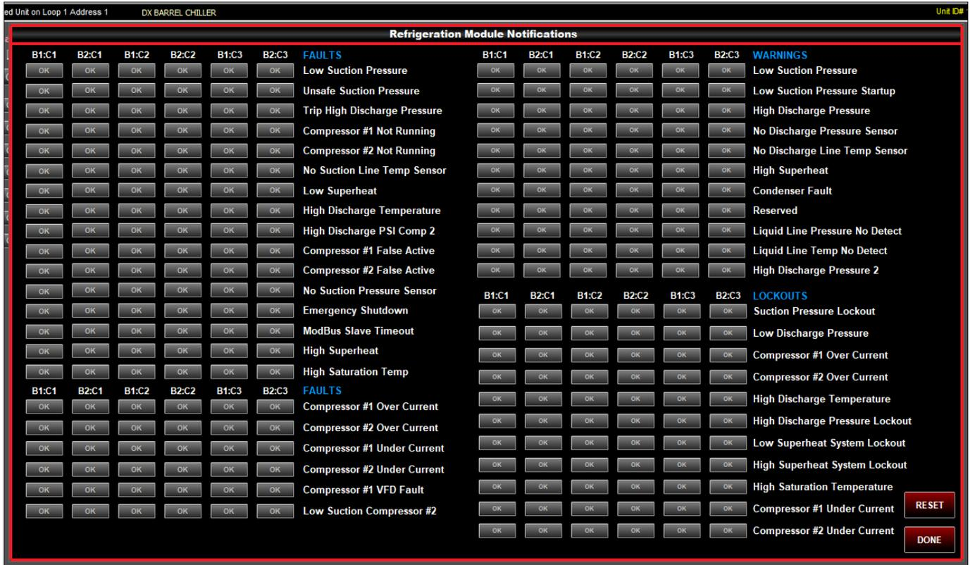
Figure 68: Prism 2 - Refrigeration Module Alarms and Reset Screen
