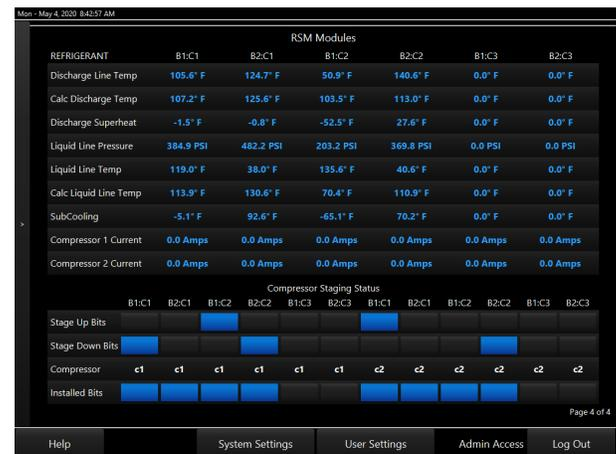
Figure 30: RSM Status and Compressor Staging Status Details Screen
