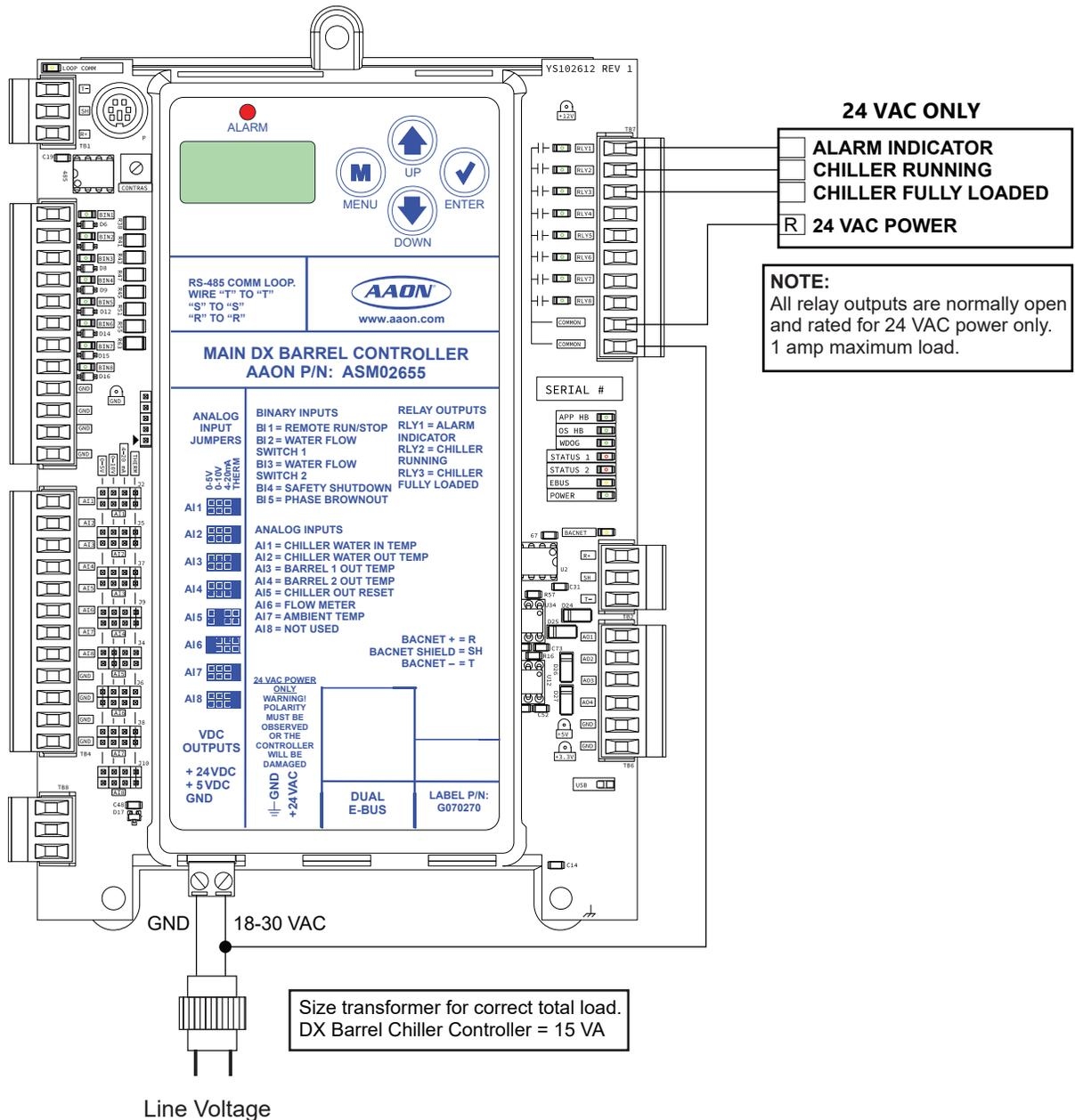
**Figure 2: Main DX Barrel Chiller Controller Output Wiring**
