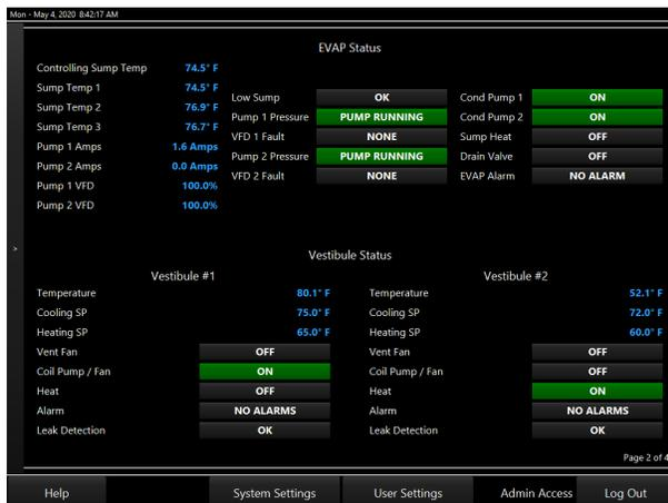
Figure 28: Evaporator Condenser Status and Vestibule Status Details Screen
