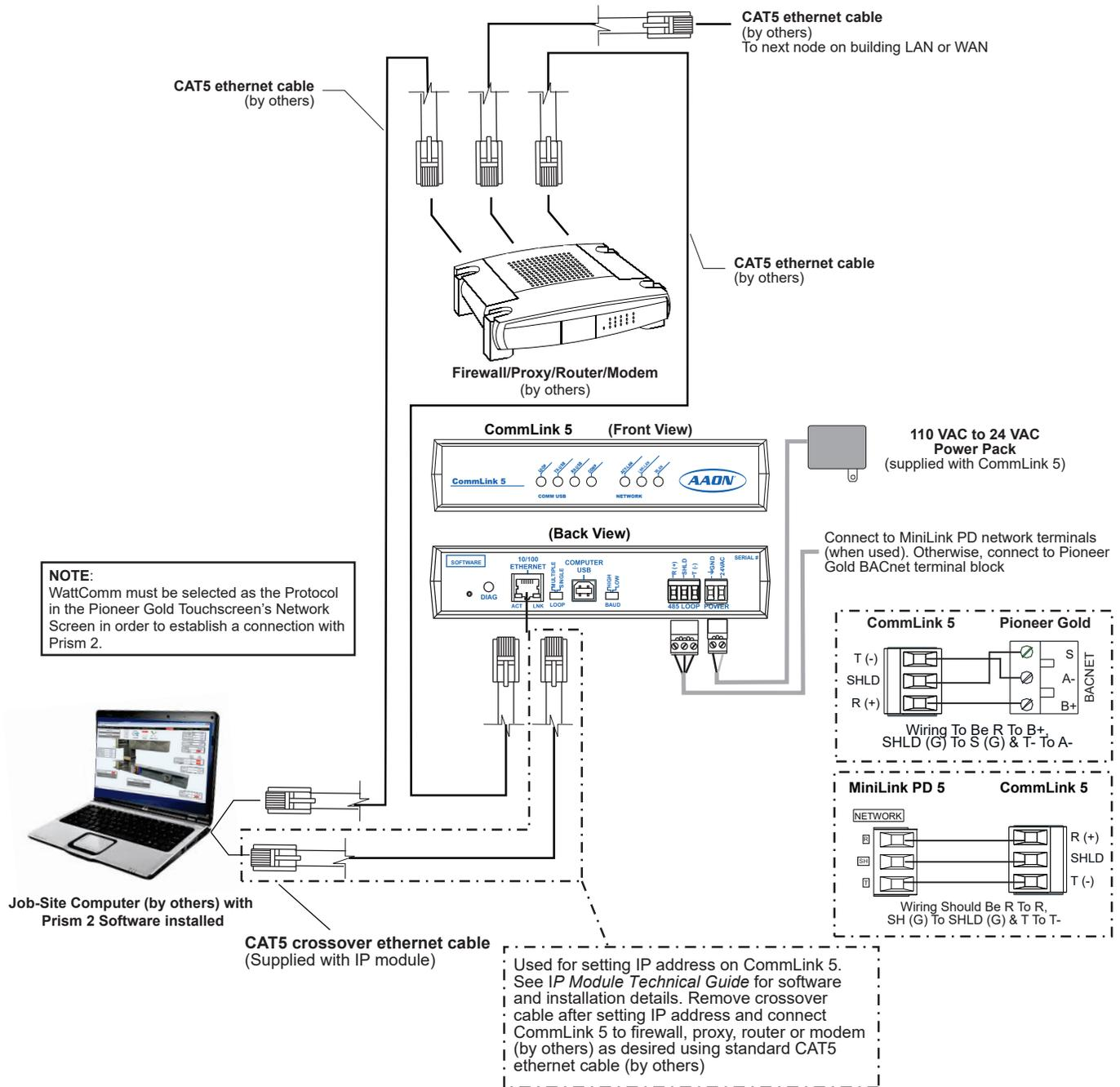
Figure 73: Prism 2 - IP Module Connection
