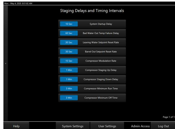
**Figure 37: Staging Delays and Timing Intervals Setpoints Screen**
