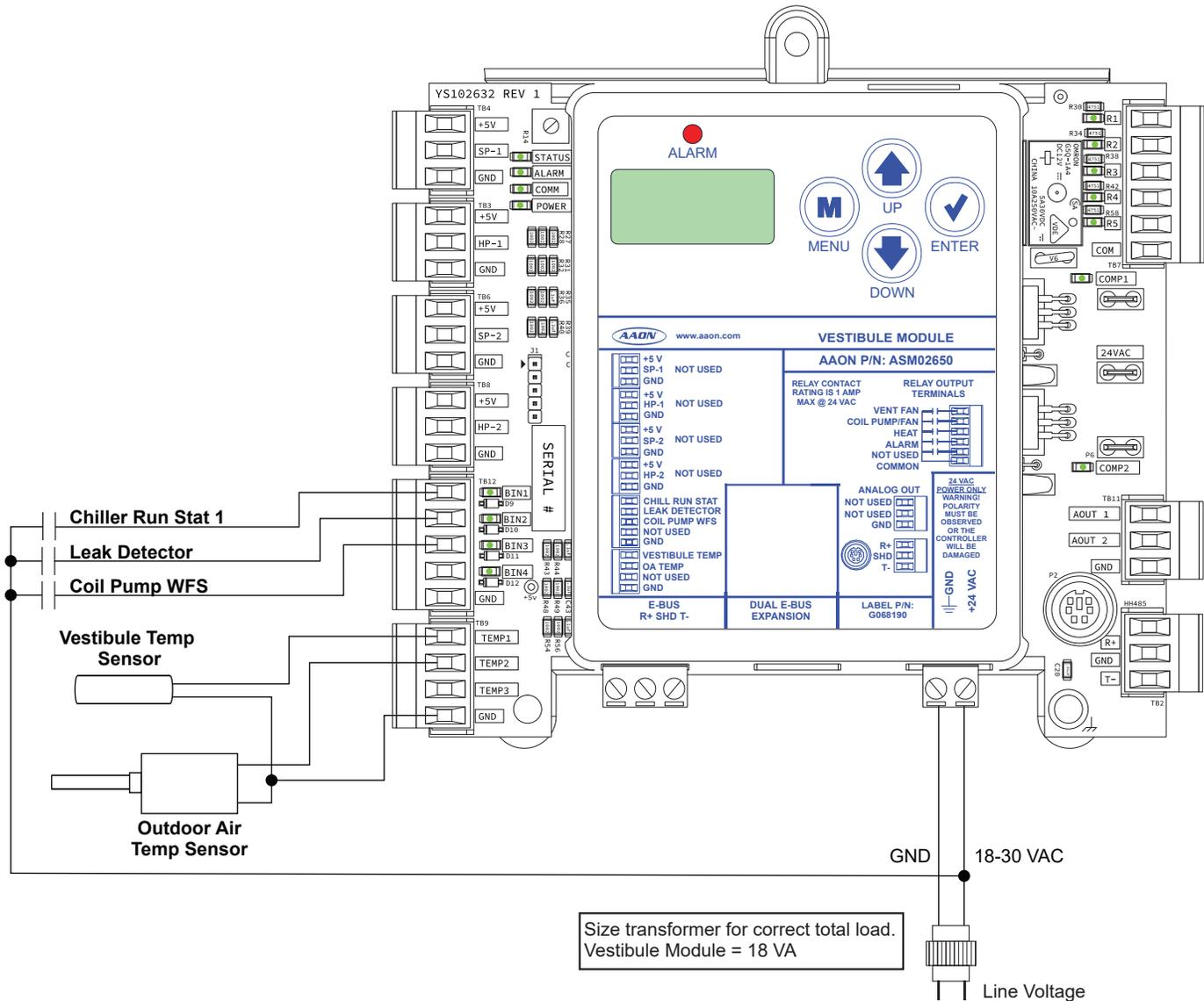
**Figure 9: Vestibule Module Input Wiring**
