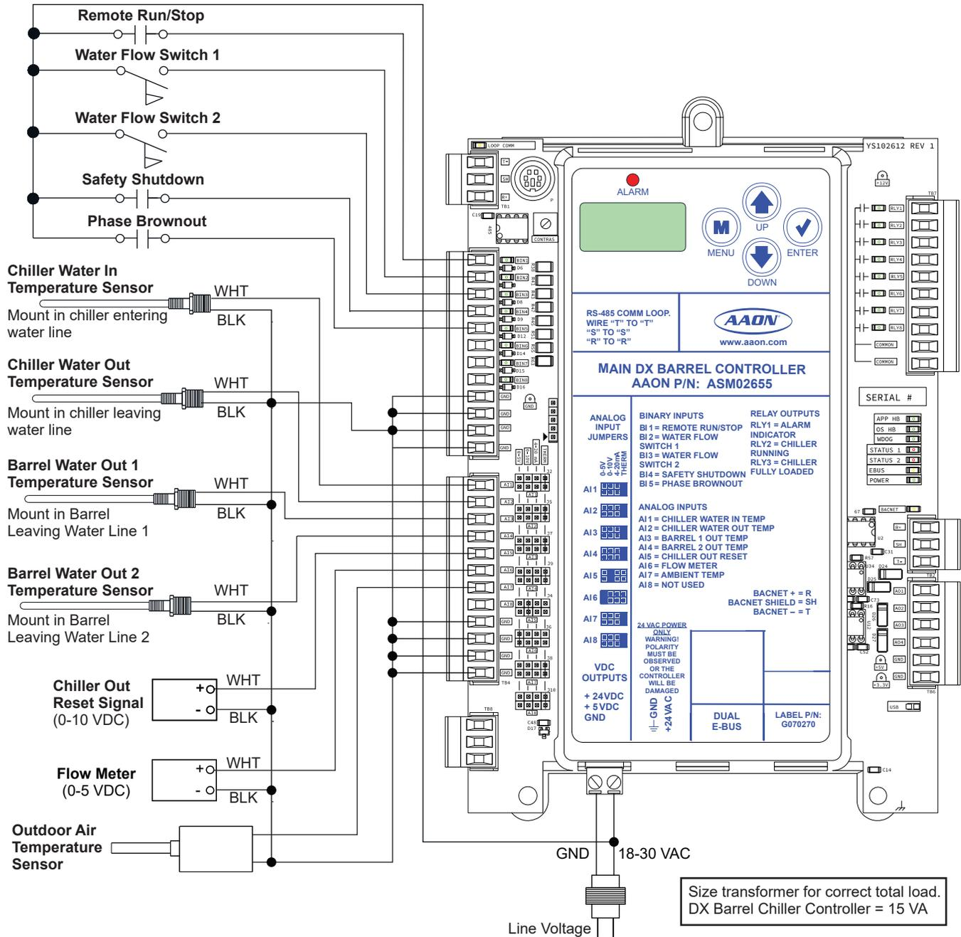
Figure 1: Main DX Barrel Chiller Controller Input Wiring
