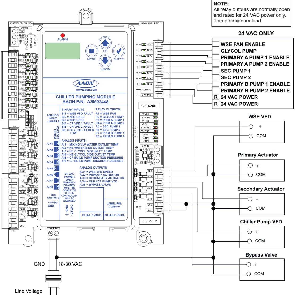
Figure 6: Chiller Pumping Module Output Wiring
