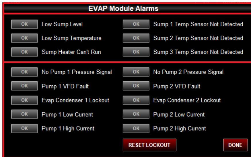
Figure 69: Prism 2 - EVAP Module Alarms and Reset Screen
