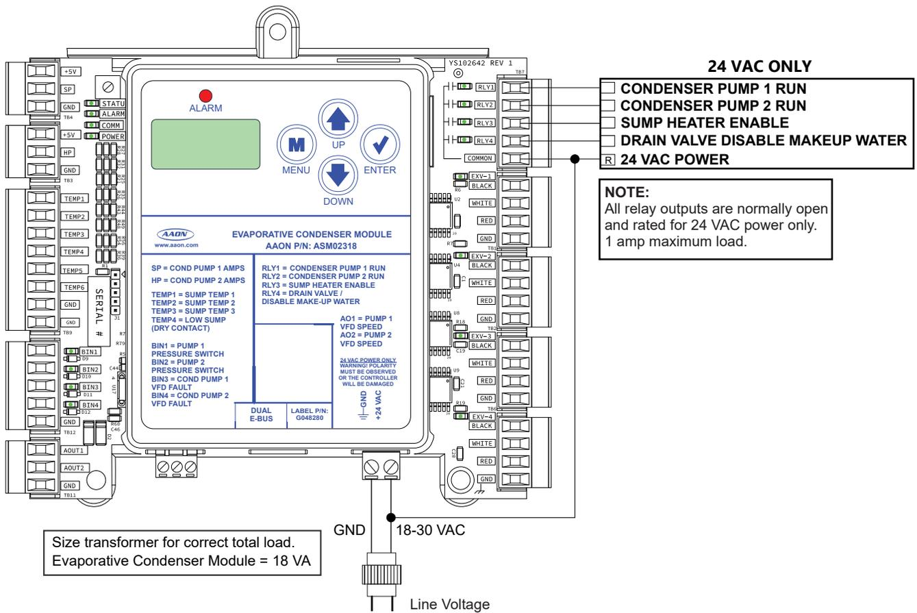
Figure 8: Evaporative Condenser Module Output Wiring
