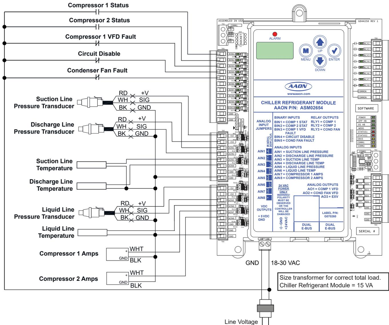
Figure 3: Chiller Refrigerant Module Input Wiring
