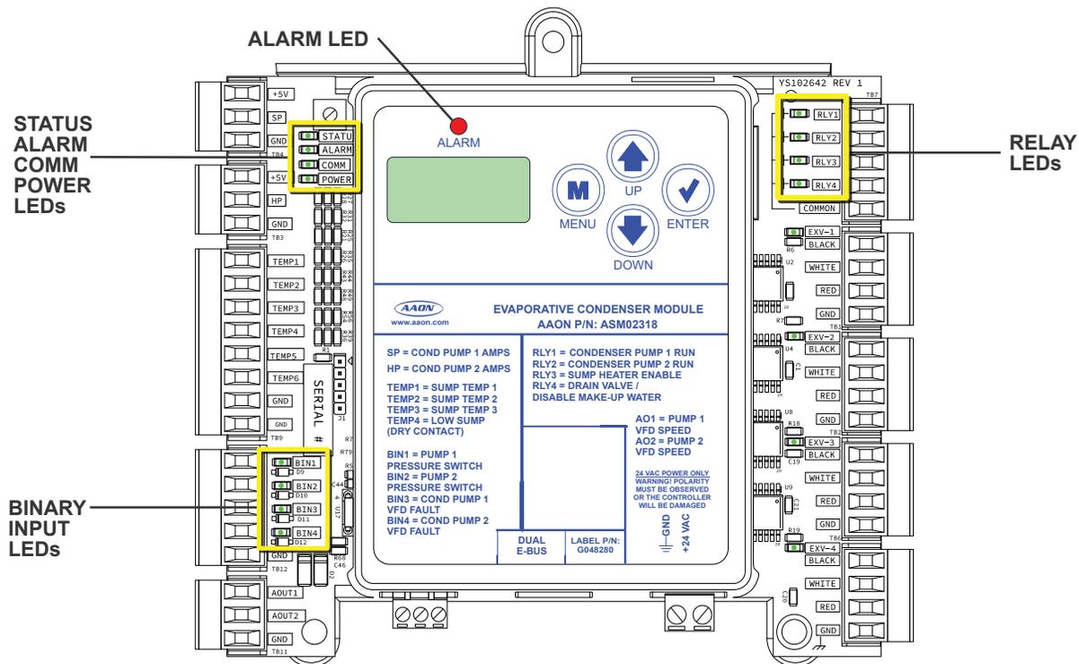
Figure 14: Evaporative Condenser Module LEDs
