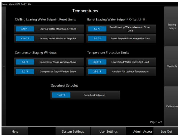
**Figure 36: Temperatures Setpoints Screen**
