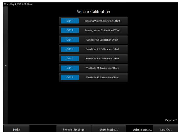
**Figure 39: Sensor Calibration Setpoints Screen**
