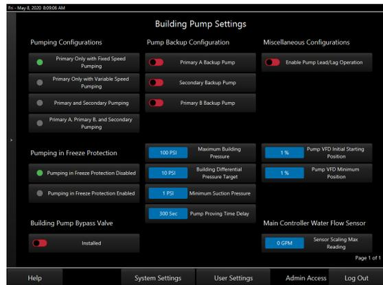
**Figure 43: Boiler Pump Settings Screen**
