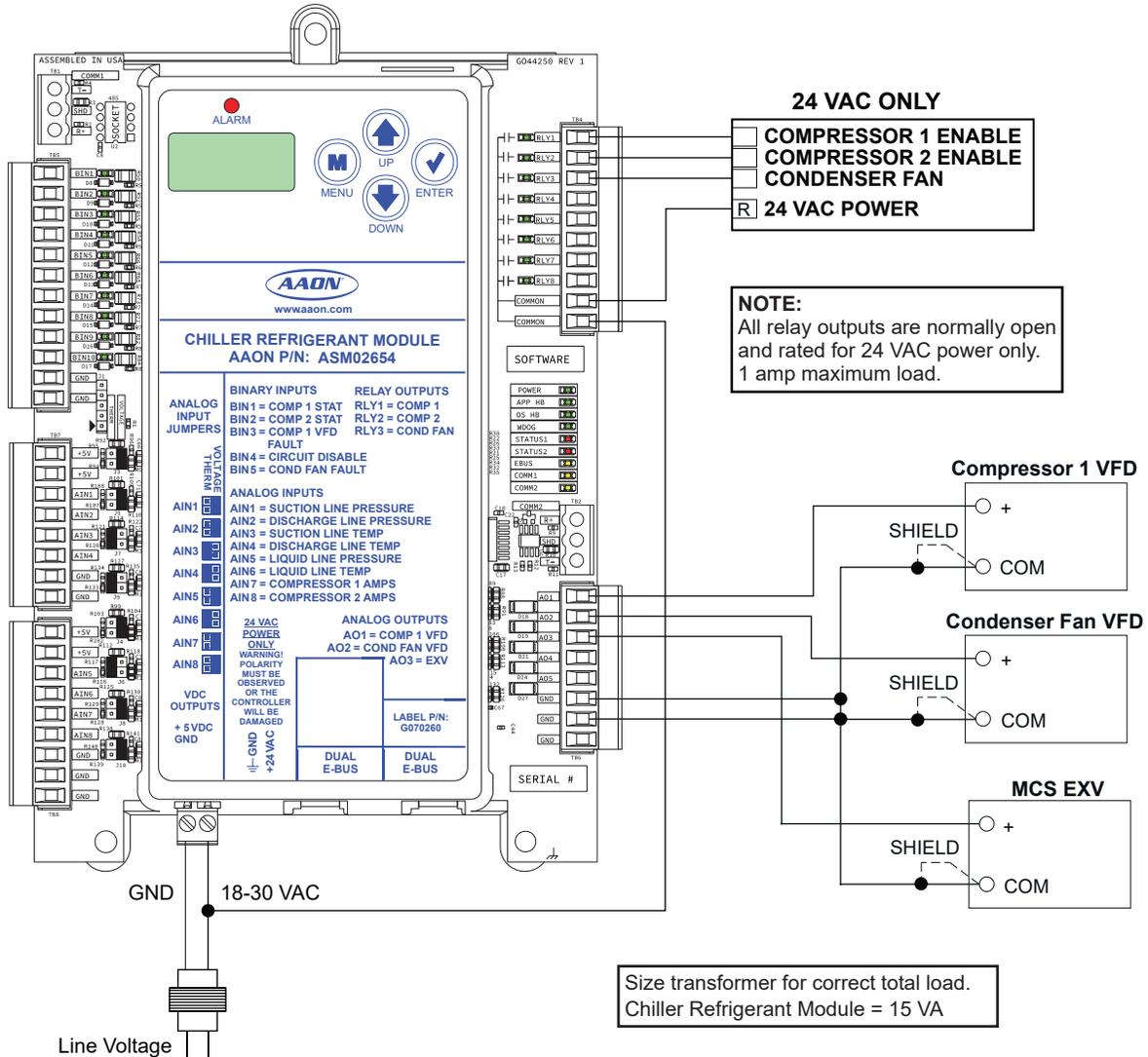
**Figure 4: Chiller Refrigerant Module Output Wiring**
