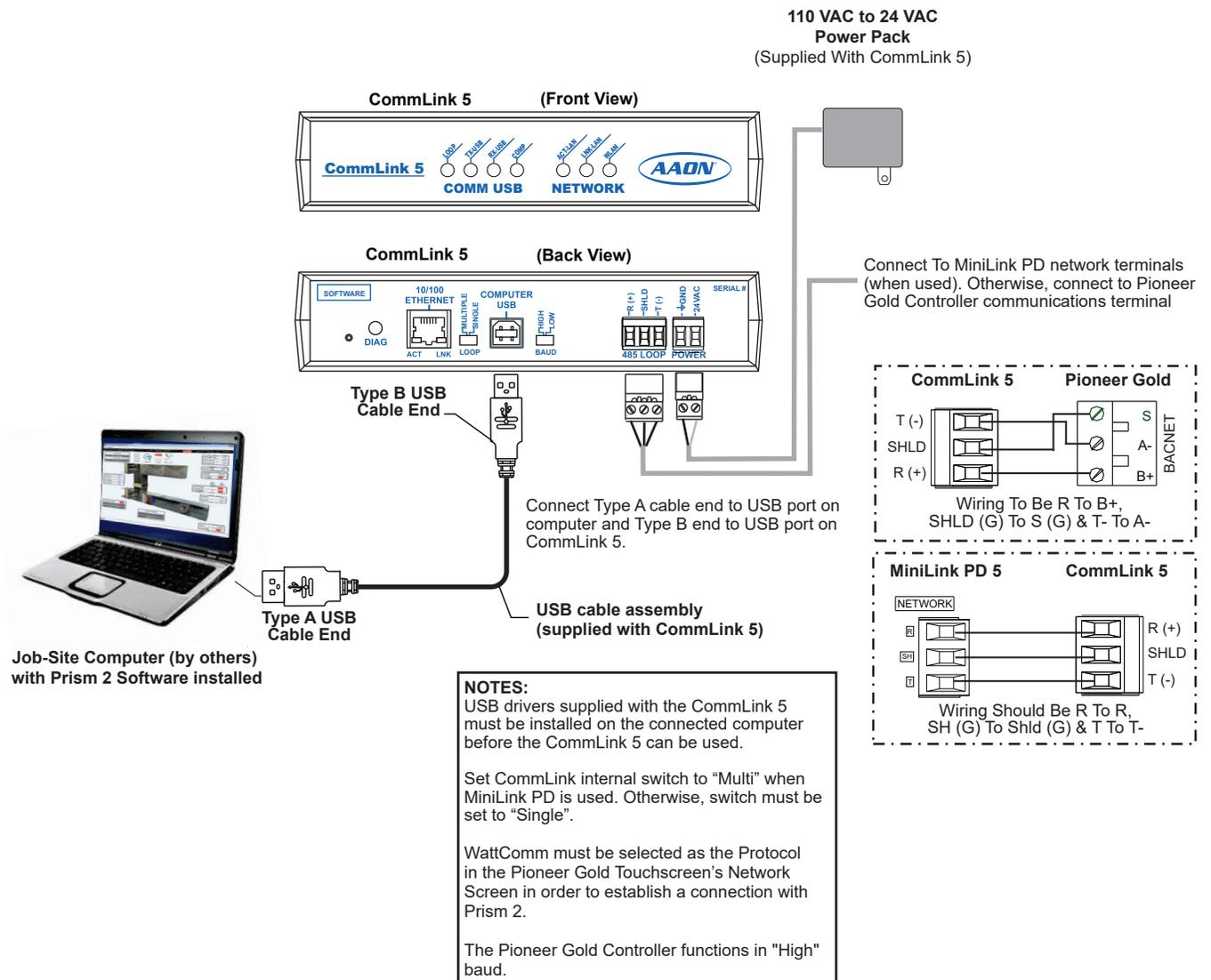
Figure 72: Prism 2 - CommLink 5 Connection
