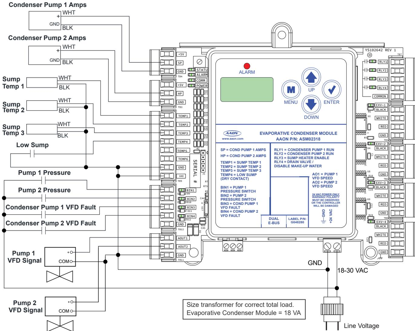
Figure 7: Evaporative Condenser Module Input Wiring
