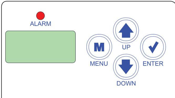
**Figure 16: LCD Display Screen and Navigation Keys**
