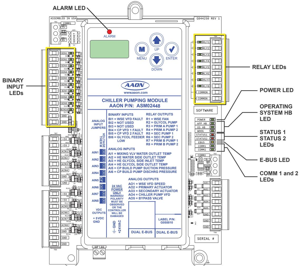
**Figure 13: Chiller Pumping Module LED Locations**
