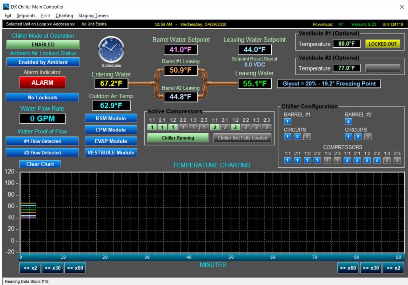
**Figure 48: Prism 2 - DX Chiller Main Controller Status Screen**
