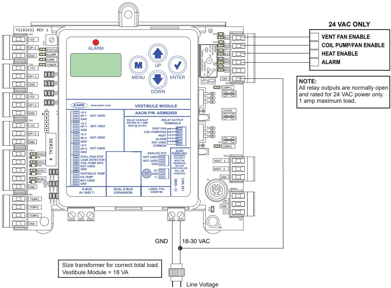
**Figure 10: Vestibule Module Output Wiring**
