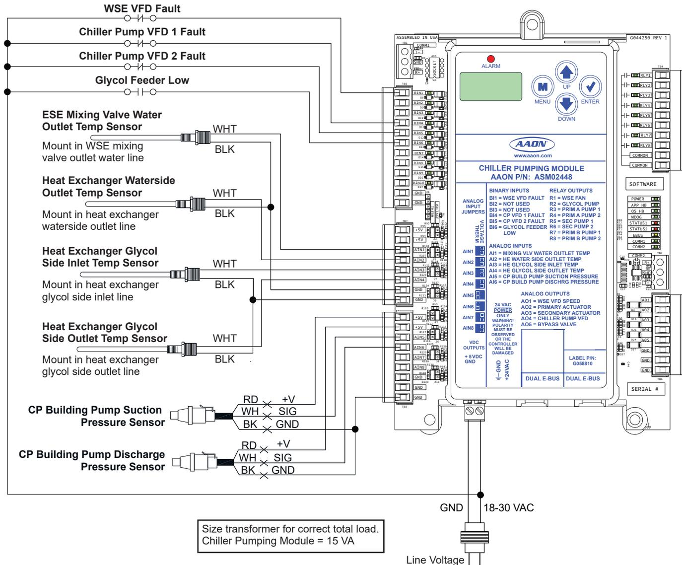
**Figure 5: Chiller Pumping Module Input Wiring**
