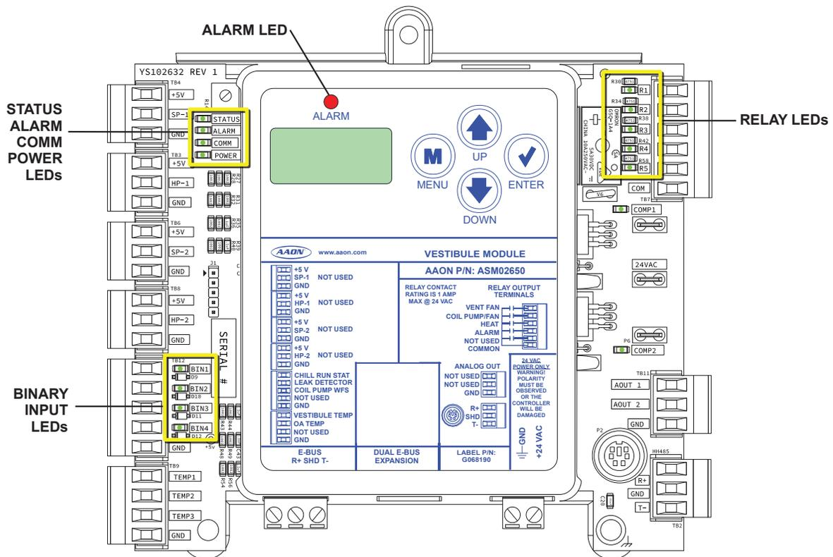
Figure 15: Vestibule Module LEDs
