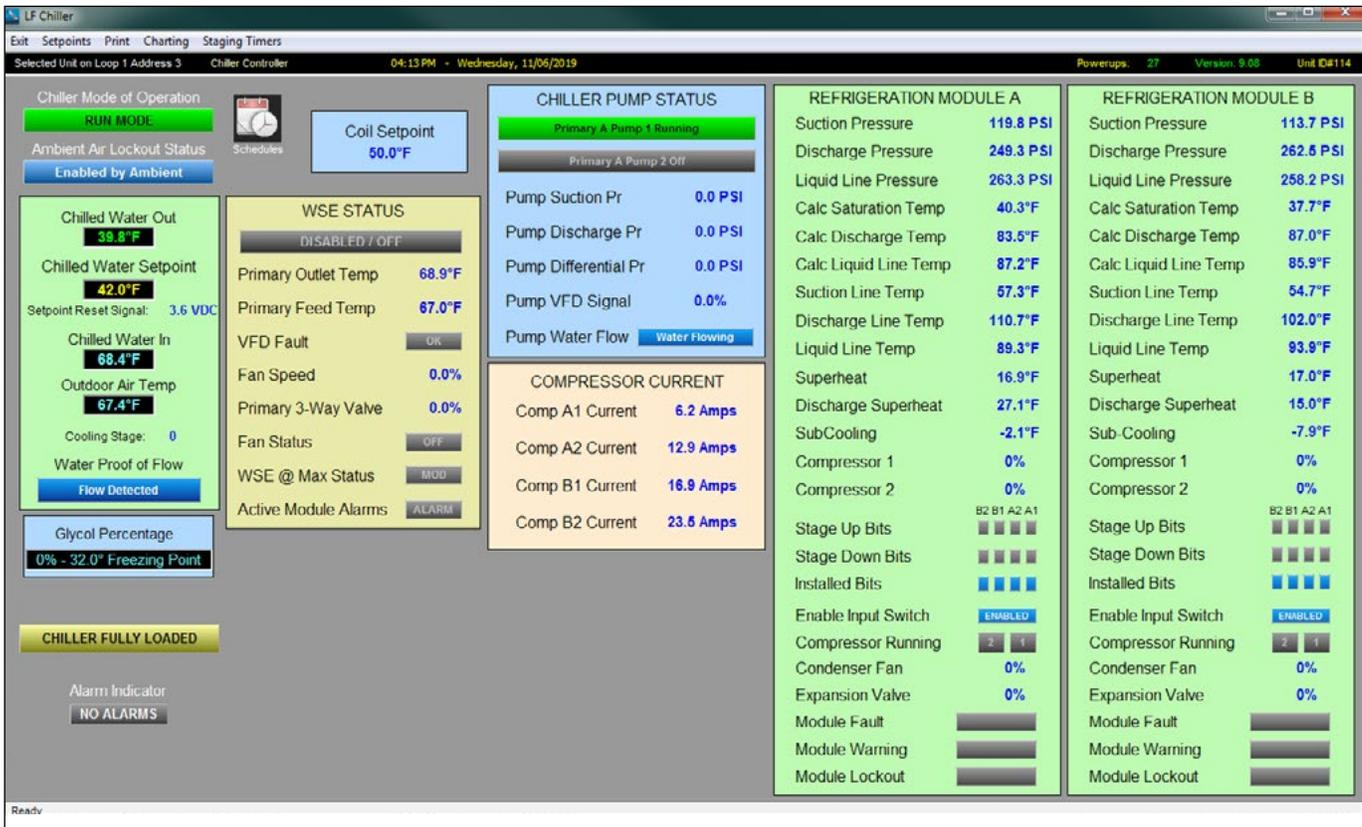
Figure 14: LF Chiller Controller Status Screen
