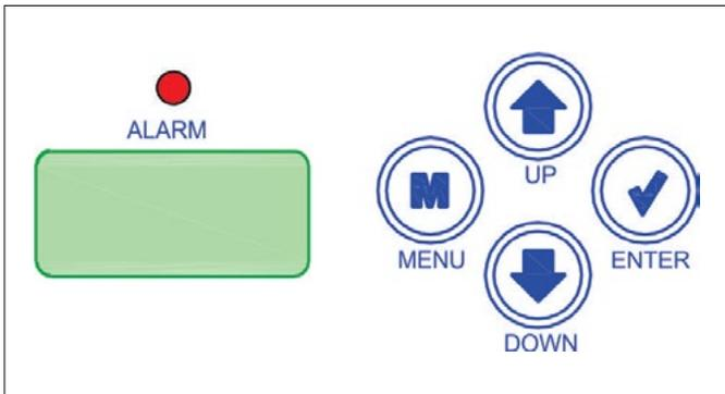
**Figure 12: LCD Display and Navigation/Editing Keys**
