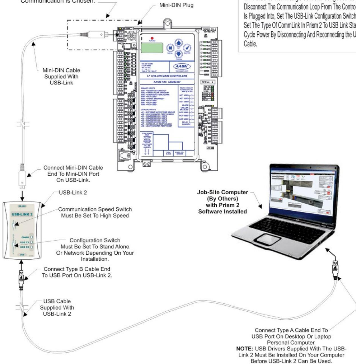
Figure 32: USB-Link 2 Connection
