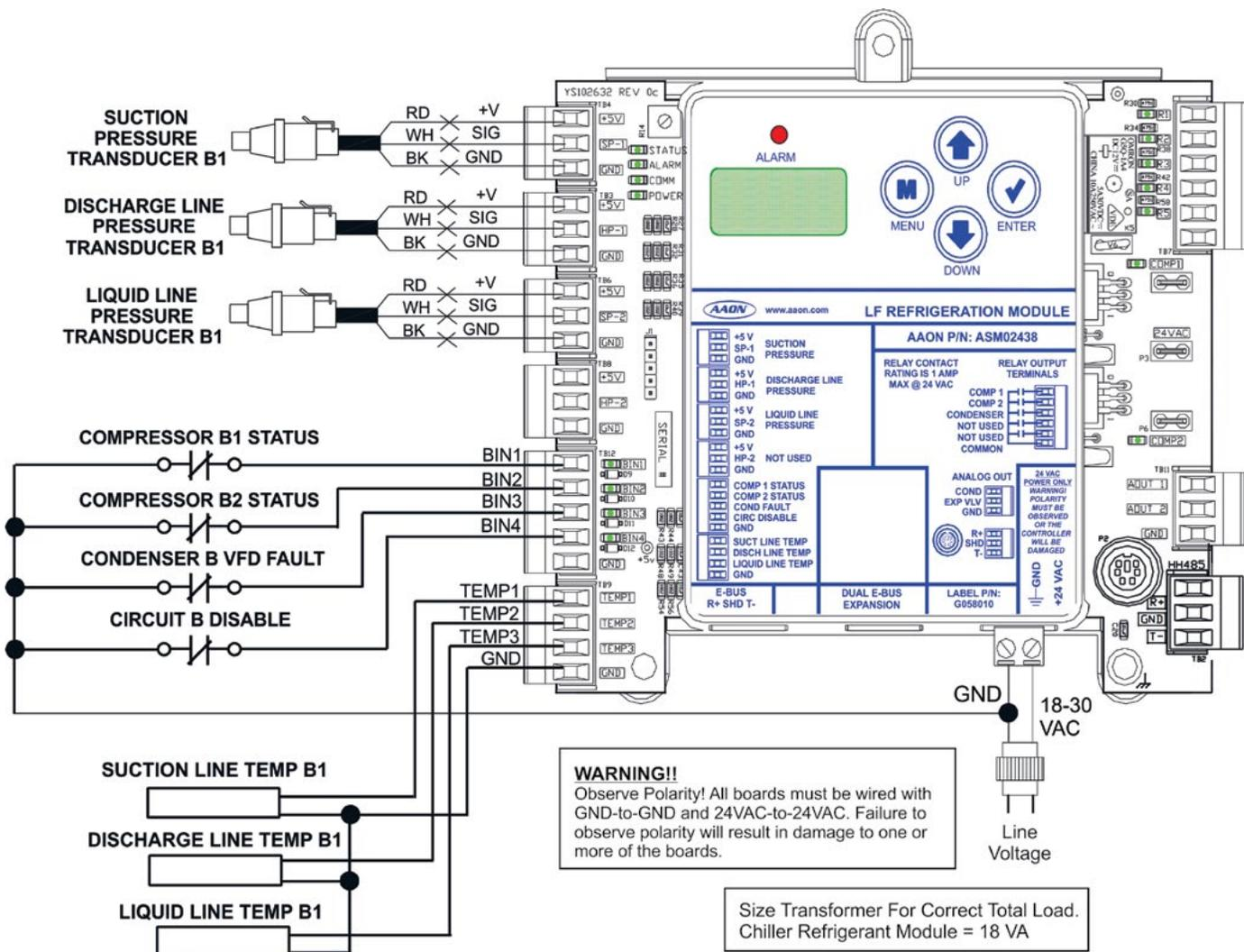
Figure 5: Chiller Refrigerant B Module Input Wiring
