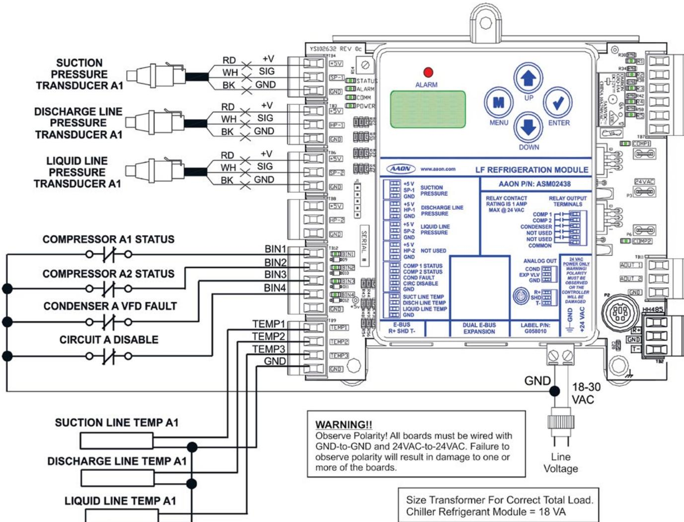
Figure 3: Chiller Refrigerant A Module Input Wiring
