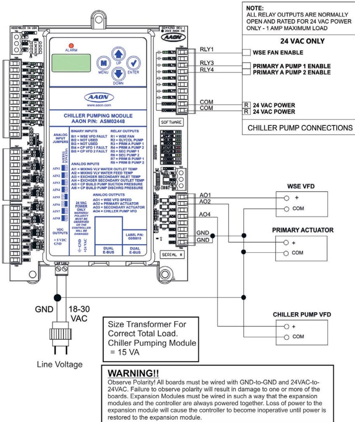
Figure 8: Chiller Pumping Module Output Wiring
