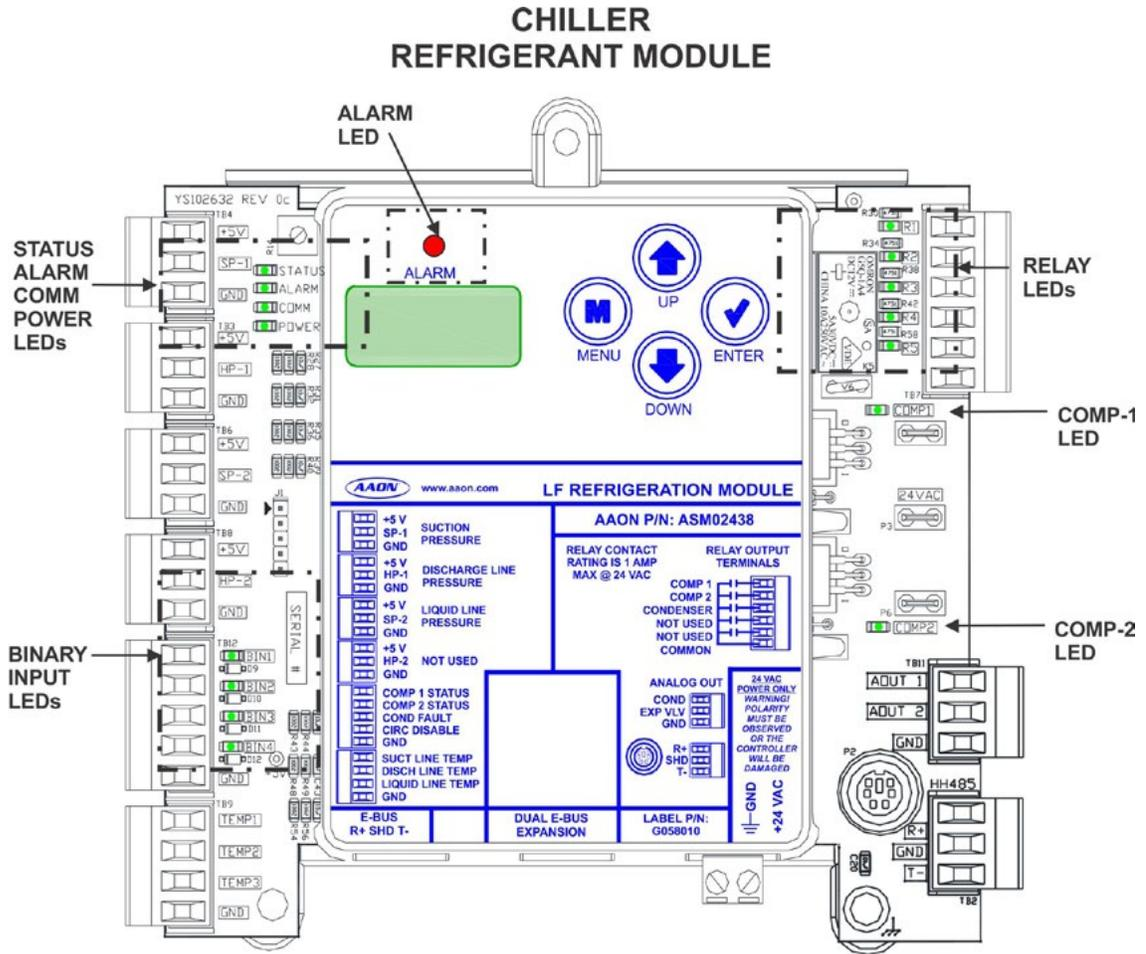
Figure 10: Refrigerant Module A & B LED Locations
