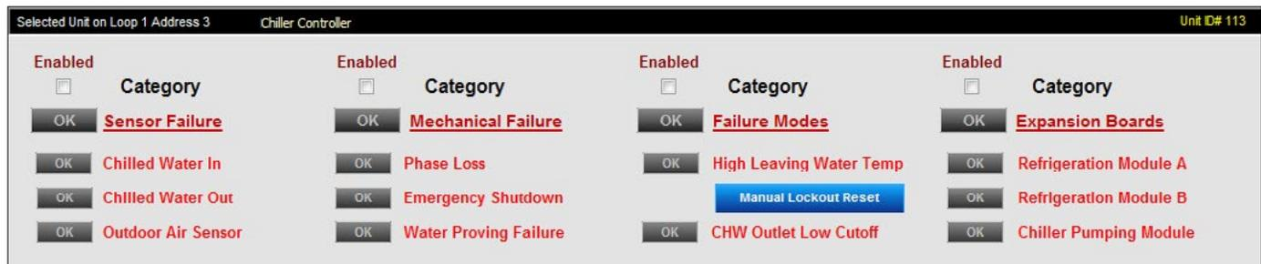
**Figure 29: Unit Alarm Status Screen**
