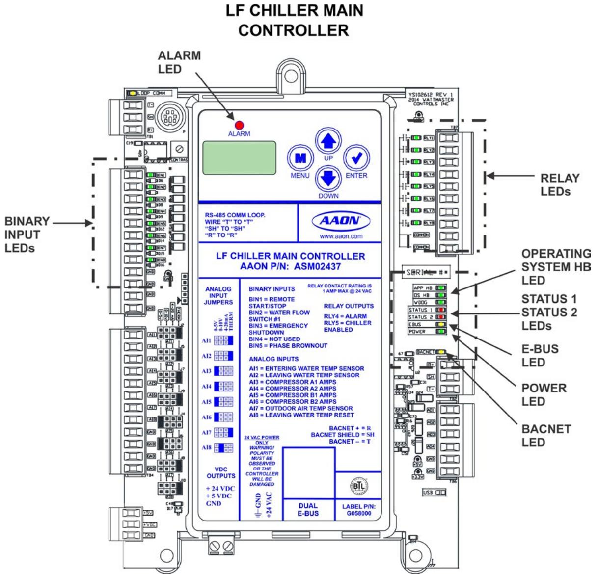
Figure 9: LF Chiller Main Controller LED Locations
