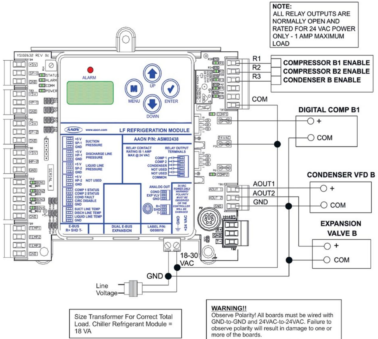
Figure 6: Chiller Refrigerant B Module Output Wiring
