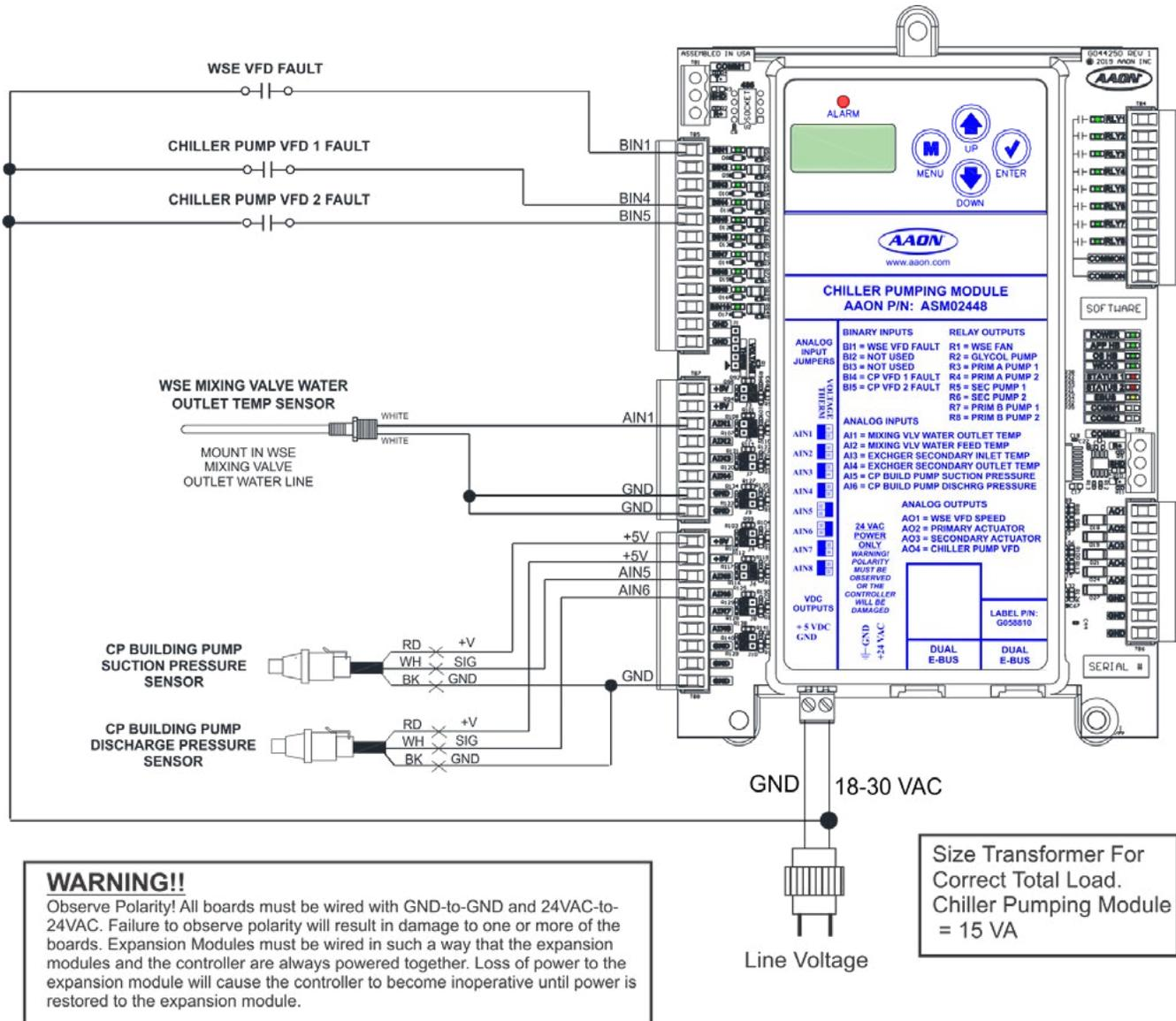
Figure 7: Chiller Pumping Module Input Wiring
