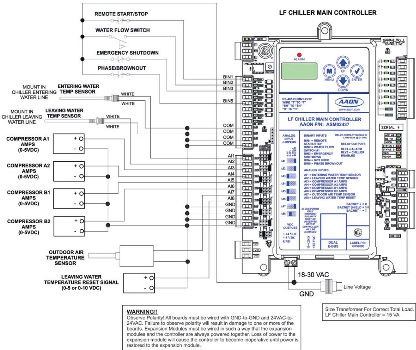
Figure 1: LF Chiller Main Controller Input Wiring
