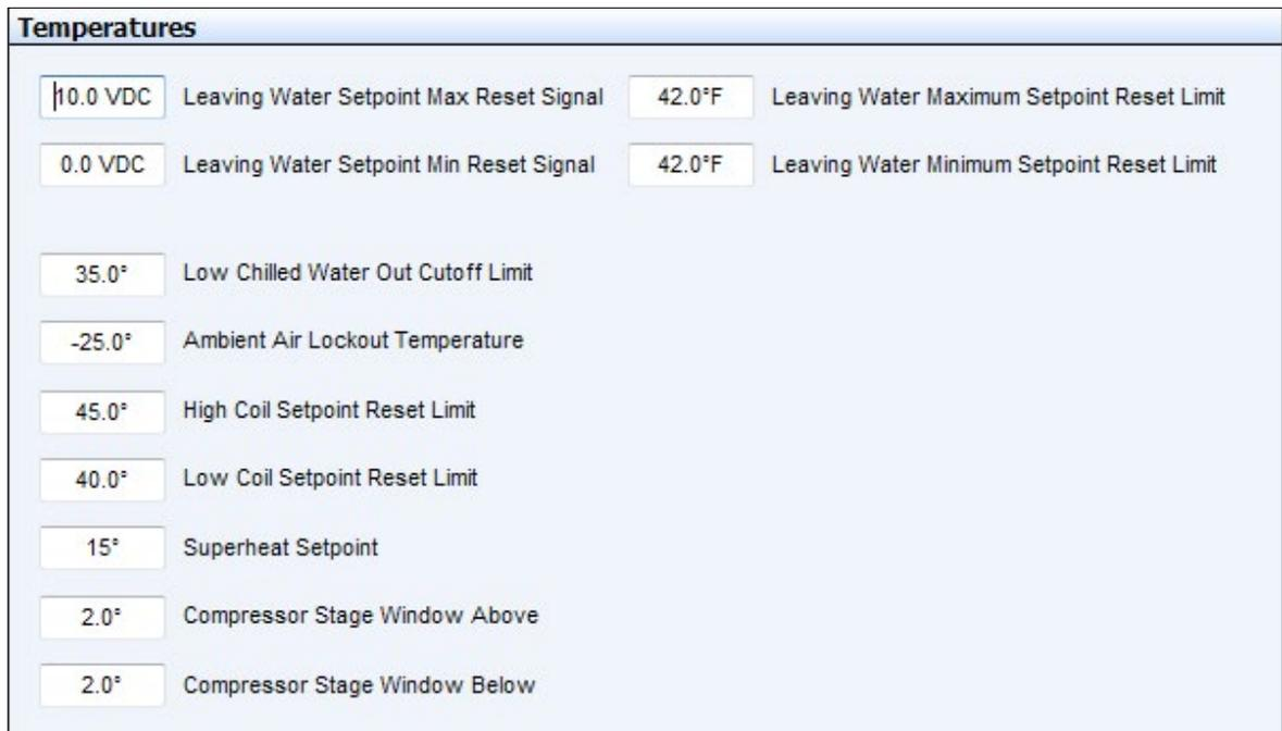
**Figure 15: Temperatures Setpoints Screen**
