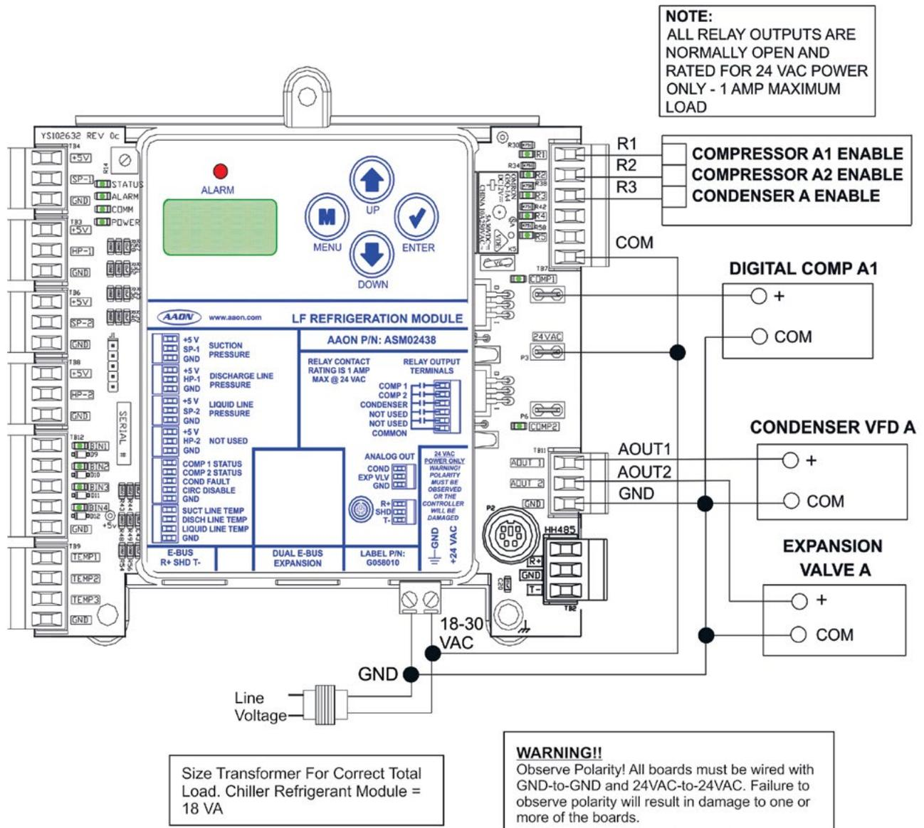
Figure 4: Chiller Refrigerant A Module Output Wiring
