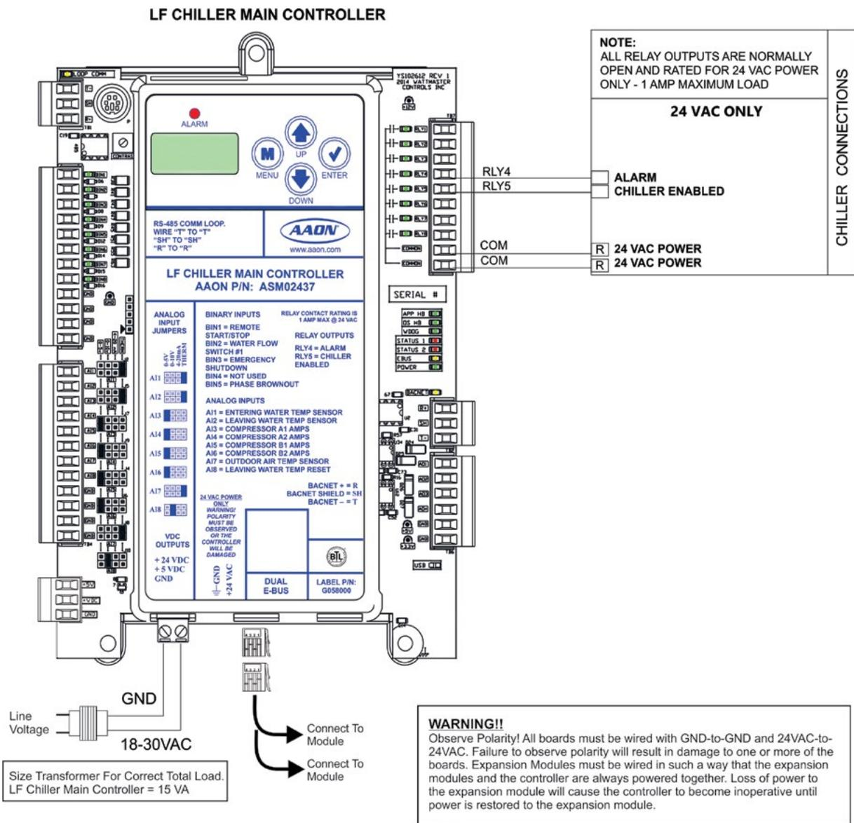
Figure 2: LF Chiller Main Controller Output Wiring
