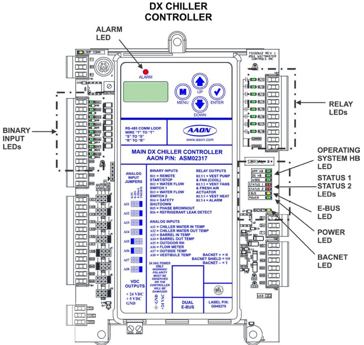
Figure 13: DX Chiller Controller LED Locations
