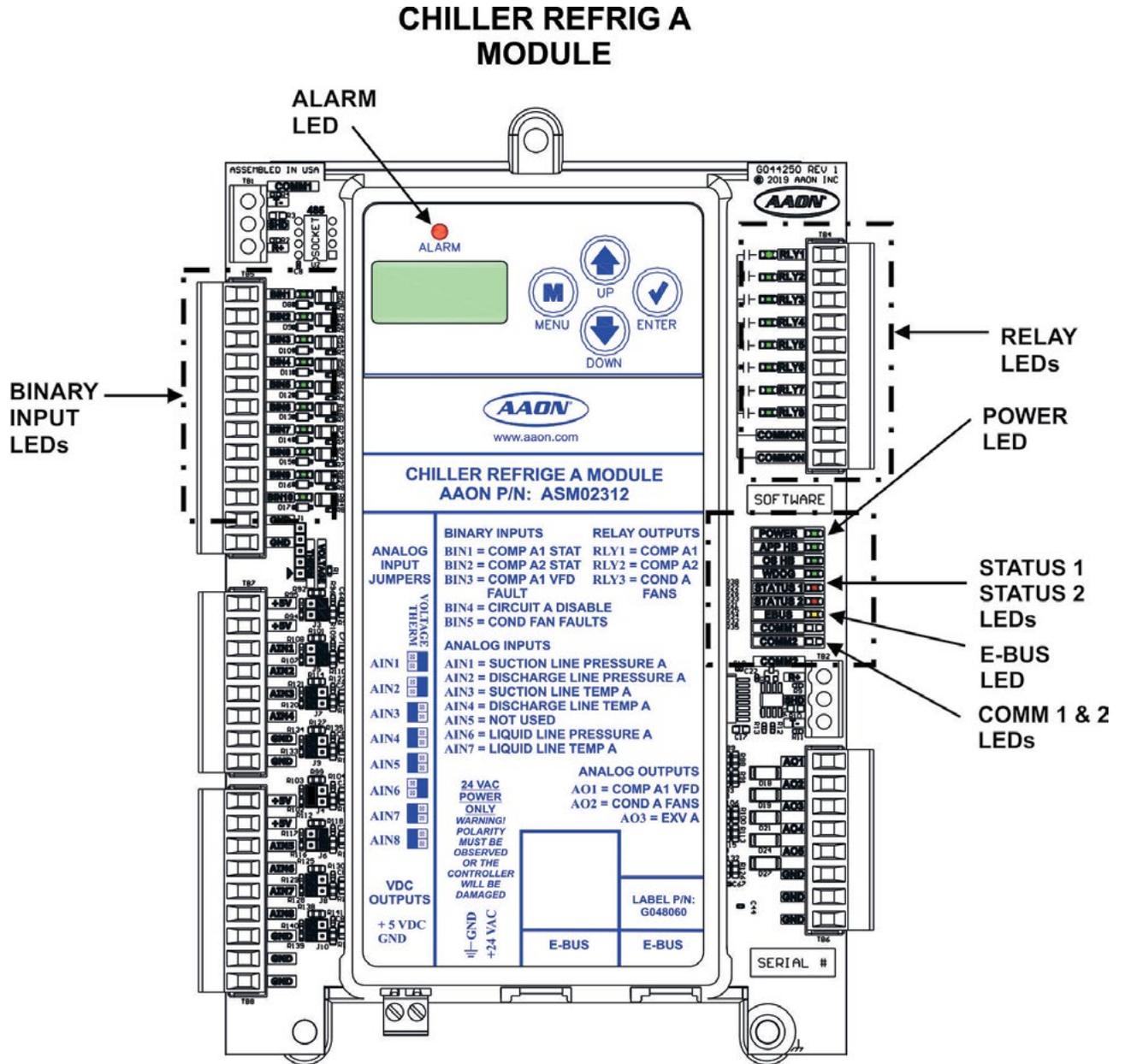
Figure 14: Refrigerant A & B Module LED Locations (Refrig A Module Shown)
