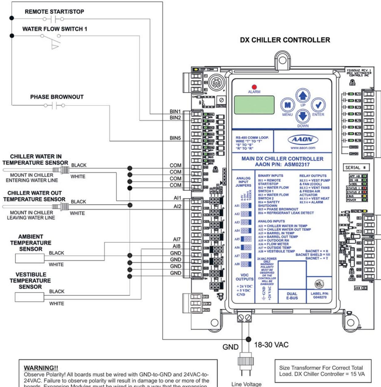
Figure 1: Main DX Chiller Controller Input Wiring
