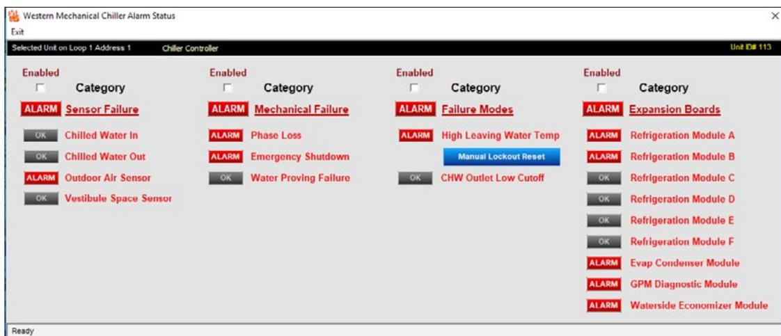
Figure 32: Unit Alarm Status Screen
