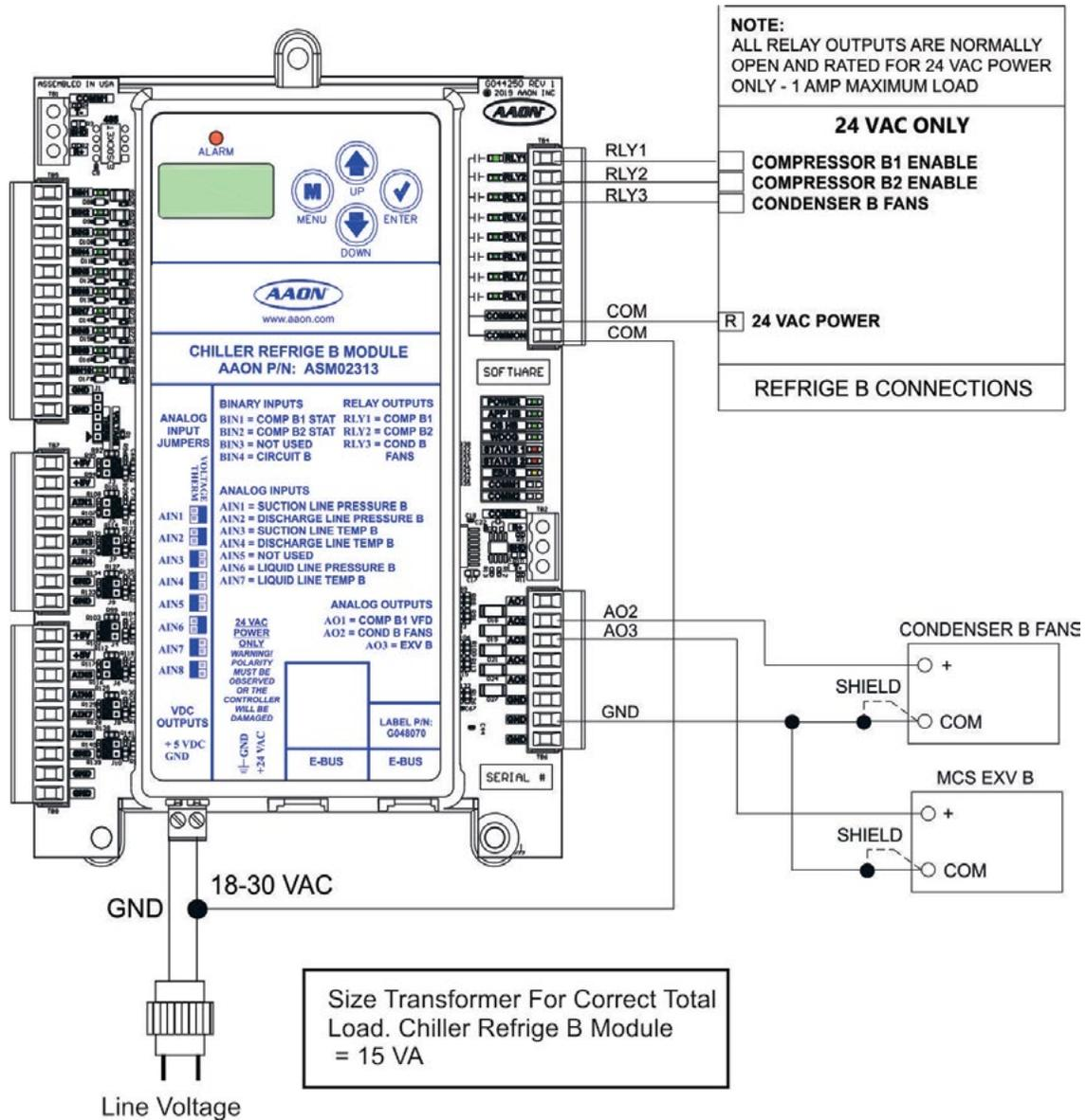
Figure 6: Chiller Refrigeration B Module Output Wiring
