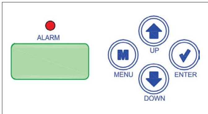
**Figure 17: LCD Display and Navigation/Editing Keys**
