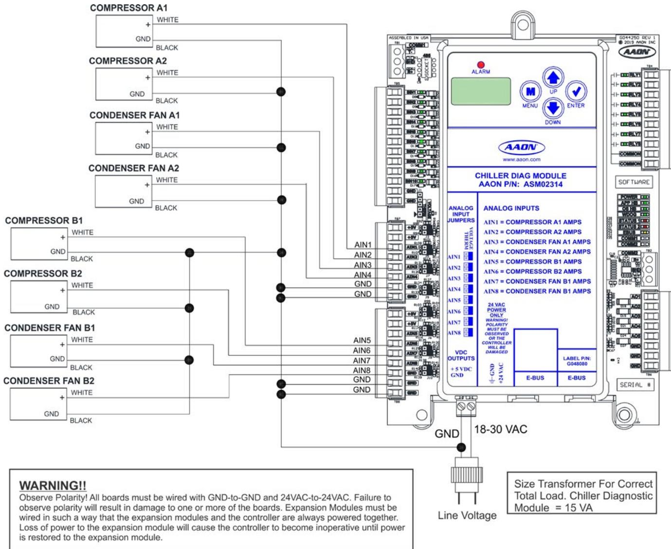
Figure 11: Chiller Diagnostic Module Wiring
