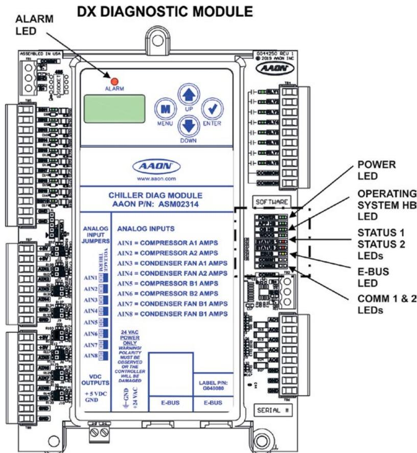
Figure 12: DX Chiller Diagnostics Module LED Locations
