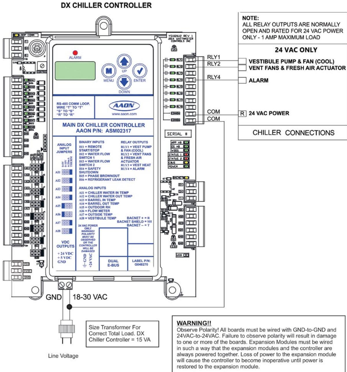
Figure 2: Main DX Chiller Controller Output Wiring
