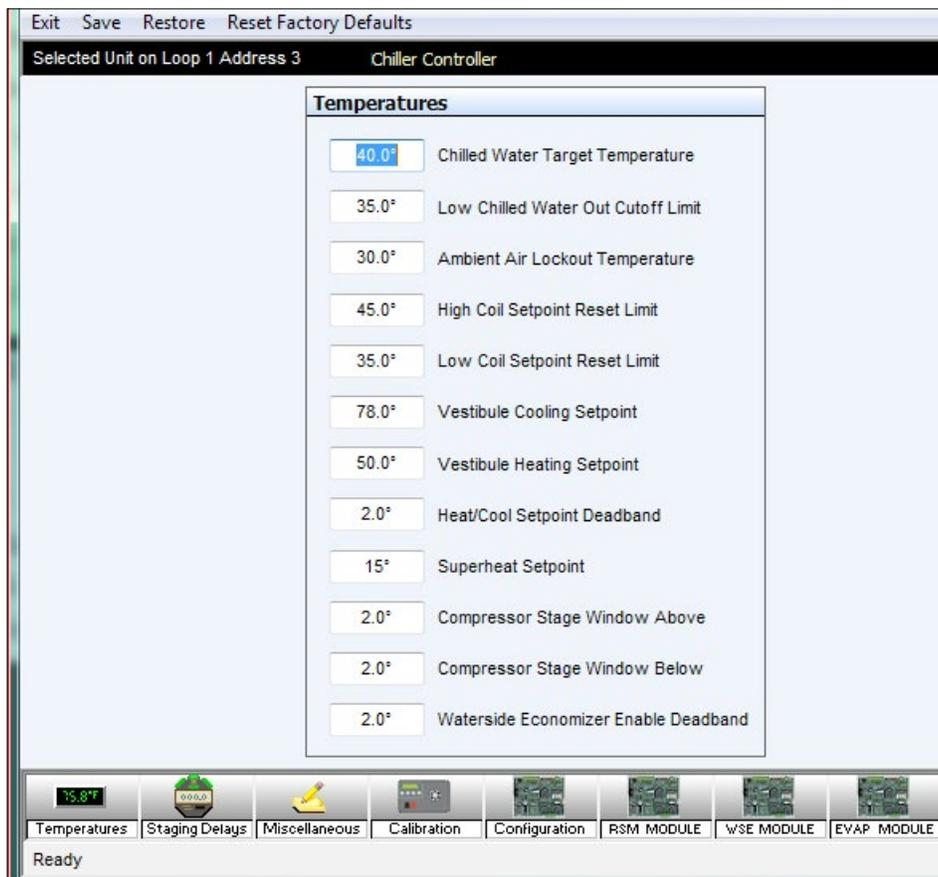
Figure 20: Temperatures Setpoints Screen
