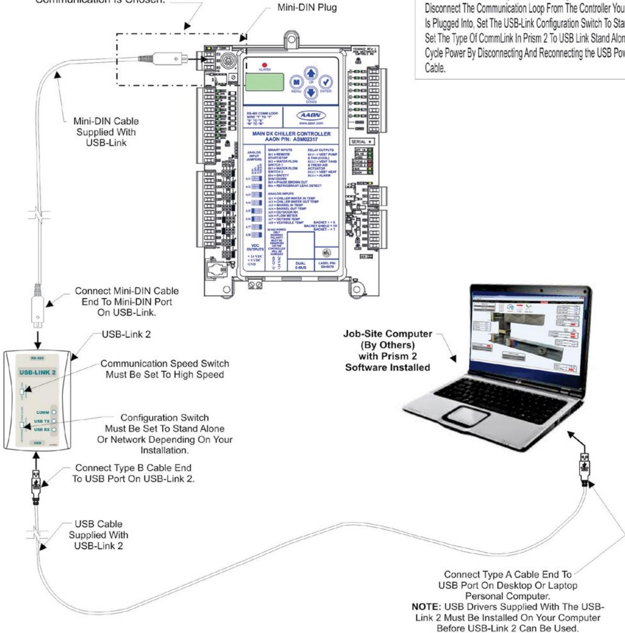
Figure 35: USB-Link 2 Connection
