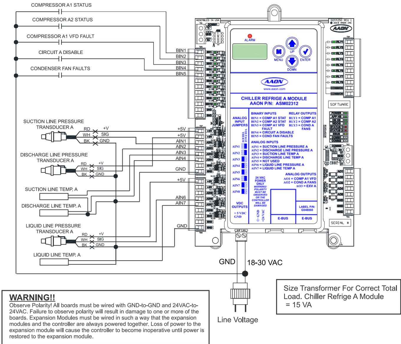
Figure 3: Chiller Refrigeration A Module Input Wiring
