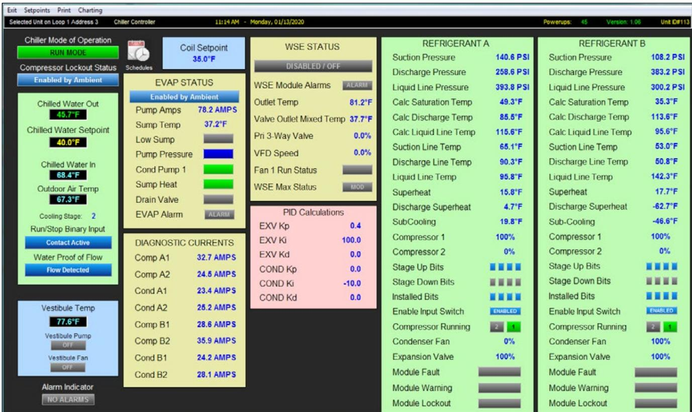
Figure 19: DX Chiller Controller Status Screen
