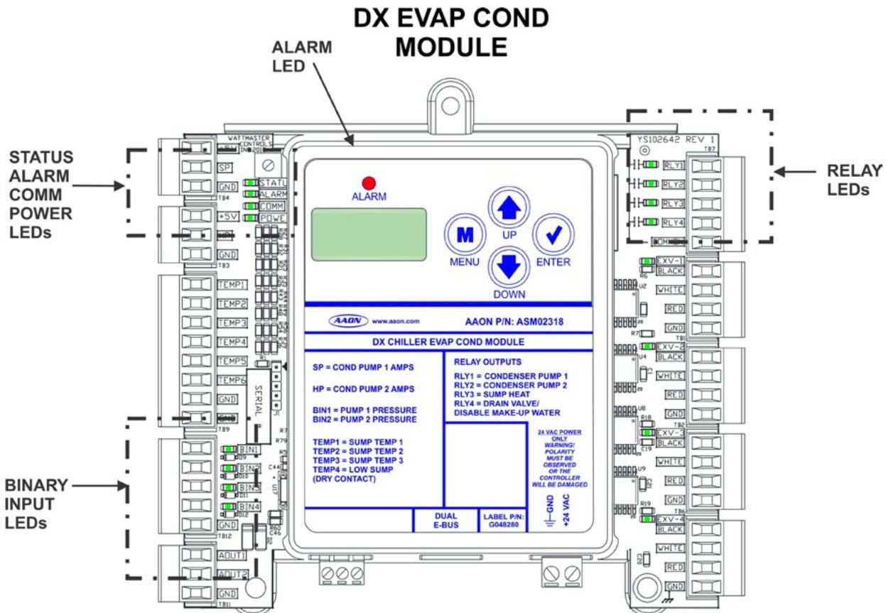
Figure 16: DX Evaporative Condenser Module LEDs
