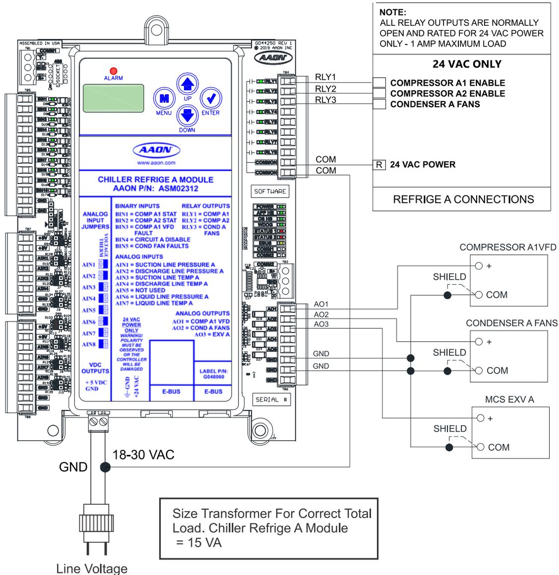
Figure 4: Chiller Refrigeration A Module Output Wiring
