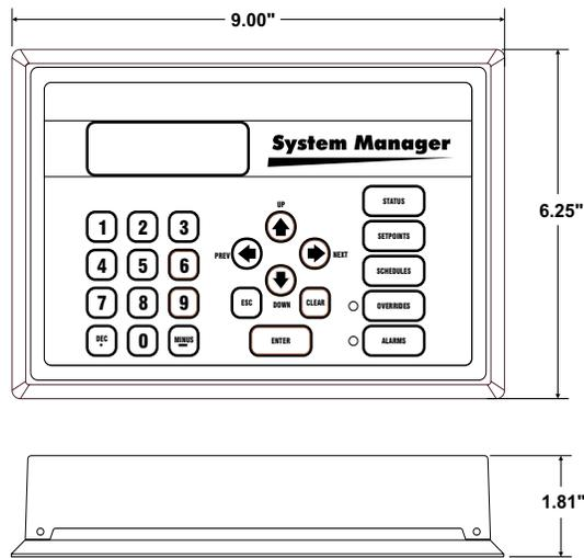
**Figure 3: Modular System Manager SD Dimensions**
