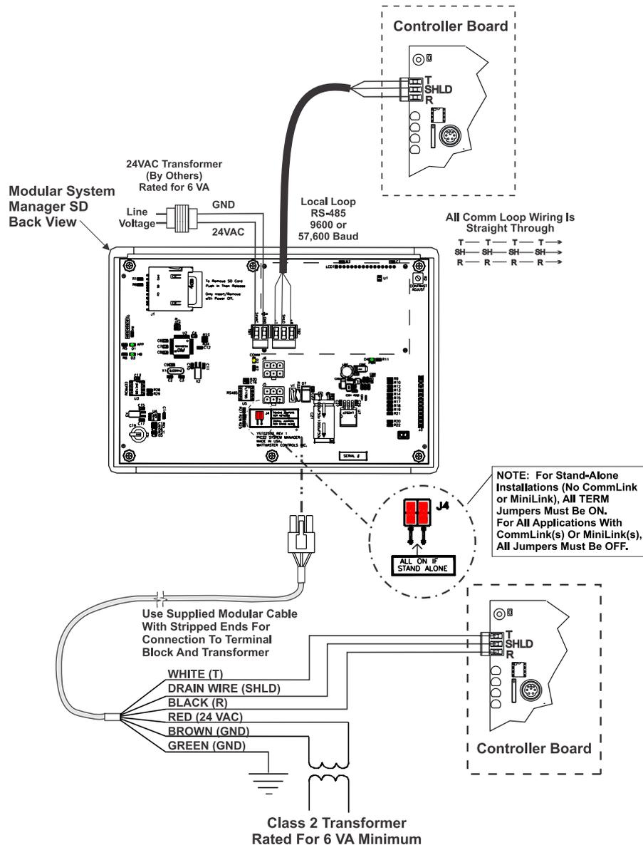
Figure 4: Modular System Manager SD Connection and Wiring Details
