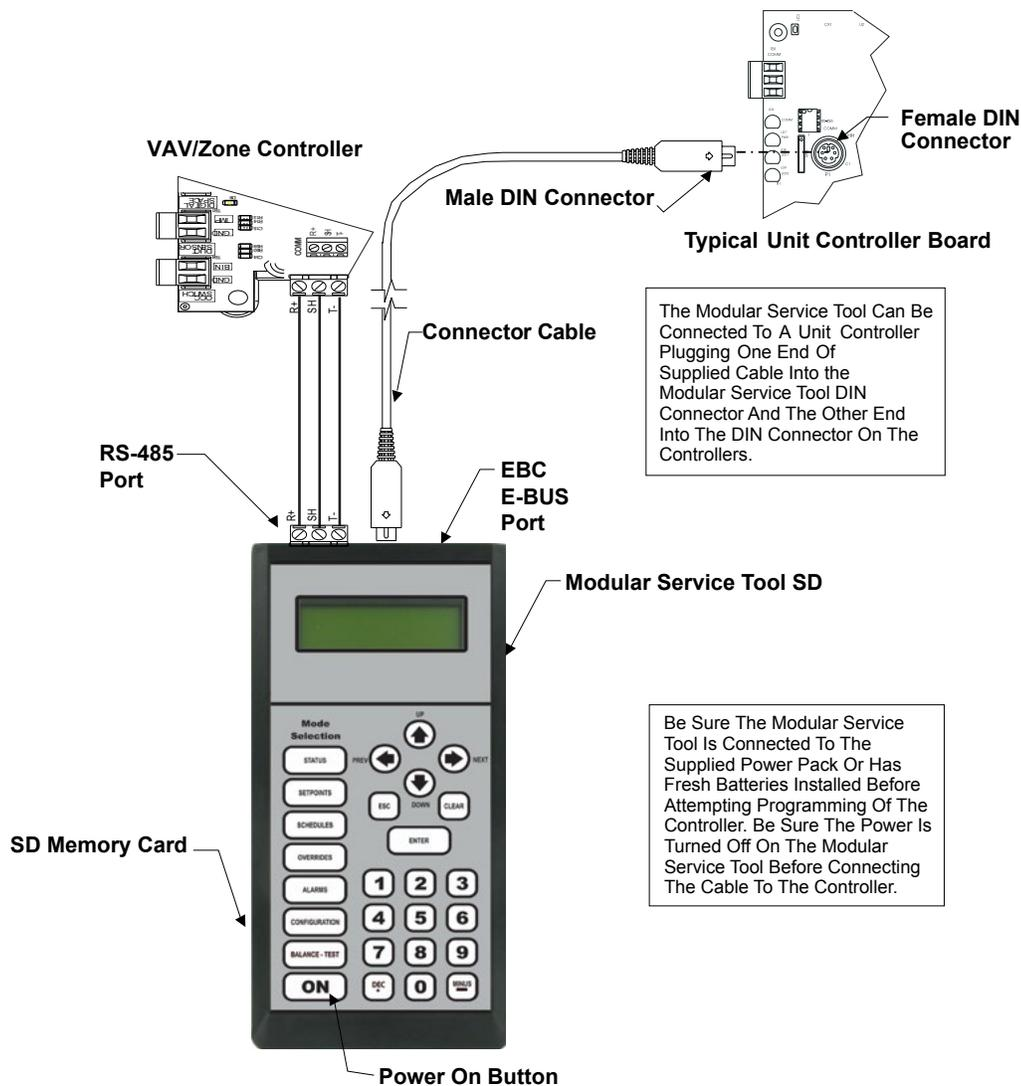
Figure 2: Modular Service Tool SD
