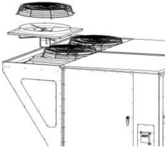
Figure 24 - Removal of a Condenser Fan Assembly
