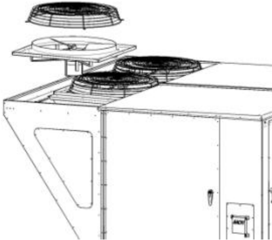
Figure 12 - Removal of a Condenser Fan Assembly
