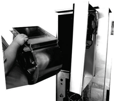
Figure 6 - Blower Assembly, Shown Pulled Away From Blower Panel
