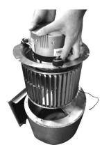
Separate the motor from the blower sub assembly, place the sub assembly (motor side down) and remove the set screw as shown below.
