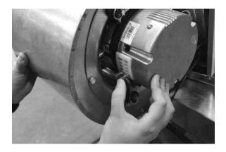
Adjustment for the A cabinet units (WH006-012) is made by adjusting the DC voltage signal to the motor from the Pioneer Expansion board or the Pioneer Gold board. Low fan speed is achieved by connecting the compressor Y call from the thermostat to Y1
