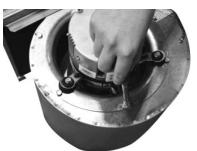
2) Pull the motor and blower up and out of the blower assembly.
