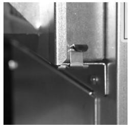
Figure 8 - Filter Rack Closed with Clip
