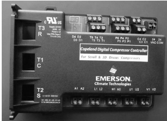
Figure 13 - Variable Capacity Compressor Controller
