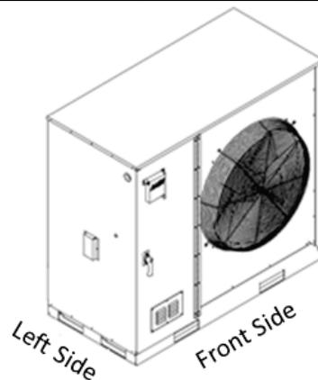
Figure 4 - Orientation of Series 2-7 ton Condensing Unit
