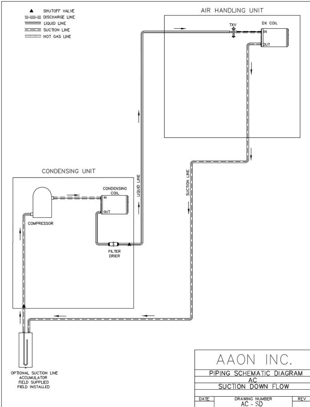
Figure 17 - A/C Split System Piping, Suction Down
