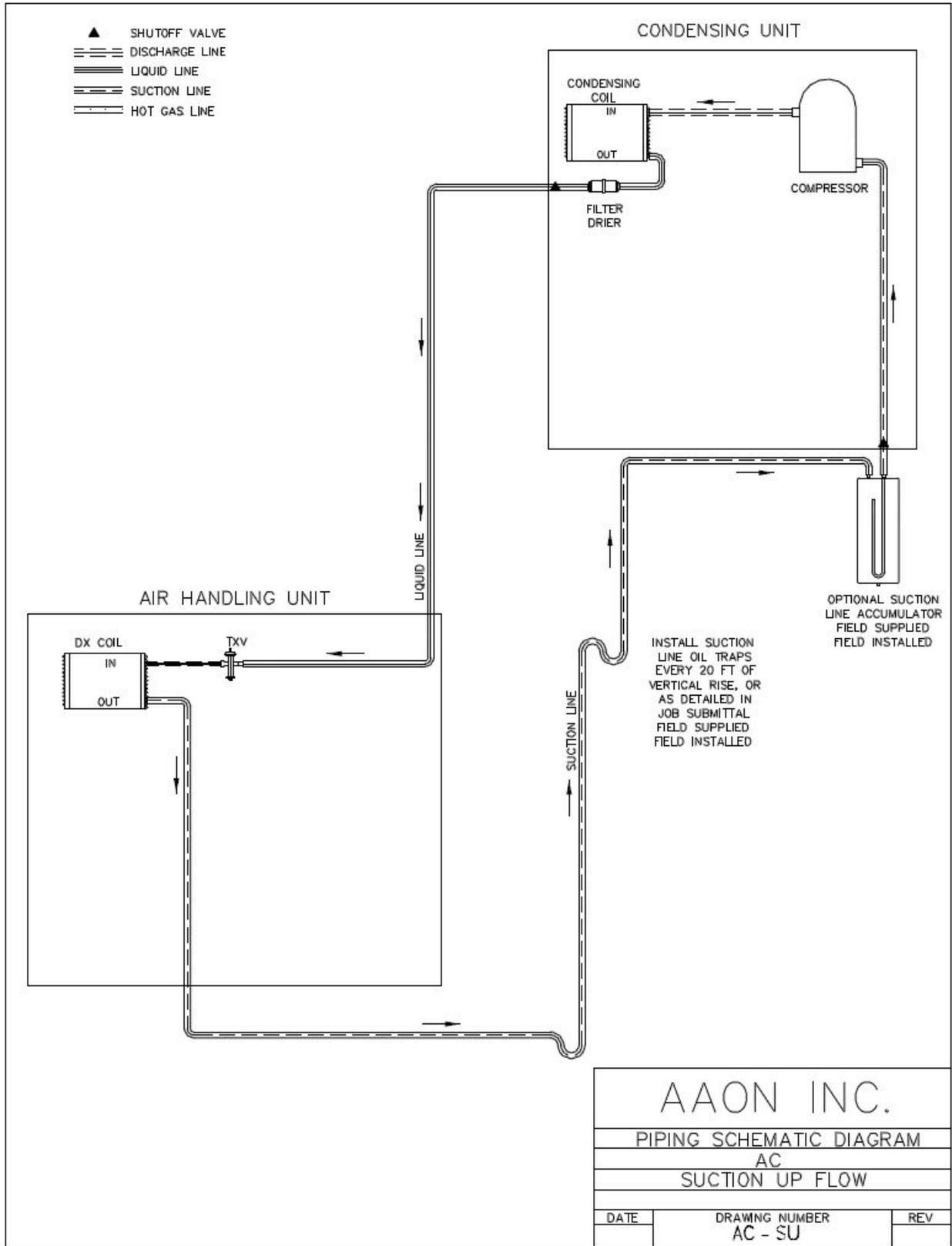
Figure 18 - A/C Split System Piping, Suction Up
