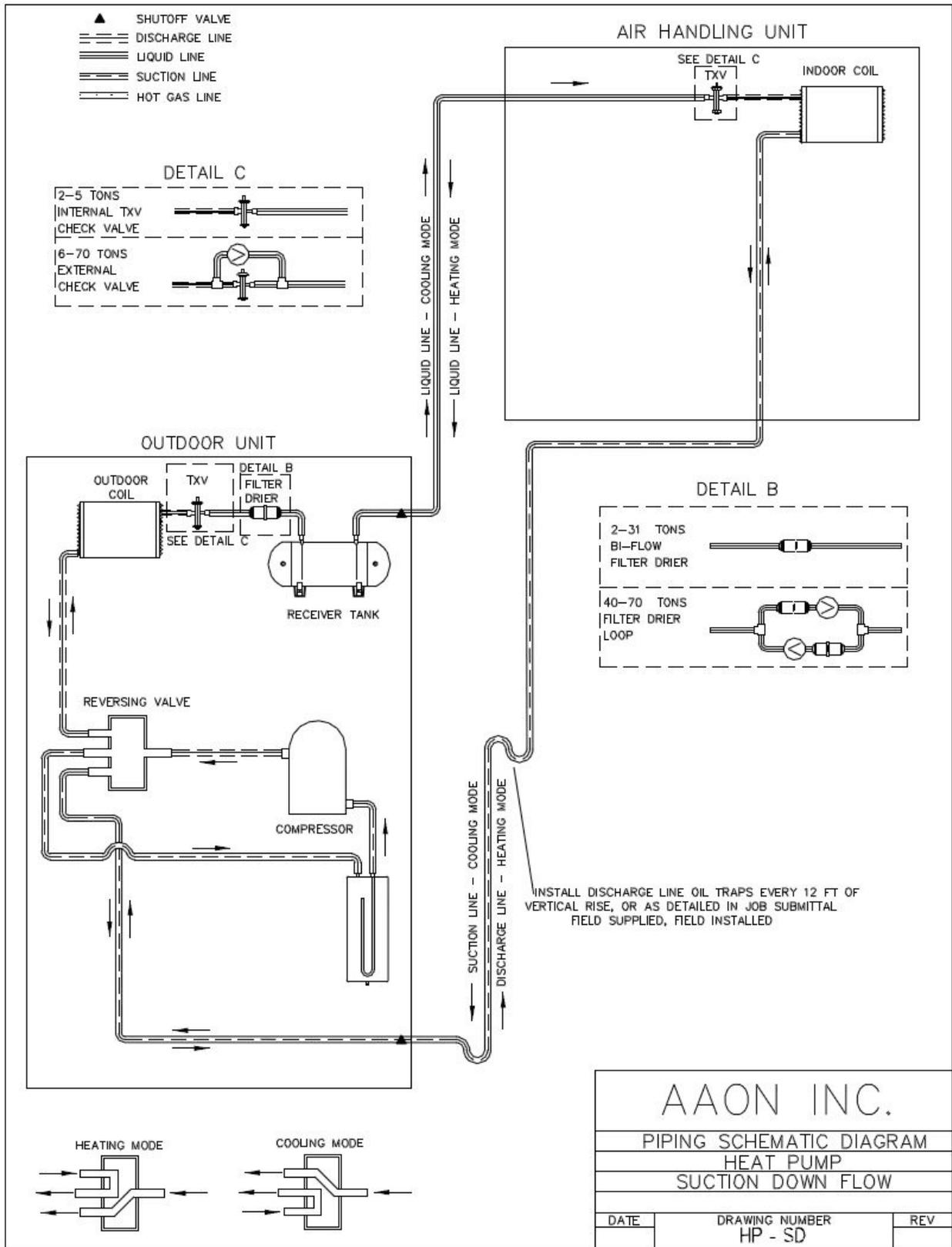
Figure 33 - Heat Pump Split System Piping, Suction Down
