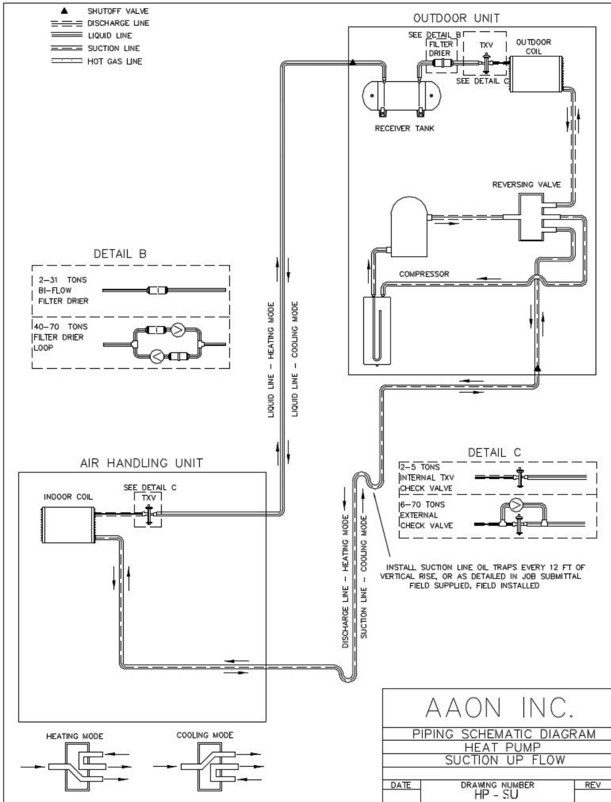
Figure 34 - Heat Pump Split System Piping, Suction Up
