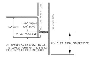
Figure 24 - Hot Gas Purge Circuit
