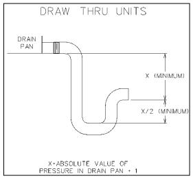
Figure 17 - Drain Trap
