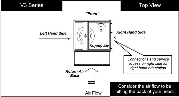
Figure 6 - V3 Series Unit Orientation
