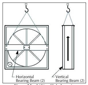
Figure 25 – Lifting Hole Locations
