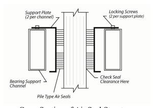
Cross Section of Air Seal Structure
