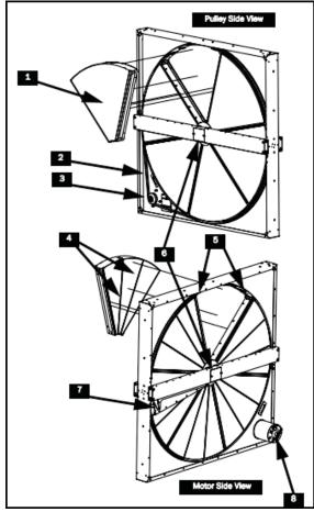
Figure 26 - Polymer Energy Recovery Wheel
