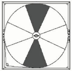
Figure 27 - Wheel Segment Removal Pattern
