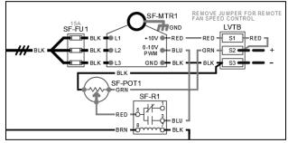
Figure 18 - Typical wiring diagram with EC motor
