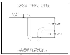
Figure 14 - Drain Trap
