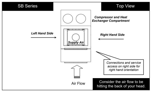
Figure 3 - SB Series Unit Orientation
