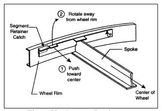
Figure 22 - Segment Retainer
