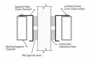
Figure 16 - Cross Section of Air Seal Structure
