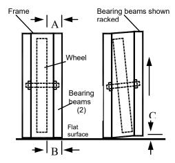
Figure 19 - Avoid Racking of Cassette Frame
