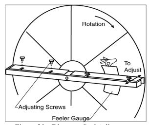
Figure 20 - Diameter Seal Adjustment
