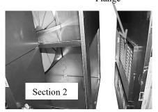
Figure 5 - Connect Sections
