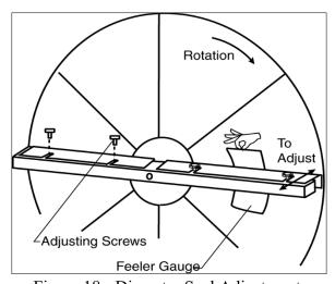
Figure 18 - Diameter Seal Adjustment
