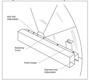
Figure 21 - Hub Seal Adjustment
