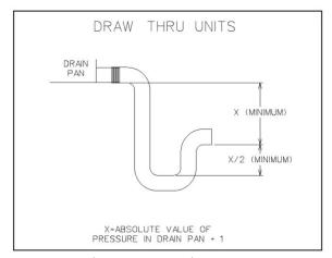
Figure 11 - Drain Trap
