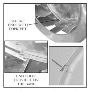
Figure 21 - Securing the Band
