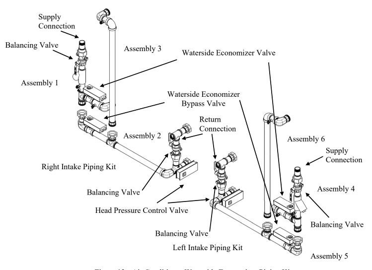
Figure 13 - Air Conditioner Waterside Economizer Piping Kit
