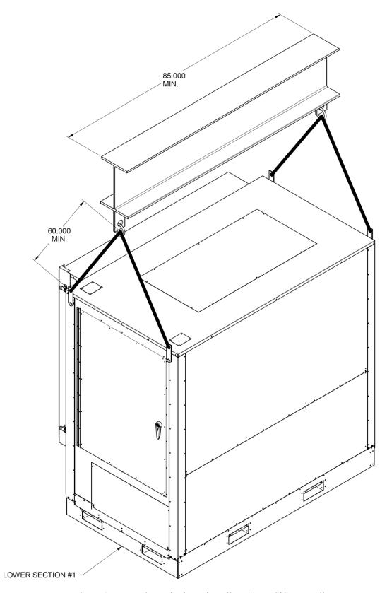
Figure 3 - Two Piece Single Unit Coil Section Lifting Details
