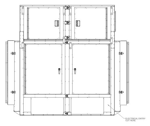
Figure 10 - Dual unit with splices after being bolted together.
