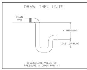
Figure 11 - Drain Trap
