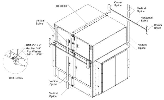
Figure 9 - Dual Unit Assembly Details
