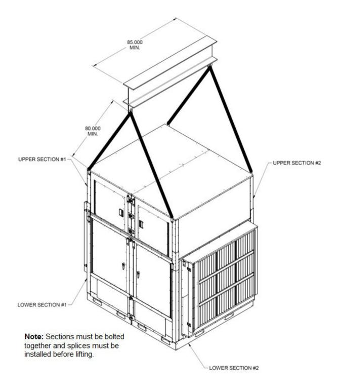
Figure 5- One Piece Dual Unit Lifting Details
