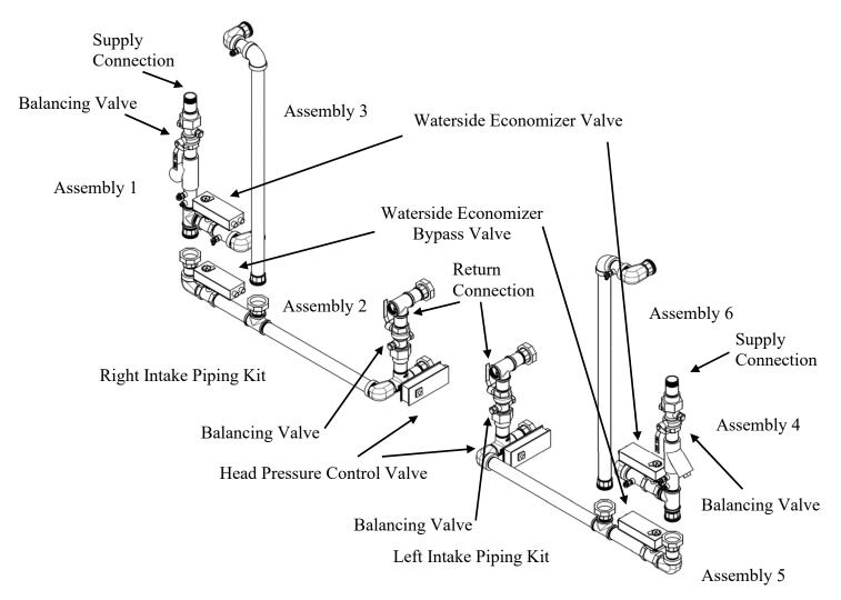
Figure 13 - Air Conditioner Waterside Economizer Piping Kit
