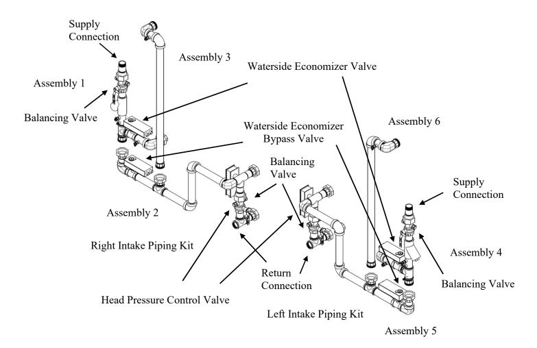
Figure 15 - Water-Source Heat Pump Waterside Economizer Piping Kit
