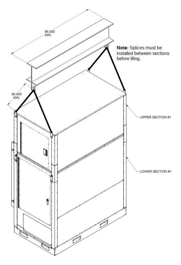
Figure 2 - One Piece Single Unit Lifting Details
