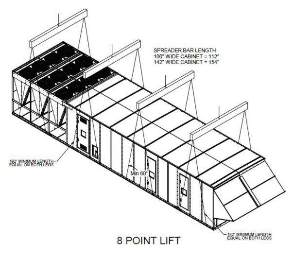
Figure 5 - 8 Point Lift RZ Series Air-Cooled Condenser Unit
