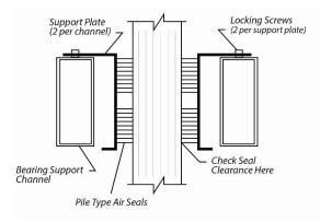
Cross Section of Air Seal Structure
