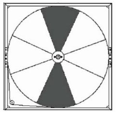
Figure 35 - Polymer Wheel Segment Removal Pattern
