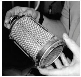
Figure 27 - RPE-48-BD filter element
