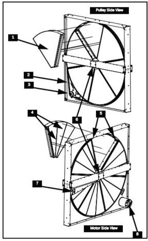
Figure 34 - Polymer Energy Recovery Wheel
