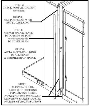
Figure 9 - Unit Base and Sides
