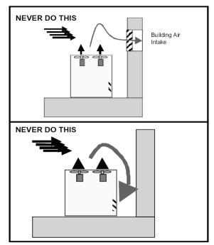
Figure 29 - Improper Unit Locations
