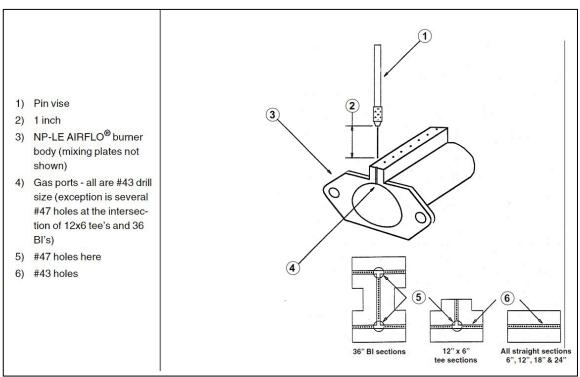
Figure 42 - Removing Piping Scale with Pin Vise
