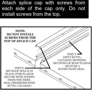
Figure 10 - Unit Roof Flange Splice Detail
