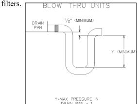
Figure 18 - Blow-Through Drain Trap
