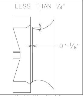
Note: 1/4" = 6.35 mm, 1/8" = 3.18 mm Figure 23 - Plenum Fan Gap Tolerances
