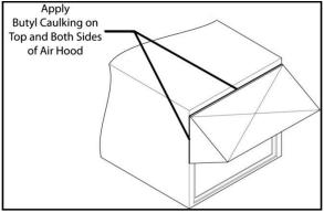
Figure 12 - Air Hood Shown in the Open Position
