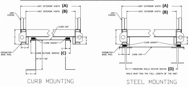
Figure 8 - Curb & Steel Mounting Rail with Dimensions
