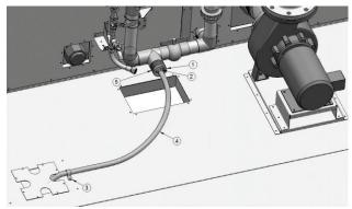
Figure 30 - Temporary Drain Components
