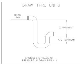
Figure 17 - Draw-Through Drain Trap
