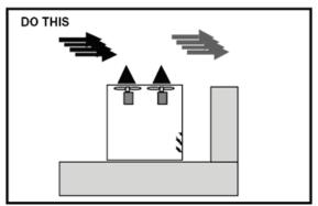
Figure 28 - Proper Unit Location
