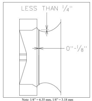
Figure 23 - Plenum Fan Gap Tolerances
