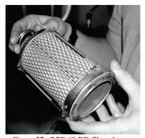
Figure 27 - RPE-48-BD filter element
