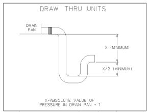
Figure 17 - Draw-Through Drain Trap
