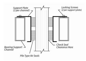
Cross Section of Air Seal Structure
