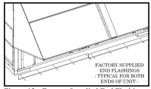
Figure 13 - Factory Supplied End Flashings
