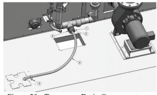
Figure 30 - Temporary Drain Components
