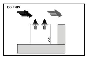
Figure 28 - Proper Unit Location
