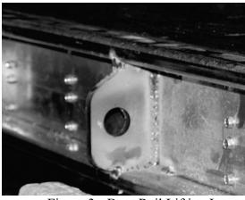
Figure 3 - Base Rail Lifting Lug
