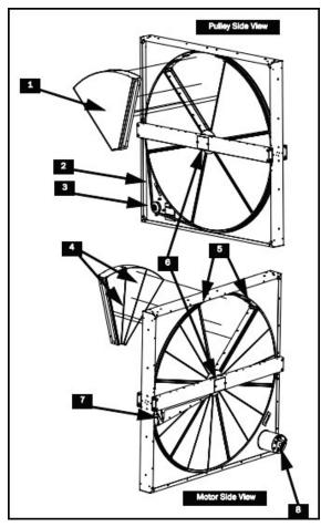
Figure 33 - Polymer Energy Recovery Wheel
