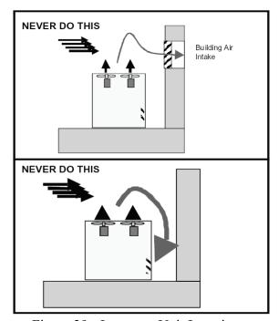
Figure 29 - Improper Unit Locations
