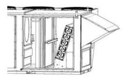
Figure 40 - Evaporator Coil Access
