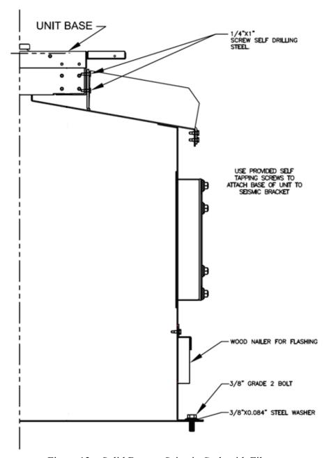
Figure 12 – Solid Bottom Seismic Curb with Filters
