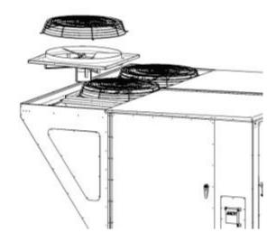
Figure 41 - Removal of a Condenser Fan Assembly
