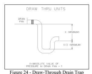
The X dimension on the draw-through trap must be at least equal to the absolute value of the negative static pressure in the drain pan plus one inch. To calculate the static pressure at the drain pan add the pressure drops of all components upstream of the drain pan, including the cooling coil, and add the return duct static pressure. Include the dirt
