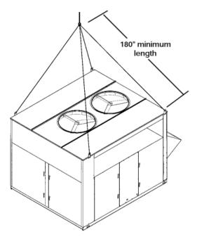
Figure 10 - Lifting Details of a 26, 31-50, 60 and 70 ton Unit
