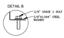
Figure 15 - Seismic Solid Bottom Curb without Filters Detail B
