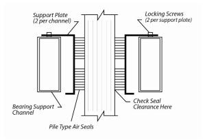
Cross Section of Air Seal Structure
