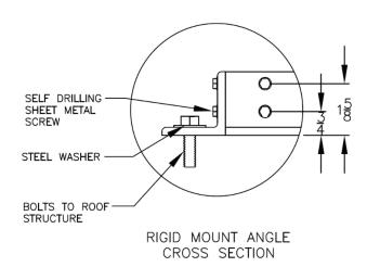
Figure 16 - Seismic Rigid Mount Curb
