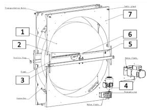
Figure 43 - Aluminum Energy Recovery Wheel
