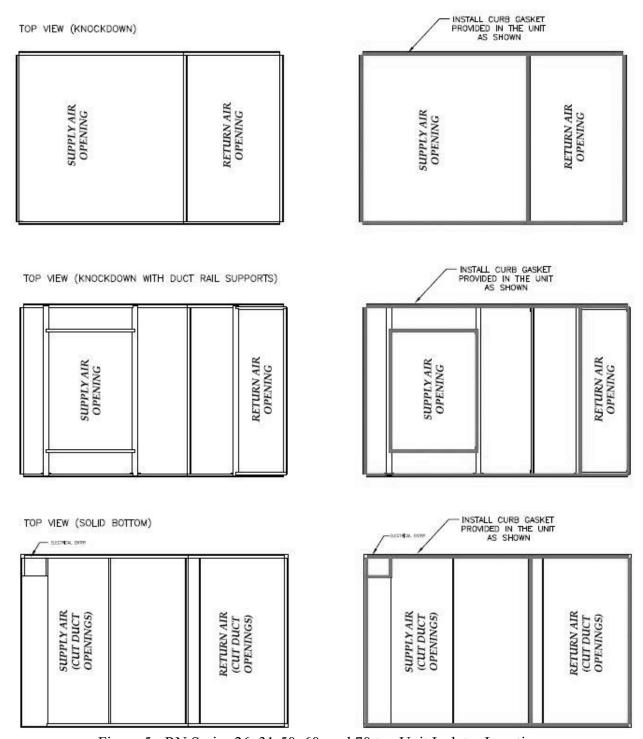
Figure 5 - RN Series 26, 31-50, 60, and 70 ton Unit Isolator Locations
