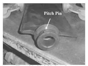
Figure 34 - Pitch Pin Location
