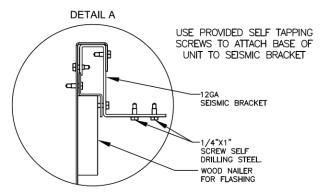
Figure 14 - Seismic Solid Bottom Curb without Filters Detail A
