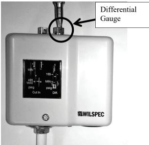
To raise the pressure set point for the **DIFFERENTIAL** Gauge, turn the adjustable screw clockwise.
