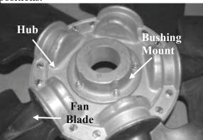
Figure 31 - Assembled Fan
