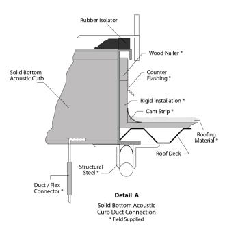
Figure 11 - Duct Connection
