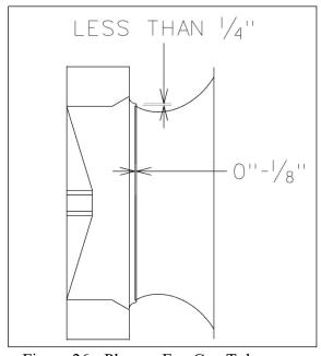
Figure 26 - Plenum Fan Gap Tolerances
