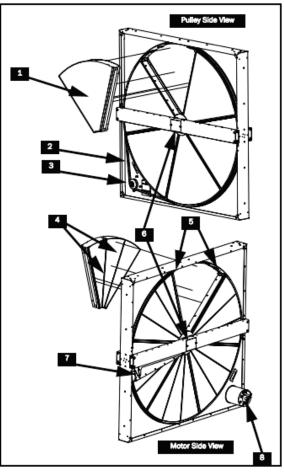
Figure 45 - Polymer Energy Recovery Wheel
