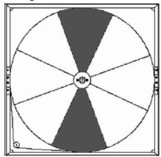
Figure 46 - Wheel Segment Removal Pattern
