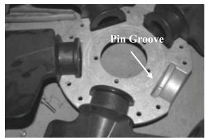
Figure 33 - Pin Groove Location
