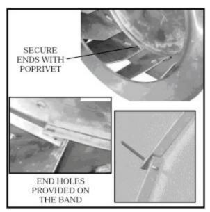
Figure 25 - Supply Fan Banding
