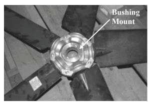
Figure 27 - Fan with the HUB on the Top and RET on the Bottom
