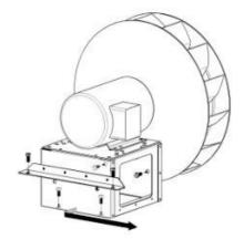
Figure 37 - Bolts which Connect Motor Mount to Blower Fan
