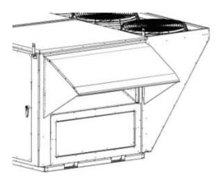
Figure 18 – 6-25 and 30 ton Open Rain Hood
