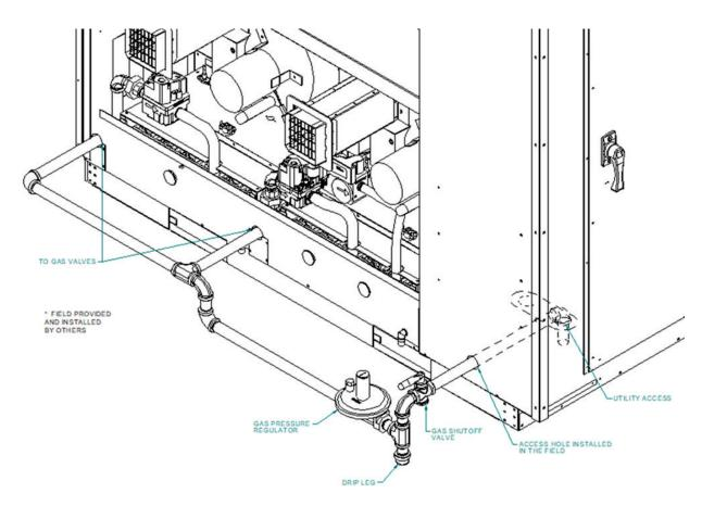
Figure 51 - Example 6-50, 60 & 70 ton through the Base Gas Piping
