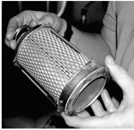
Figure 42 - RPE-48-BD filter element
