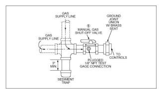
Figure 31 - Sediment Trap for Gas Heat
