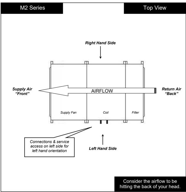
Figure 2 - Unit Orientation
