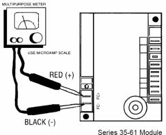
Figure 49 - Flame Sensor Current Check
