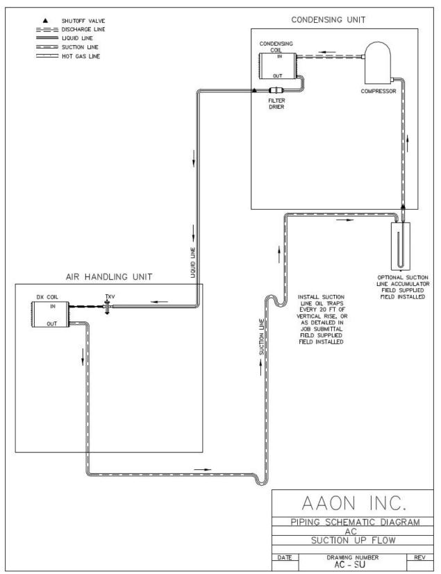
Figure 55 - A/C Split System Piping, Suction Up
