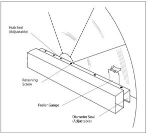
Figure 42 - Hub Seal Adjustment
