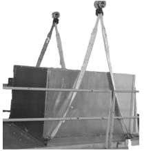
Figure 7 - M2 Series Individual Module Bottom Tier Lifting
