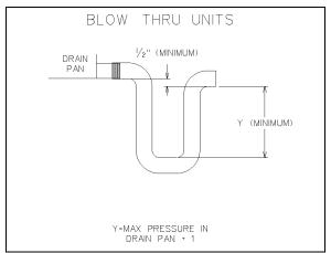
Figure 27 - Blow-Through Drain Trap
