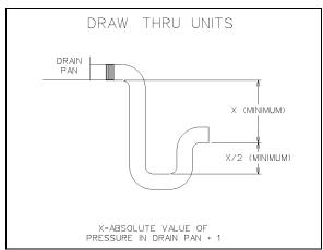
Figure 26 - Draw-Through Drain Trap
