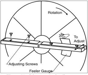
Figure 41 - Diameter Seal Adjustment
