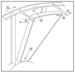
Figure 44 - Segment Installation
