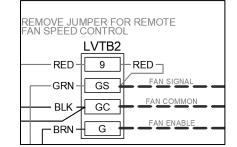
Figure 28 – Jumper for Remote Fan Speed Control
