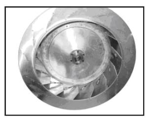
Figure 30 - Supply Fan Banding
