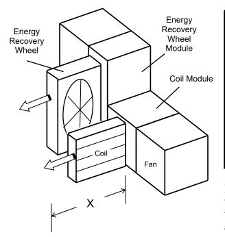
Figure 4 - Service Access Clearance
