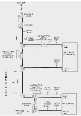
Figure 22 – Waterside Economizer Piping
