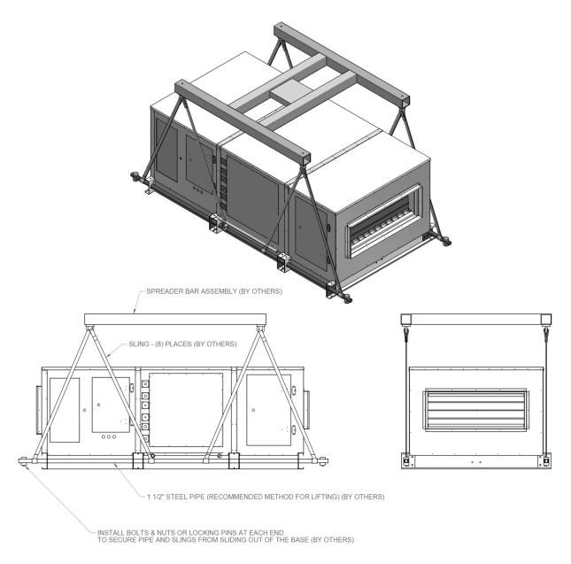
Figure 6 - M2 Series Unit Eight Point Lifting
