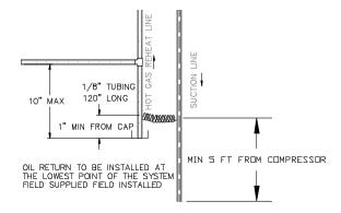
Figure 24 - Hot Gas Purge Circuit
