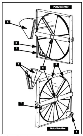
Figure 26 - Polymer Energy Recovery Wheel
