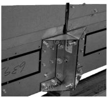
Figure 13 - Forklift Base Assembly
