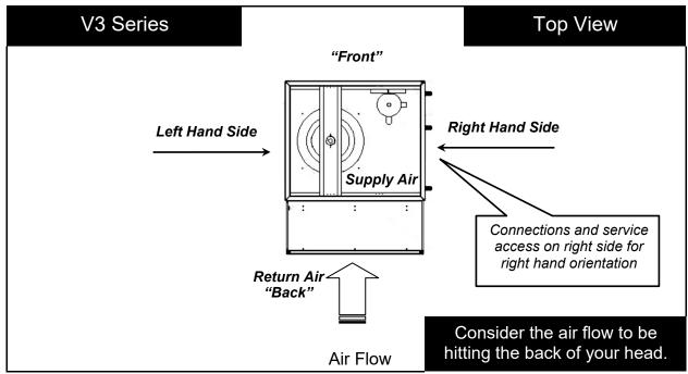
Figure 6 - V3 Series Unit Orientation
