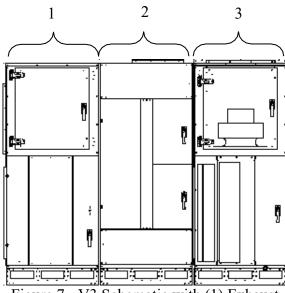
Figure 7 - V3 Schematic with (1) Exhaust Fan, (2) Energy Recovery, (3) Air Handler
