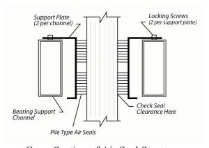
Cross Section of Air Seal Structure
