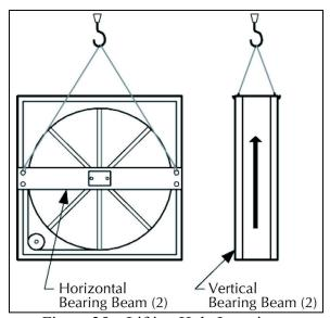
Figure 25 – Lifting Hole Locations
