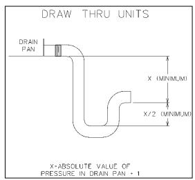
Figure 17 - Drain Trap
