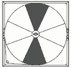
Figure 27 - Wheel Segment Removal Pattern
