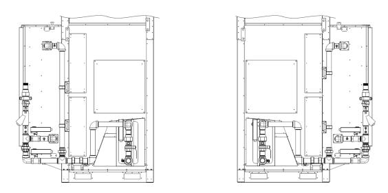
Figure 16 - Water-Source Heat Pump Waterside Economizer Back View
