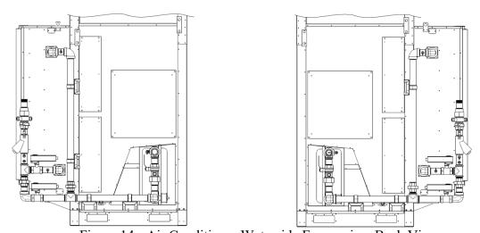
Figure 14 - Air Conditioner Waterside Economizer Back View
