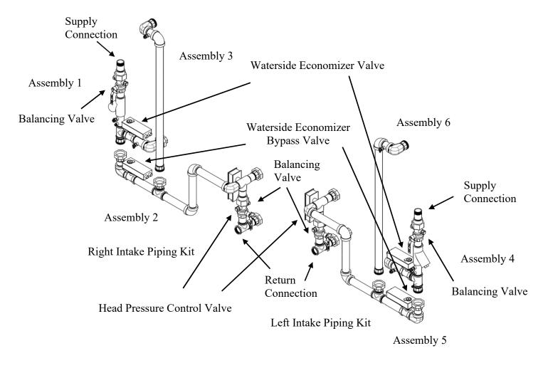
Figure 15 - Water-Source Heat Pump Waterside Economizer Piping Kit
