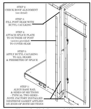
Figure 9 - Unit Base and Sides
