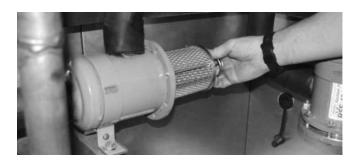
6. Replace the suction filter end plate and bolts
