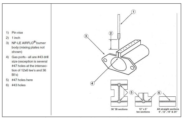
Figure 41 - Removing Piping Scale with Pin Vise
