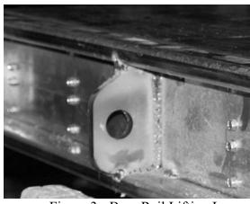
Figure 3 - Base Rail Lifting Lug
