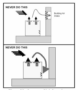
Figure 29 - Improper Unit Locations
