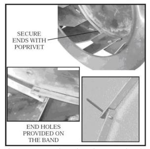
Figure 22 - Securing Air Volume Band Ends
