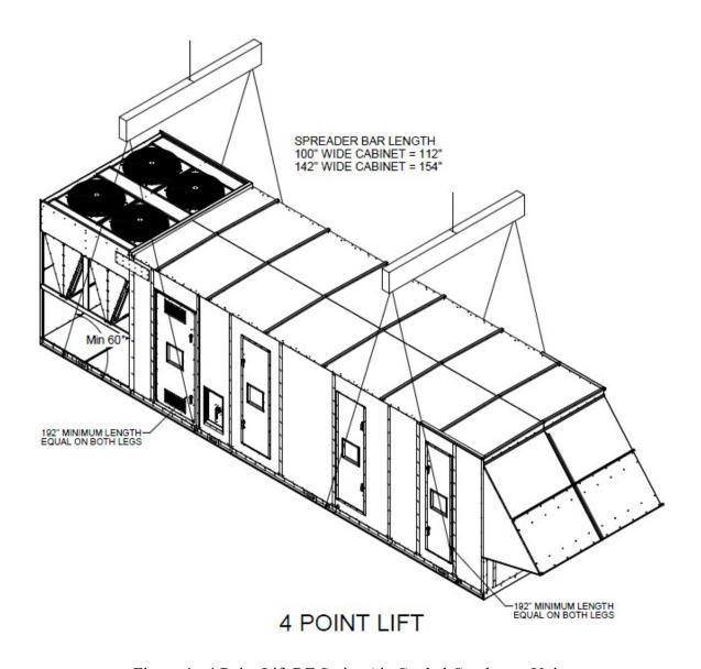
Figure 4 - 4 Point Lift RZ Series Air-Cooled Condenser Unit
