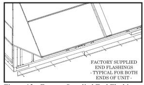
Figure 13 - Factory Supplied End Flashings
