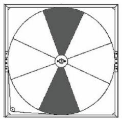
Figure 34 - Polymer Wheel Segment Removal Pattern
