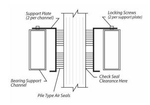
Cross Section of Air Seal Structure
