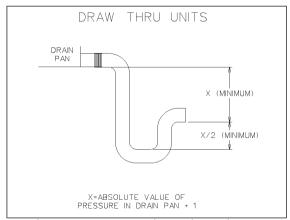
Figure 17 - Draw-Through Drain Trap
