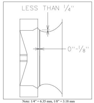
Figure 23 - Plenum Fan Gap Tolerances
