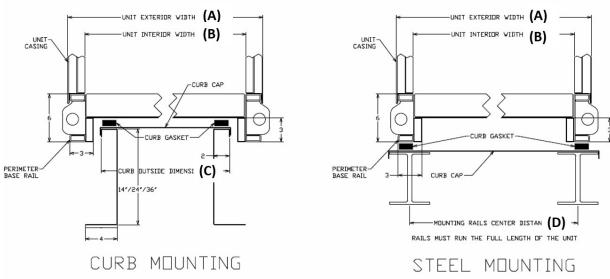
Figure 8 - Curb & Steel Mounting Rail with Dimensions
