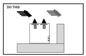
Figure 28 - Proper Unit Location
