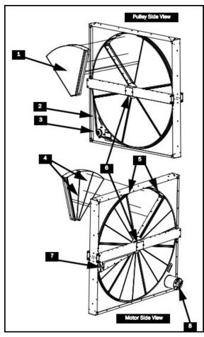
Figure 33 - Polymer Energy Recovery Wheel
