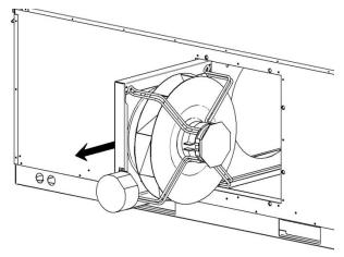
Figure 28 - RQ Supply Fan Removal Slide
