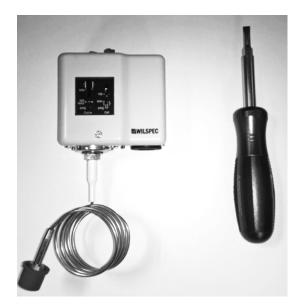
To adjust the fan cycle switch you will need a flathead screwdriver.
