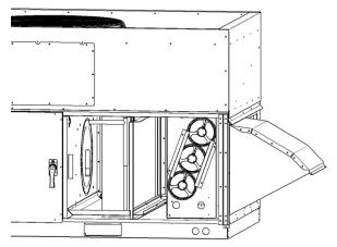
Figure 31 - Evaporator Coil Access
