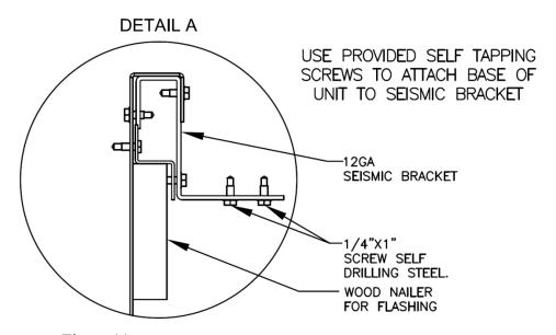
Figure 11 - Seismic Solid Bottom Curb without Filters Detail A
