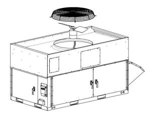
Figure 32 - Removal of a Condenser Fan Assembly
