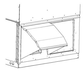
Figure 16 - RQ Series unit Open Rain Hood
