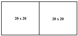
Figure 38 - RQ Series 2-6 ton Standard Filter Layout (Viewed from the Upstream Side of the Cooling Coil)
