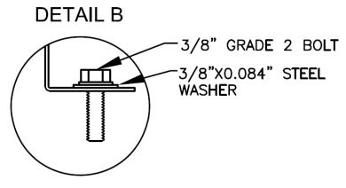
Figure 12 - Seismic Solid Bottom Curb without Filters Detail B
