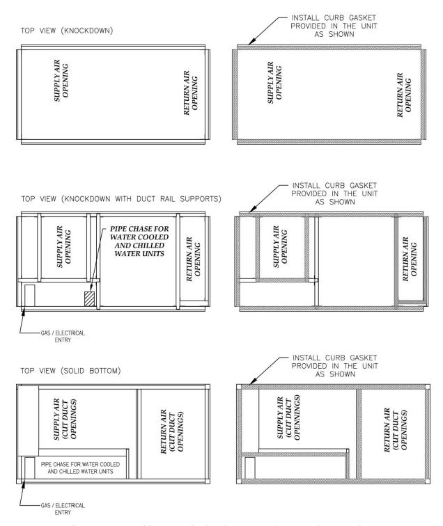
Figure 3 - RQ Cabinet Standard and Power Exhaust Gasket Locations
