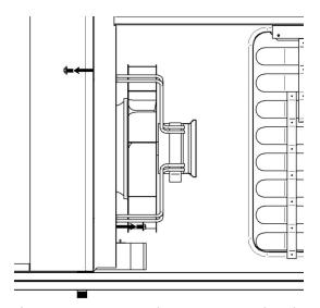
Figure 27 - RQ Supply Fan Removal Bolts
