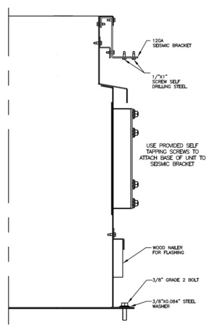
Figure 9 - Solid Bottom Seismic Curb with Filters
