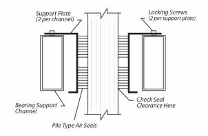
Cross Section of Air Seal Structure
