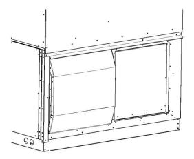
Figure 15 - RQ Series unit Closed Rain Hood
