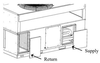
Figure 14 - Horizontal duct connections
