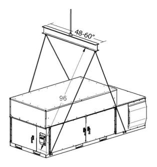
Figure 7 - Lifting Details of a 2-6 ton Energy Recovery Wheel Unit
