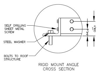
Figure 13 - Seismic Rigid Mount Curb Cross Section
