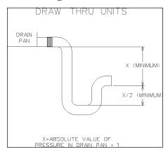
Figure 20 - Draw-Through Drain Trap
