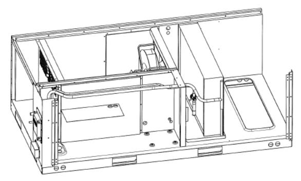
Figure 23 - Post Corner Hole Piping
