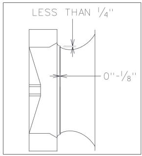
Figure 28 - Plenum Fan Gap Tolerances
