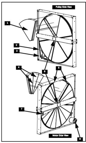
Figure 47 - Polymer Energy Recovery Wheel
