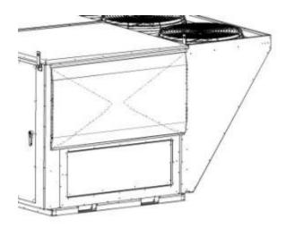
Figure 18 - 11, 13 and 16-30 ton Closed Rain Hood
