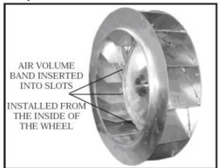
The following photos of a wheel are provided for practical guidelines only in order to identify the air band location in the wheel. Actual field installation of the air band into the wheel will require access into and through the blower wheel venture, which may require removal of the blower motor and wheel.
