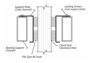
Cross Section of Air Seal Structure
