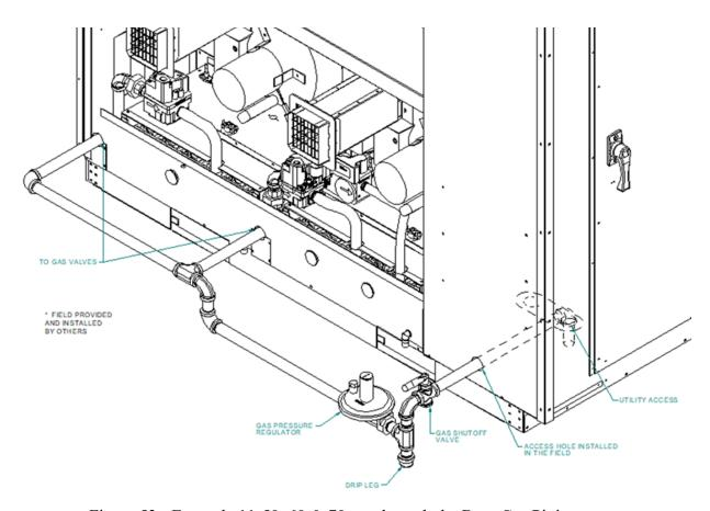
Figure 53 - Example 11-50, 60 & 70 ton through the Base Gas Piping
