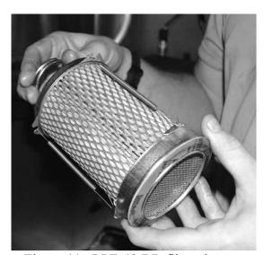
Figure 44 - RPE-48-BD filter element
