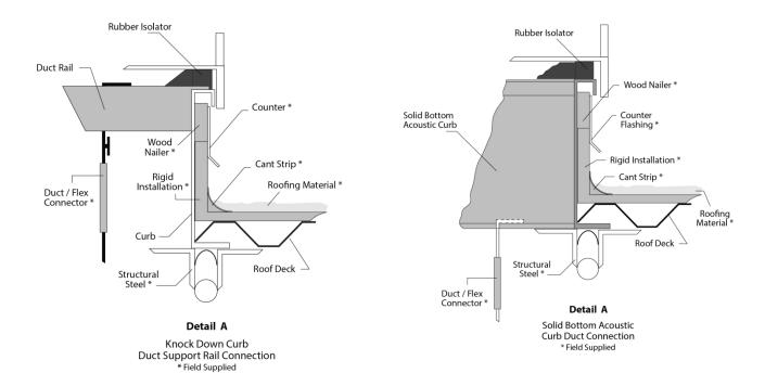
Figure 12 - Duct Connection
