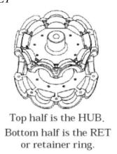
Figure 32 - Fan HUB and RET Castings
