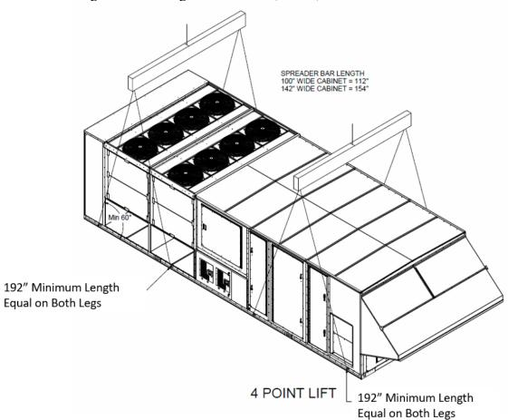
Figure 11 - Lifting Details of a 55, 65 and 75-140 ton Unit
