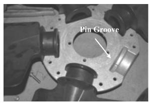
Figure 35 - Pin Groove Location
