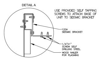
Figure 15 - Seismic Solid Bottom Curb without Filters Detail A
