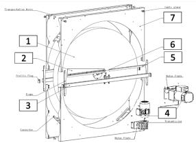
Figure 45 - Aluminum Energy Recovery Wheel
