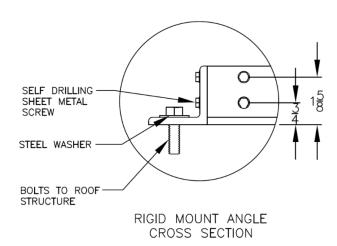
Figure 17 - Seismic Rigid Mount Curb
