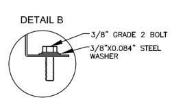
Figure 16 - Seismic Solid Bottom Curb without Filters Detail B
