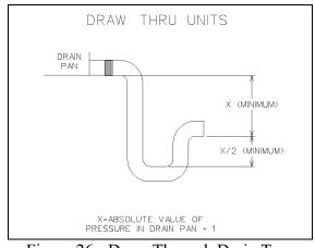
Figure 26 - Draw-Through Drain Trap
