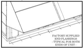
Figure 21 - Factory Supplied End Flashings
