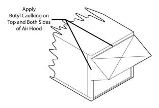
Figure 20 - 26 and 31-70 ton Open Rain Hood
