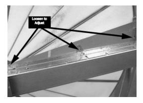
1. Loosen the three purge adjusting screws.
