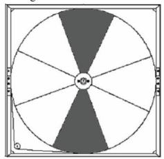
Figure 48 - Wheel Segment Removal Pattern
