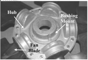
Figure 33 - Assembled Fan
