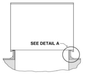
SECTIONAL VIEW OF UNIT ON ROOF CURB
