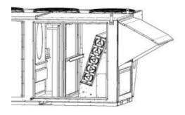
Figure 42 - Evaporator Coil Access
