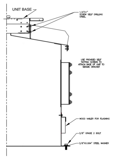
Figure 13 – Solid Bottom Seismic Curb with Filters
