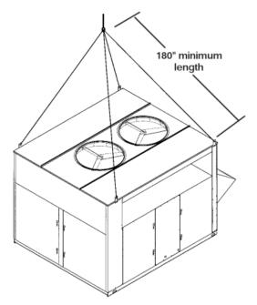
Figure 10 - Lifting Details of a 26, 31-50, 60 and 70 ton Unit
