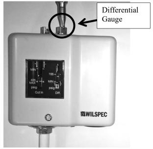
To lower the pressure set point for the **DIFFERENTIAL** Gauge, turn the adjustable screw counter clockwise.
