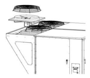
Figure 43 - Removal of a Condenser Fan Assembly
