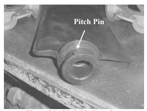
Figure 36 - Pitch Pin Location
