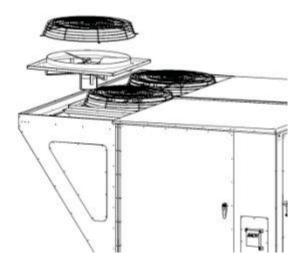
Figure 34 - Removal of a Condenser Fan Assembly
