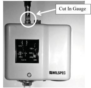
To raise the pressure set point for the **CUT IN** gauge, turn the adjustable screw counter clockwise.
