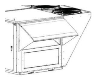
Figure 22 - 6-25 and 30 ton Open Rain Hood
