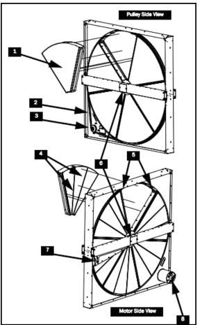
Figure 38 - Polymer Energy Recovery Wheel
