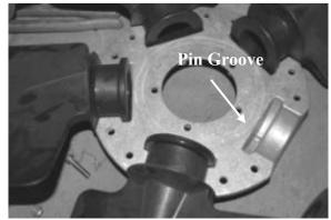
Figure 26 - Pin Groove Location
