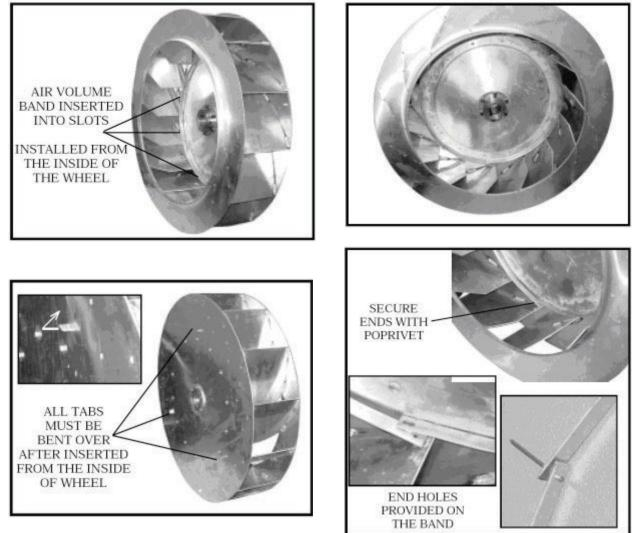
Figure 18 - Supply Fan Banding
