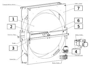
Figure 36 - Aluminum Energy Recovery Wheel
