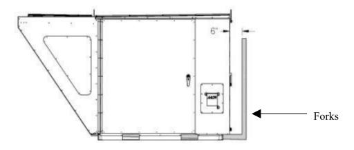
Figure 7 - Forklifting an RN Series A, B and C Cabinet, 6-25 and 30 tons
