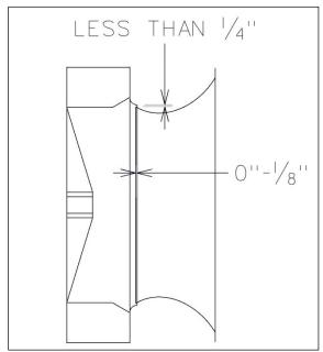
Figure 19 - Plenum Fan Gap Tolerances
