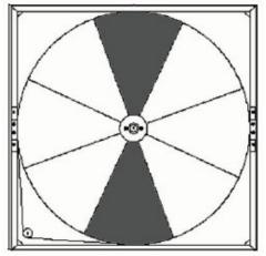
Figure 39 - Wheel Segment Removal Pattern
