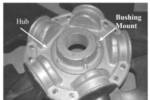
Figure 24- Assembled Fan
