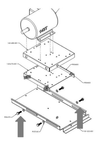
2. Remove the belt tensioner bolt completely, as indicated by the arrow below.
