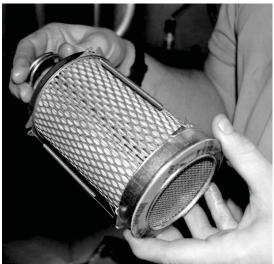
Figure 35 - RPE-48-BD filter element
