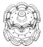
Top half is the HUB. Bottom half is the RET or retainer ring. Figure 23 - Fan HUB and RET Castings
