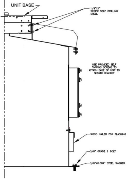
Figure 11 - Solid Bottom Seismic Curb with Filters
