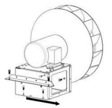
Figure 30 – Bolts which connect motor mount to fan
