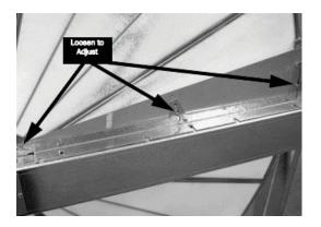
1. Loosen the three purge adjusting screws.
