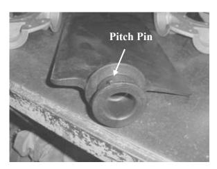
Figure 27 - Pitch Pin Location
