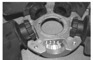
Figure 22 - RET with Pin in Groove 4
