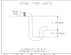
Figure 17 - Draw-Through Drain Trap
