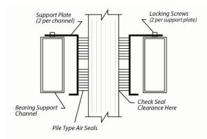
Cross Section of Air Seal Structure
