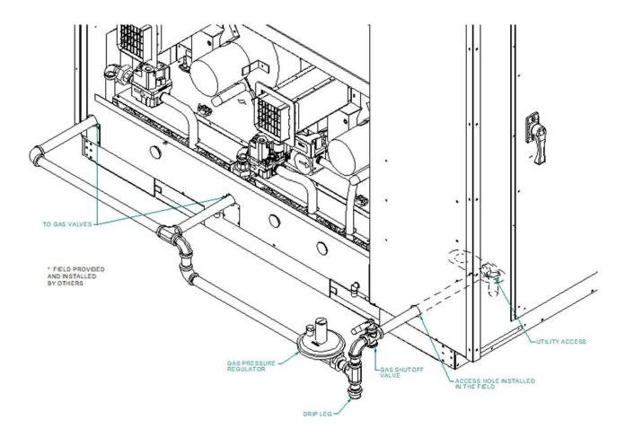
Figure 44 - Example 6-30 ton External Gas Piping
