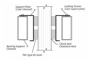
Cross Section of Air Seal Structure
