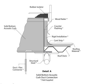
Figure 4 - Duct Connection
