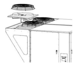
Figure 12 - Removal of a Condenser Fan Assembly
