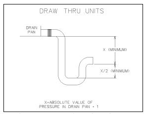
Figure 9 - Draw-Through Drain Trap
