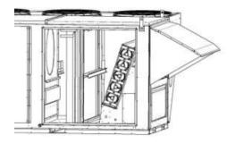
Figure 11 - Evaporator Coil Access
