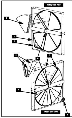
Figure 16 - Polymer Energy Recovery Wheel
