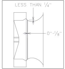
Figure 10 - Plenum Fan Gap Tolerances
