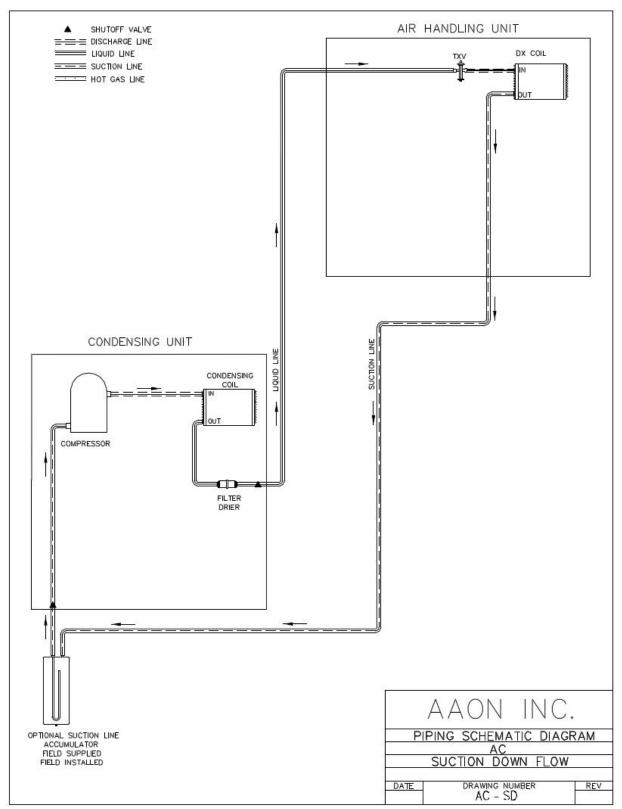
Figure 54 - A/C Split System Piping, Suction Down
