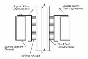
Figure 38 - Cross Section of Air Seal Structure
