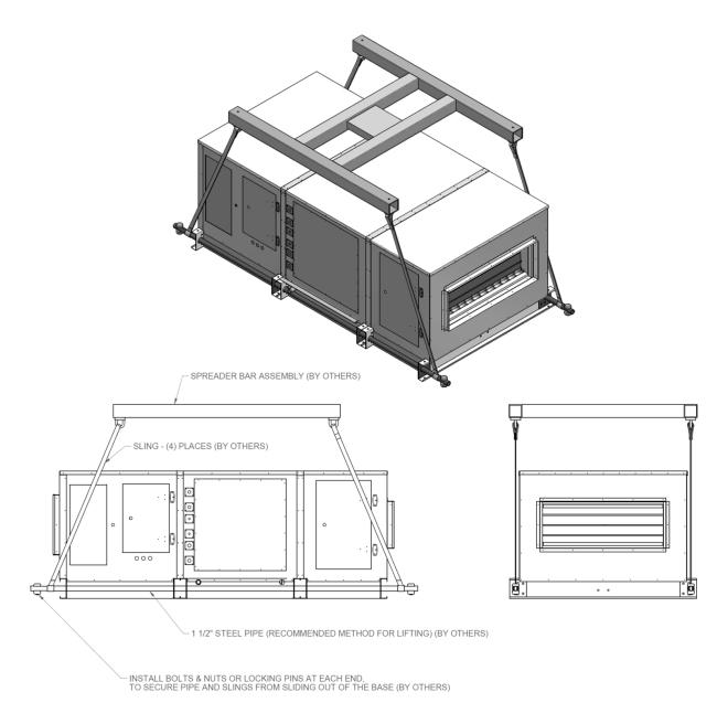
Figure 5 - M2 Series Unit Four Point Lifting
