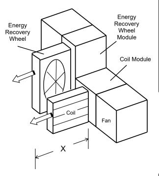
Figure 4 - Service Access Clearance
