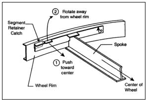
Figure 43 - Segment Retainer
