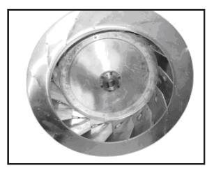
Figure 30 - Supply Fan Banding
