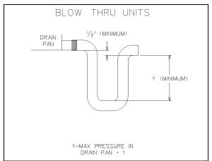
Figure 27 - Blow-Through Drain Trap
