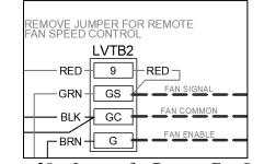
Figure 28 – Jumper for Remote Fan Speed Control
