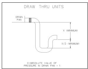
Figure 26 - Draw-Through Drain Trap
