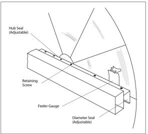
Figure 42 - Hub Seal Adjustment
