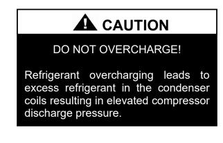
The system is undercharged if the superheat is too high and the sub-cooling is too low
