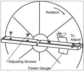
Figure 41 - Diameter Seal Adjustment
