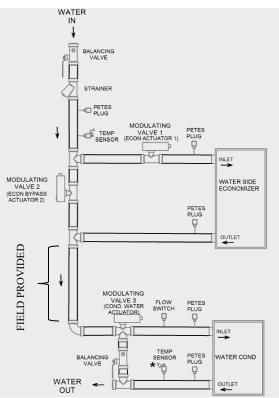
Figure 22 – Waterside Economizer Piping
