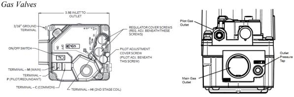
Figure 46 - Combination Gas Valve
