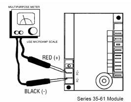
Figure 49 - Flame Sensor Current Check
