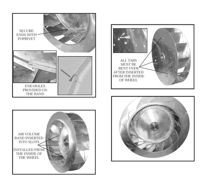
Figure 30 - Supply Fan Banding
