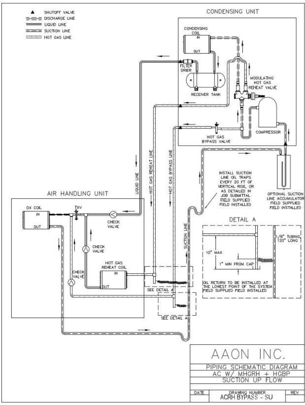
Figure 63 - A/C with Modulating Hot Gas Reheat and Hot Gas Bypass Split System Piping, Suction Up
