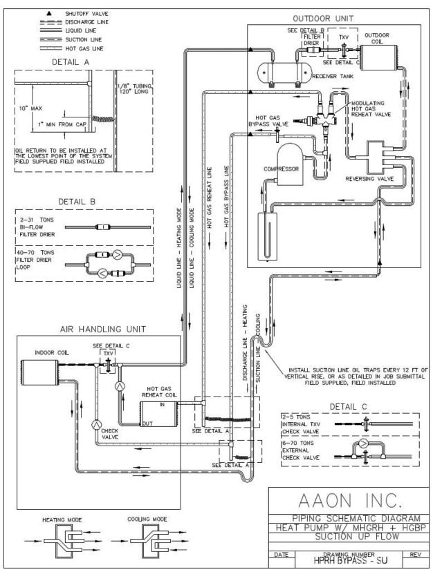
Figure 71 - Heat Pump with Modulating Hot Gas Reheat and Hot Gas Bypass Split System Piping, Suction Up
