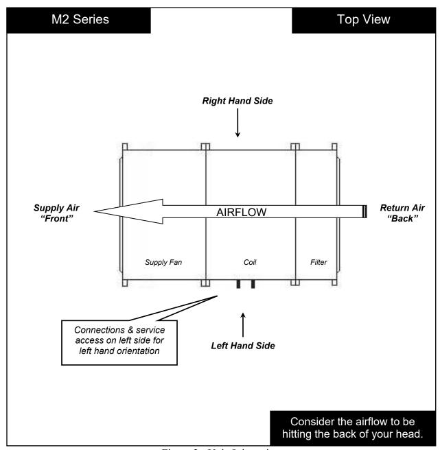
Figure 2 - Unit Orientation
