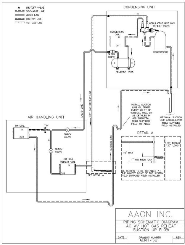
Figure 59 - A/C with Modulating Hot Gas Reheat Split System Piping, Suction Up
