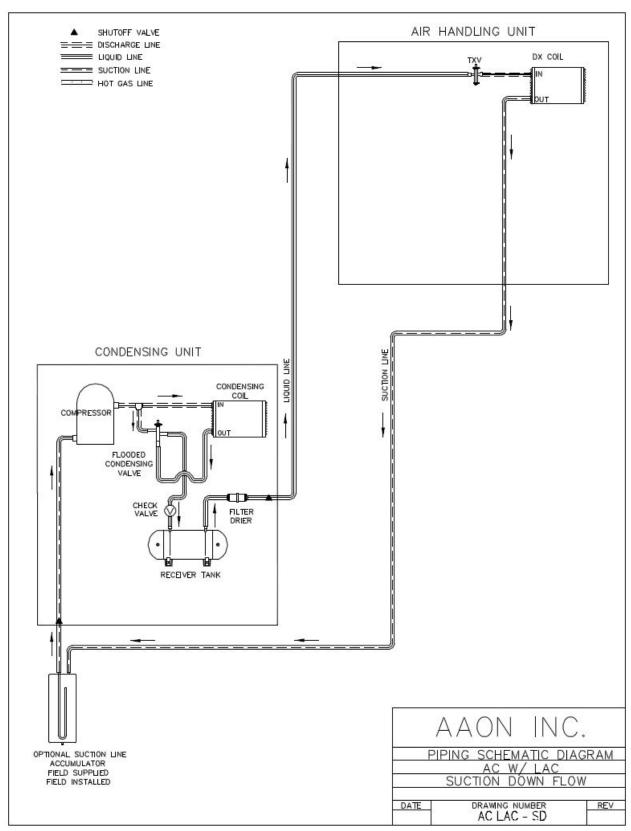
Figure 56 - A/C with LAC Split System Piping, Suction Down
