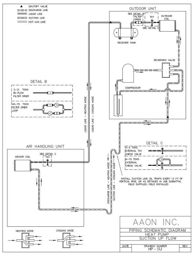
Figure 65 - Heat Pump Split System Piping, Suction Up
