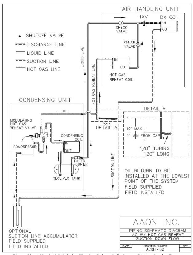
Figure 58 - A/C with Modulating Hot Gas Reheat Split System Piping, Suction Down
