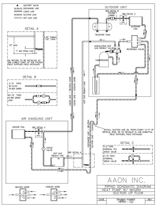
Figure 67 - Heat Pump with Modulating Hot Gas Reheat Split System Piping, Suction Up
