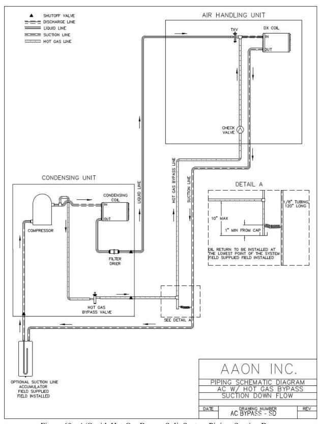
Figure 60 - A/C with Hot Gas Bypass Split System Piping, Suction Down
