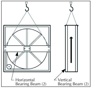
Figure 39 - Lifting Hole Locations
