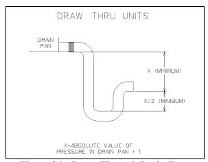
Figure 26 - Draw-Through Drain Trap
