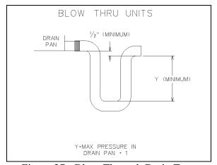
Figure 27 - Blow-Through Drain Trap
