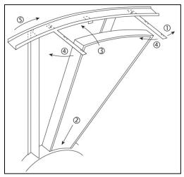
Figure 44 - Segment Installation
