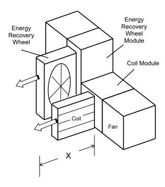
Figure 4 - Service Access Clearance
