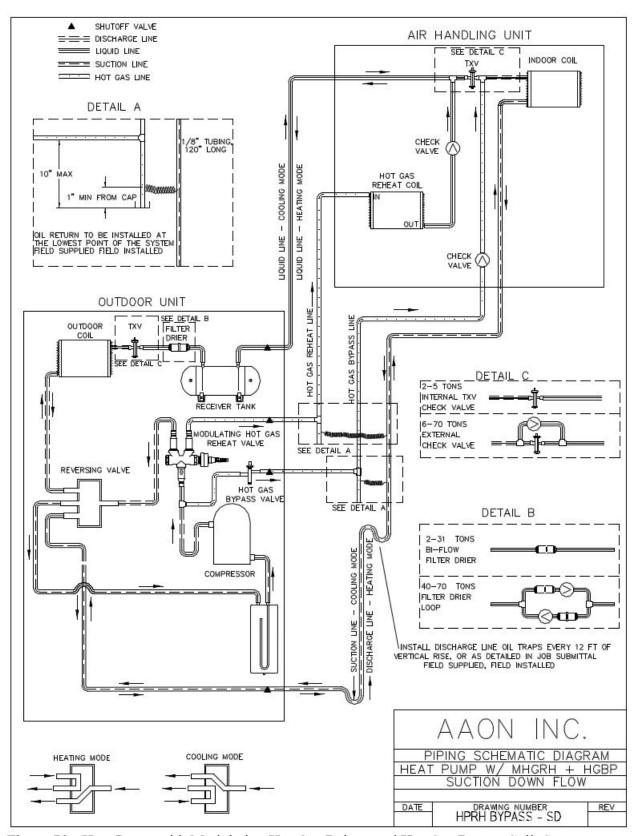
Figure 70 - Heat Pump with Modulating Hot Gas Reheat and Hot Gas Bypass Split System Piping, Suction Down
