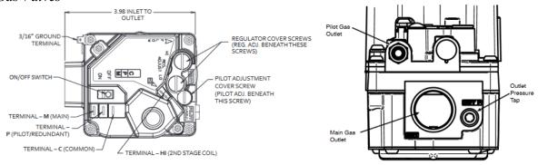
Figure 46 – Combination Gas Valve
