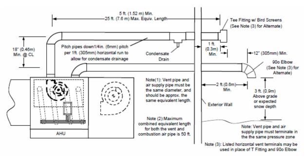
Figure 36 – Indoor Horizontal Venting Separated Combustion
