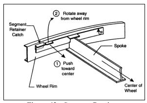
Figure 43 - Segment Retainer
