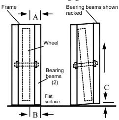
Figure 40 - Avoid Racking of Cassette Frame
