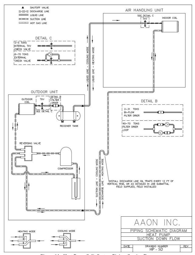
Figure 64 - Heat Pump Split System Piping, Suction Down
