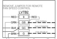
Figure 28 – Jumper for Remote Fan Speed Control
