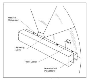
Figure 42 - Hub Seal Adjustment
