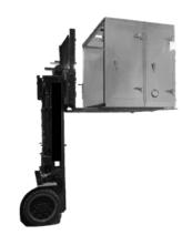
Figure 8 - M2 Series Individual Module Top Tier Lifting
