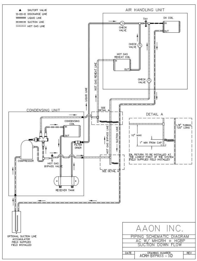
Figure 62 - A/C with Modulating Hot Gas Reheat and Hot Gas Bypass Split System Piping, Suction Down
