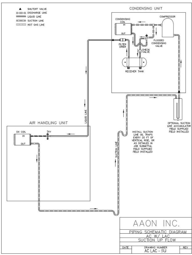
Figure 57 - A/C with LAC Split System Piping, Suction Up
