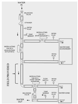
Figure 22 – Waterside Economizer Piping
