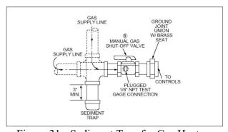
Figure 31 - Sediment Trap for Gas Heat
