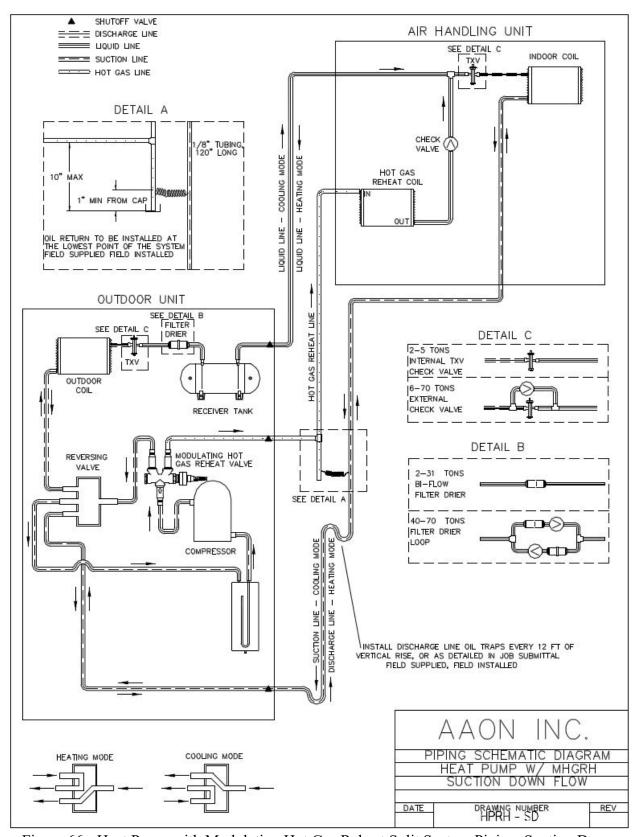
Figure 66 - Heat Pump with Modulating Hot Gas Reheat Split System Piping, Suction Down
