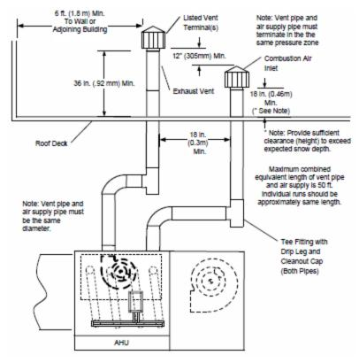
Figure 35 – Indoor Vertical Venting Separated Combustion
