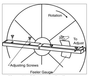
Figure 41 - Diameter Seal Adjustment
