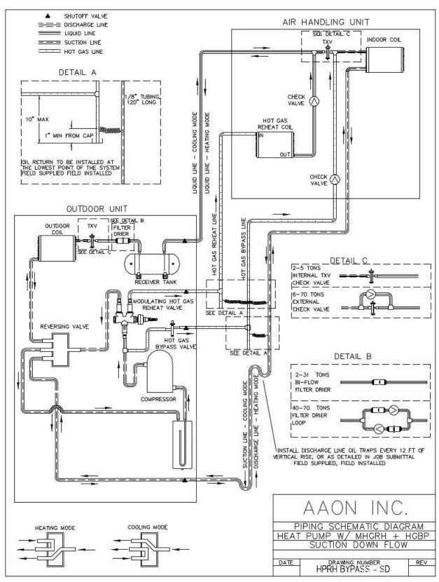
Figure 39 - Heat Pump with Modulating Hot Gas Reheat and Hot Gas Bypass Split System Piping, Suction Down
