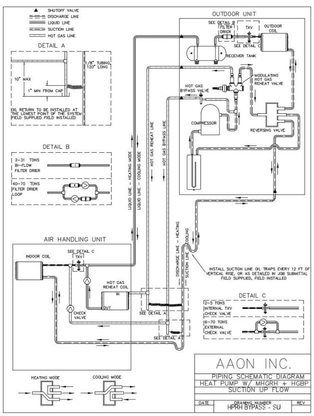
Figure 40 - Heat Pump with Modulating Hot Gas Reheat and Hot Gas Bypass Split System Piping, Suction Up
