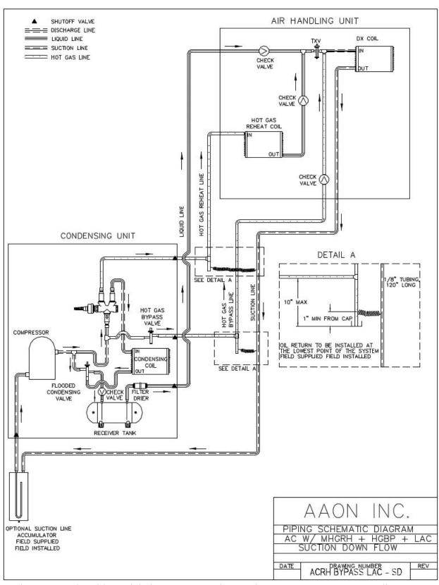
Figure 31 - A/C with Modulating Hot Gas Reheat and Hot Gas Bypass + LAC Split System Piping, Suction Down
