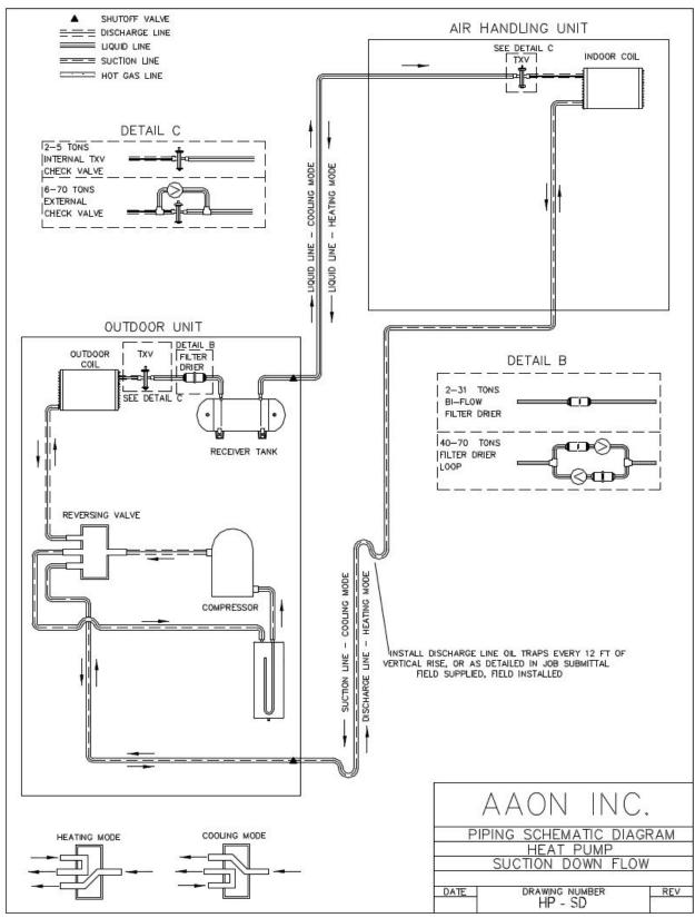
Figure 33 - Heat Pump Split System Piping, Suction Down
