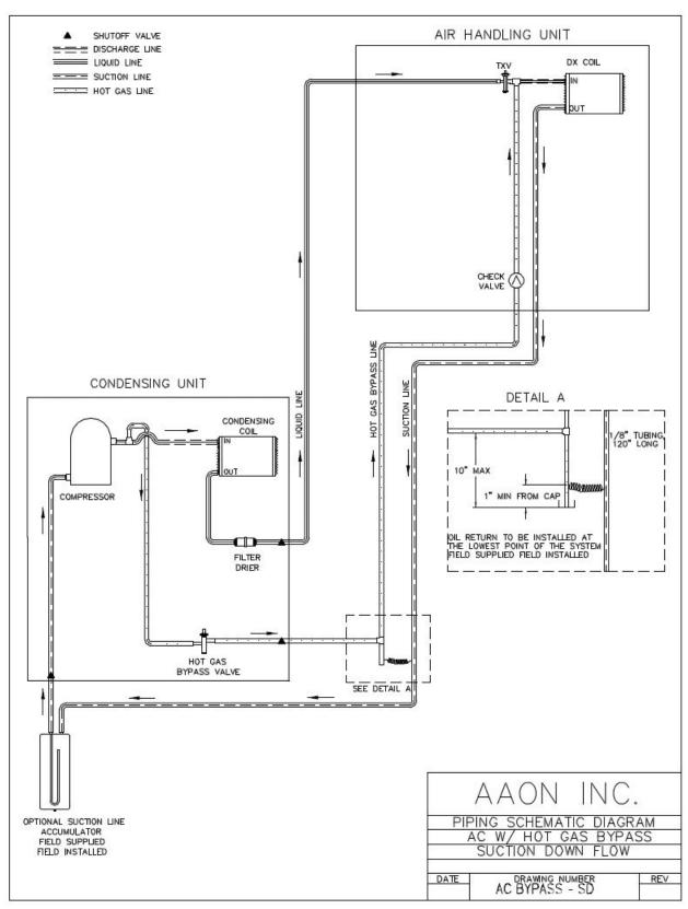
Figure 25 - A/C with Hot Gas Bypass Split System Piping, Suction Down
