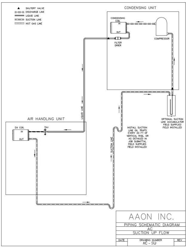
Figure 18 - A/C Split System Piping, Suction Up
