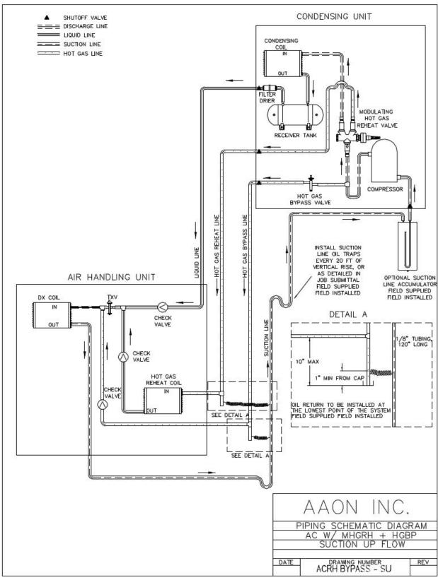
Figure 30 - A/C with Modulating Hot Gas Reheat and Hot Gas Bypass Split System Piping, Suction Up
