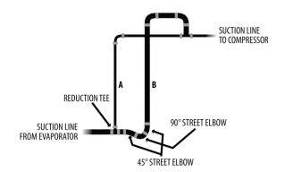
Figure 9 - Double Suction Riser Construction
