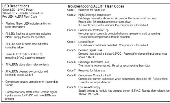
Figure 14 - Compressor Controller Flash Code Details
