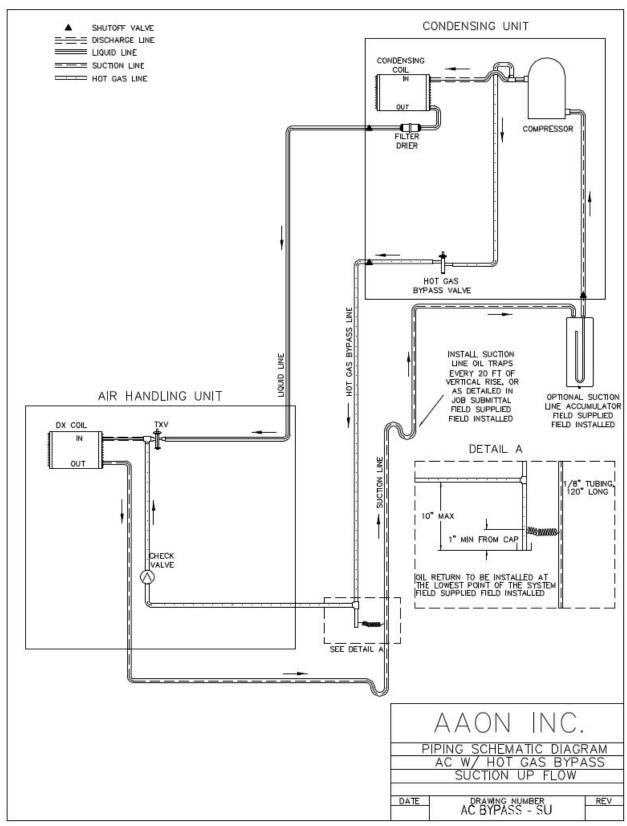
Figure 26 - A/C with Hot Gas Bypass Split System Piping, Suction Up
