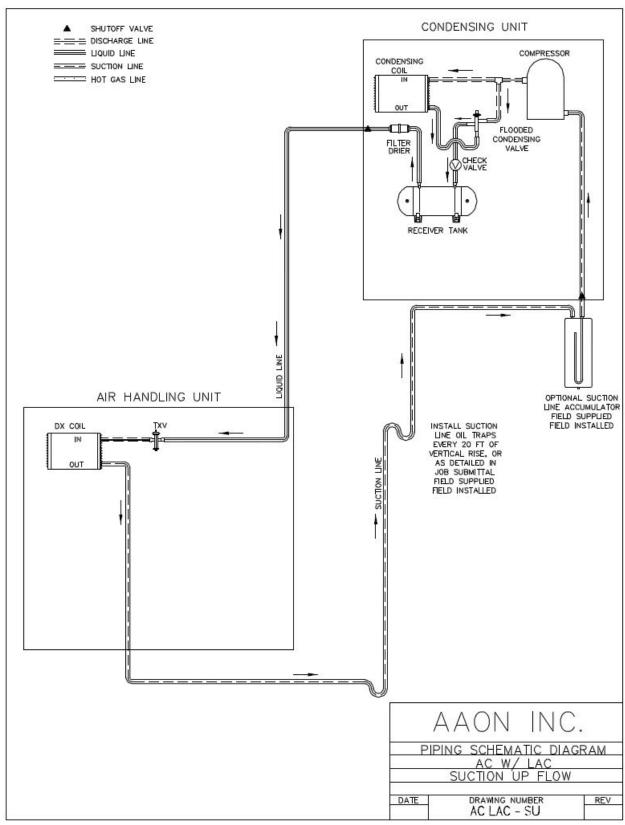
Figure 20 - A/C with LAC Split System Piping, Suction Up
