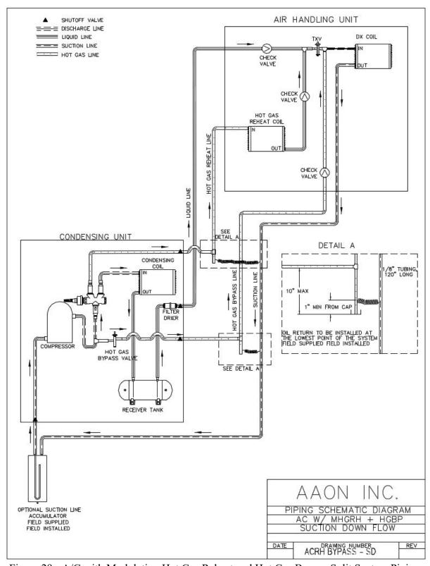
Figure 29 - A/C with Modulating Hot Gas Reheat and Hot Gas Bypass Split System Piping, Suction Down
