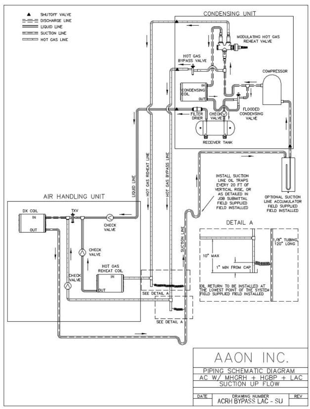
Figure 32 - A/C with Modulating Hot Gas Reheat and Hot Gas Bypass + LAC Split System Piping, Suction Up
