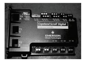
Figure 13 - Variable Capacity Compressor Controller
