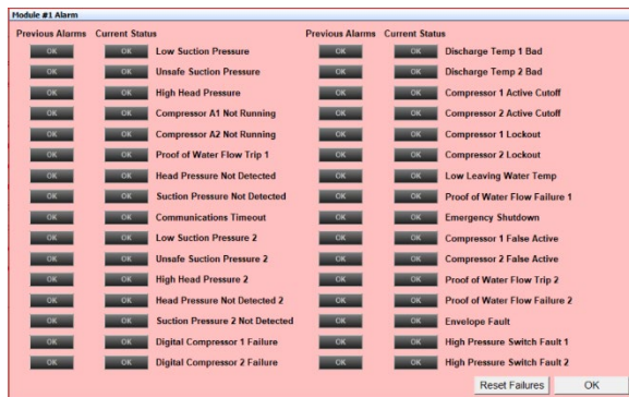
Figure 25: Prism 2 Compressor Alarms Screen
