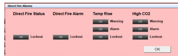
Figure 23: Prism 2 Direct Fire Alarms Screen
