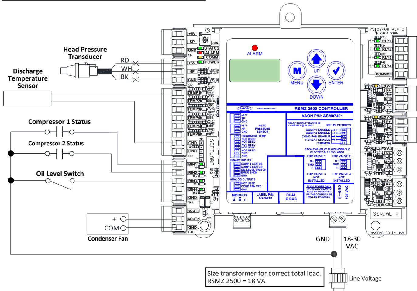
Figure 4: RSMZ 2500 Inputs Wiring - Modules 3 and 6
