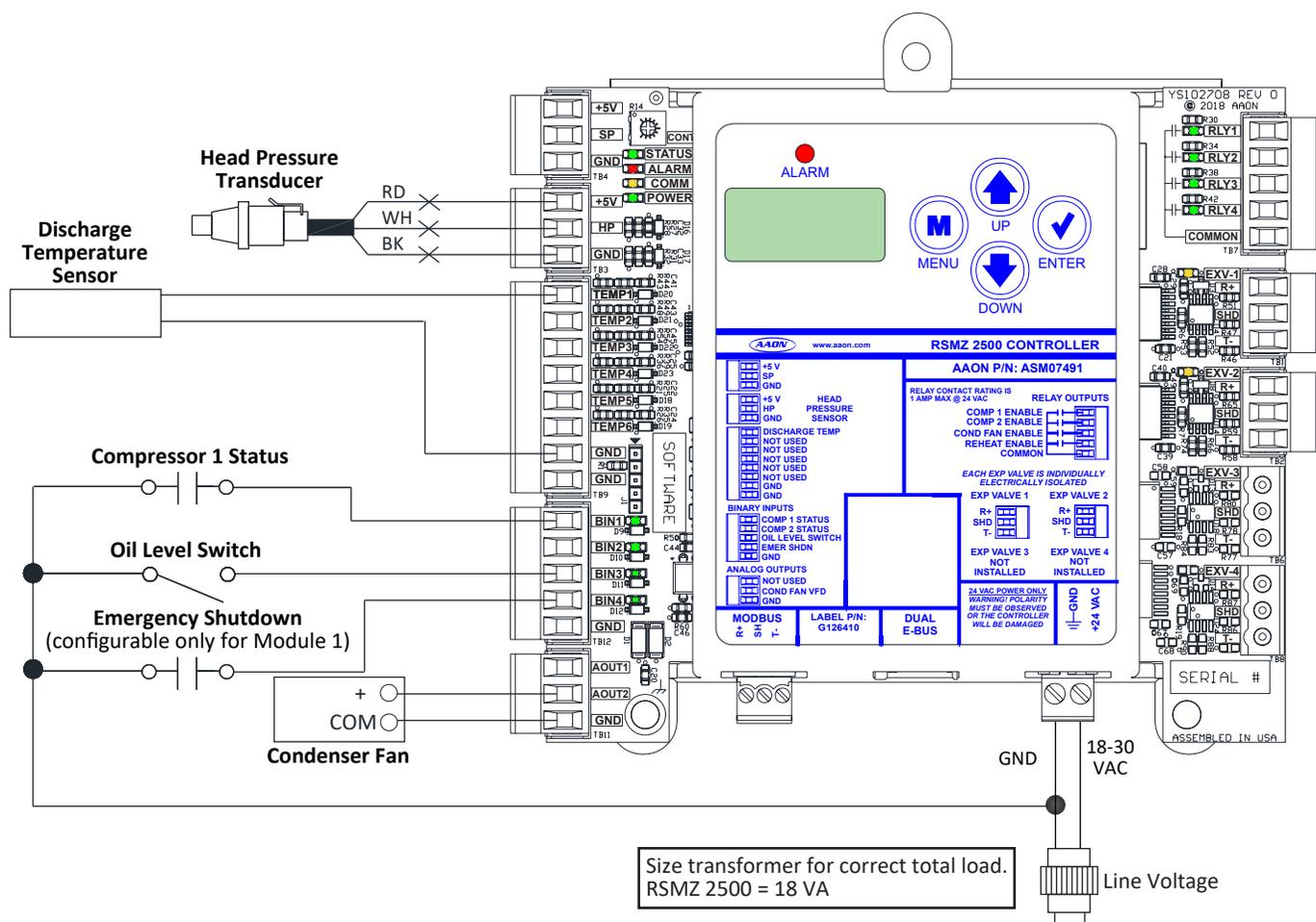
Figure 2: RSMZ 2500 Inputs Wiring - Modules 1, 2, 4, and 5
