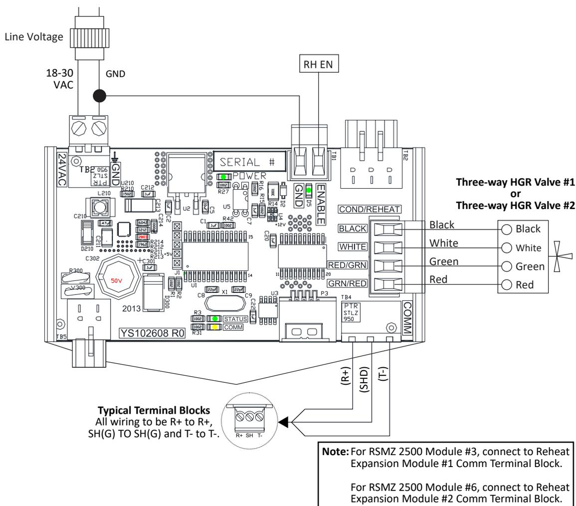
**Figure 6: Reheat Expansion Module #1 or #2 Wiring**
