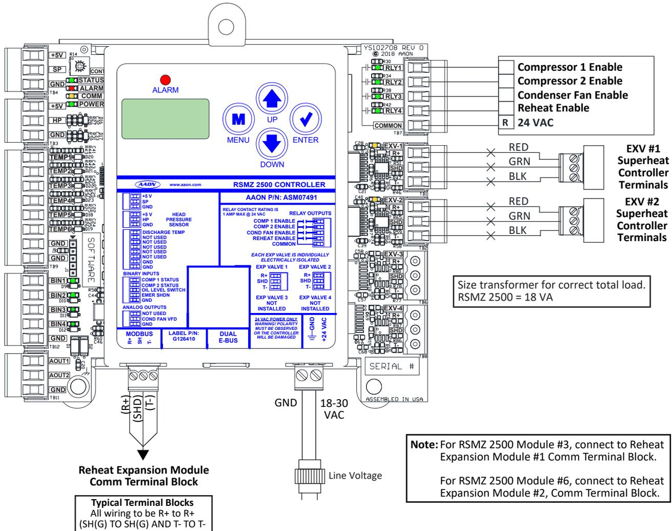
Figure 5: RSMZ 2500 Outputs Wiring - Modules 3 and 6
