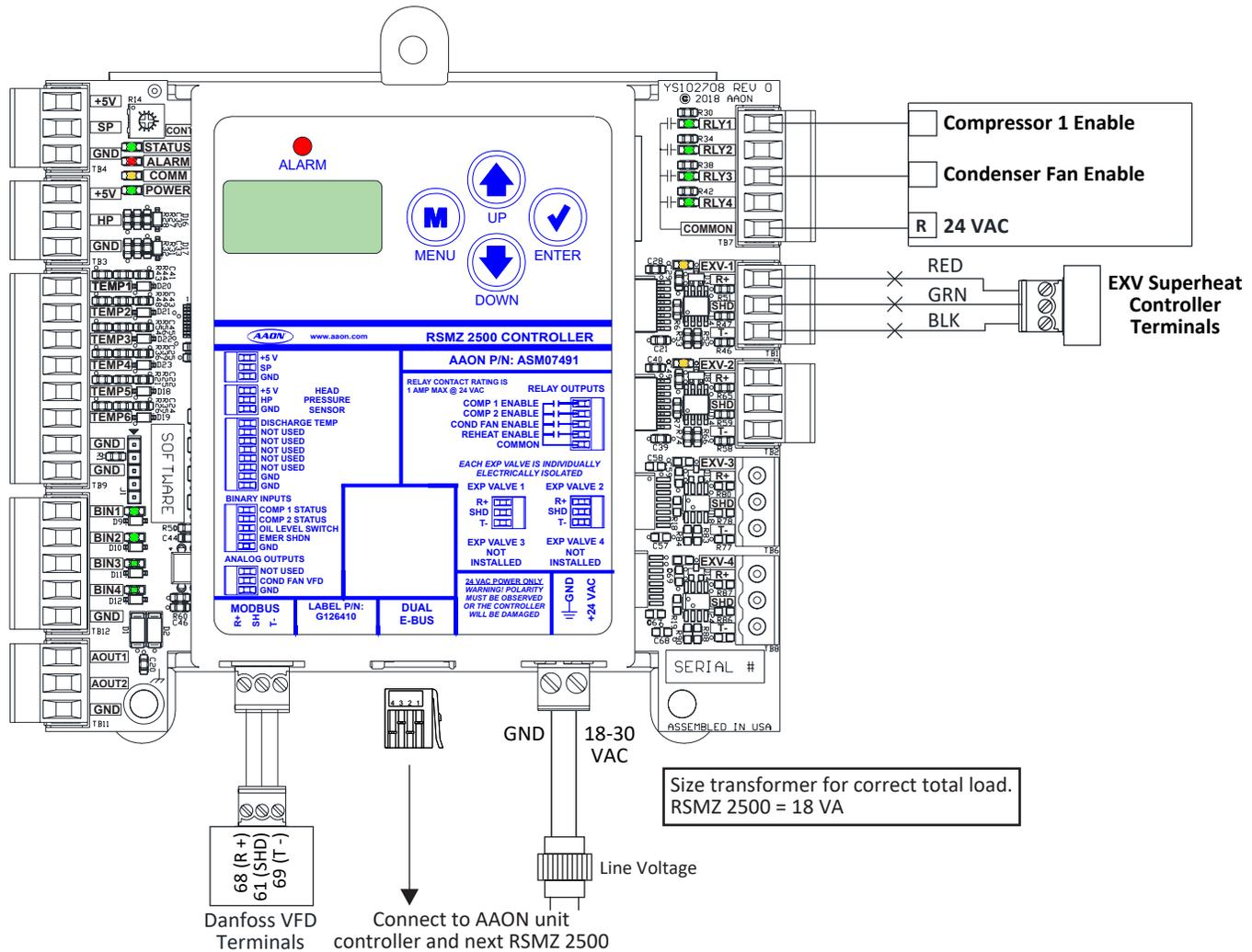
**Figure 3: RSMZ 2500 Outputs Wiring - Modules 1, 2, 4, and 5**
