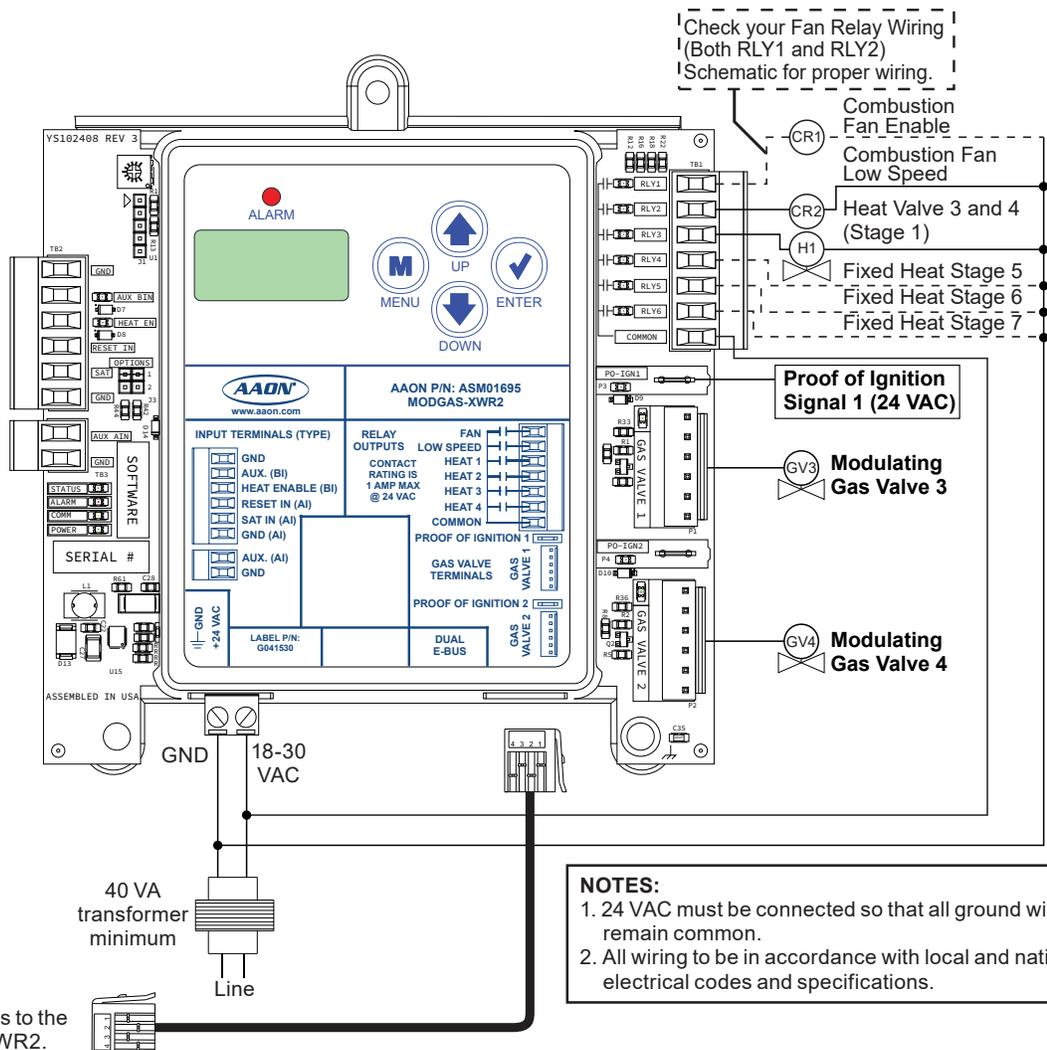
**Figure 14: Communications Wiring - Secondary Board 2V1IGN1S**
