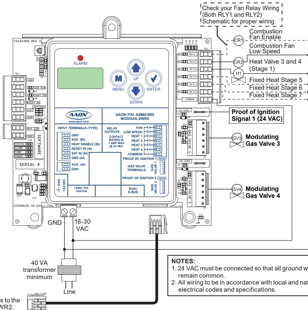
**Figure 6: Stand-Alone Wiring - Secondary Board 2V1IGN1S**
