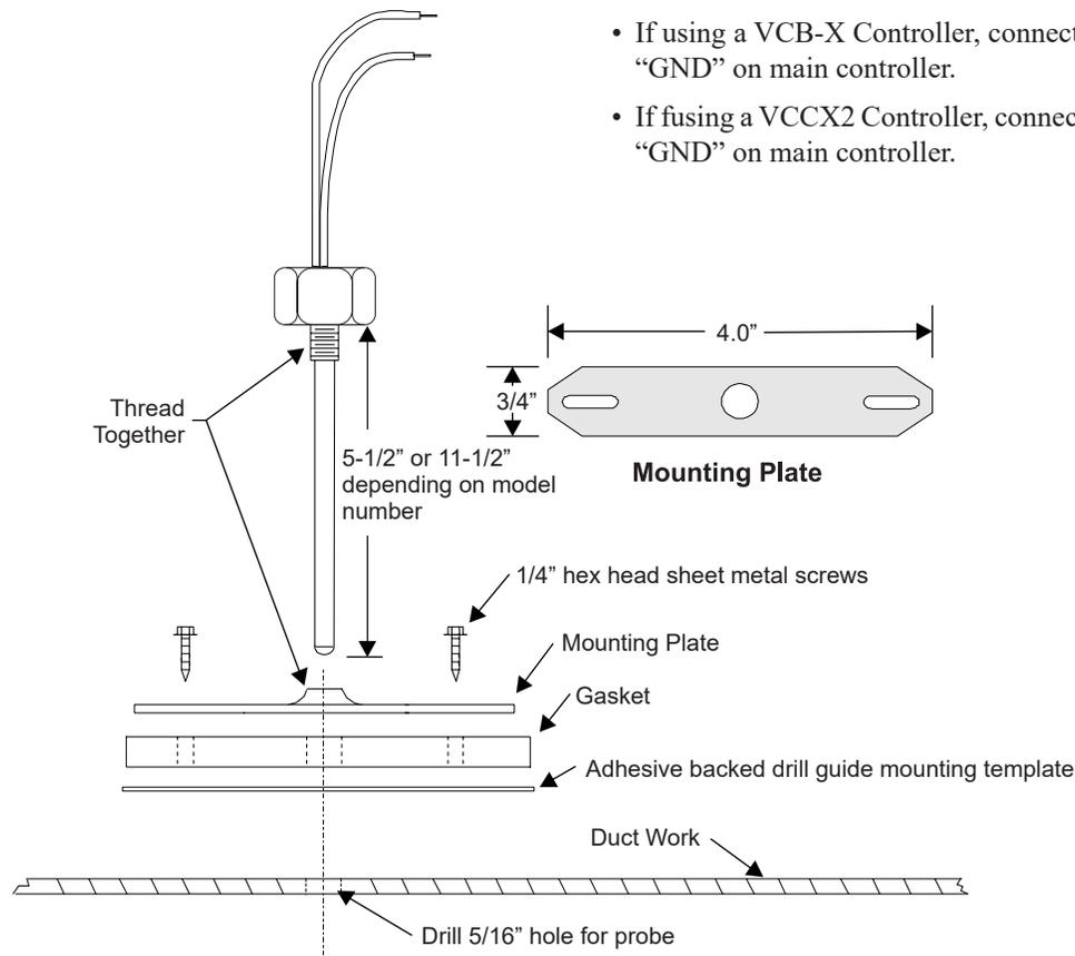
Figure 17: Supply Air Temperature Sensor Installation
