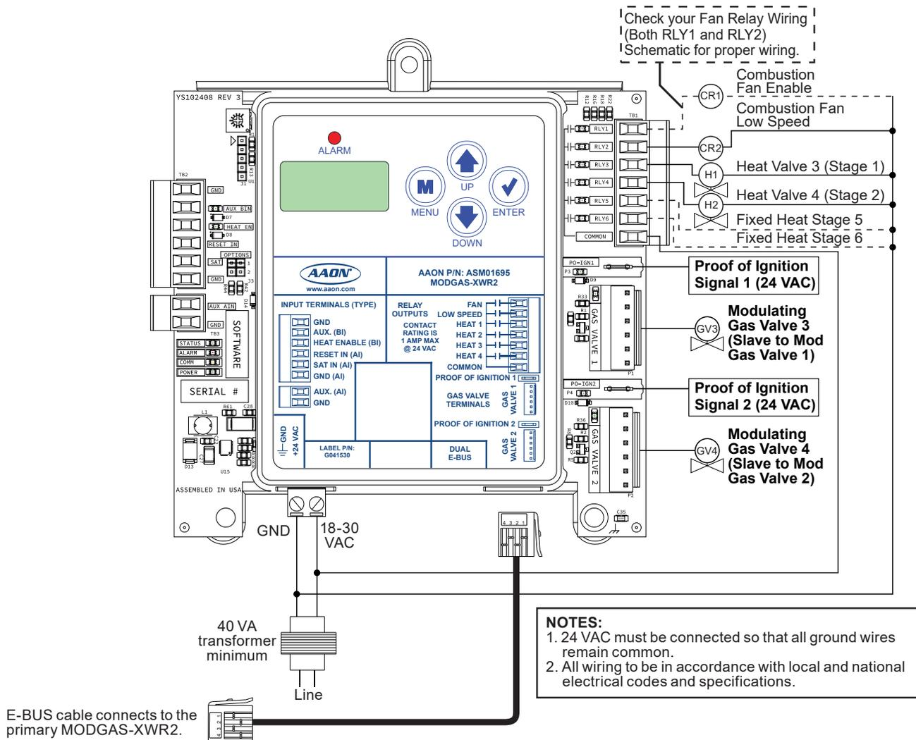
**Figure 12: Communications Wiring - Secondary Board 2V2IGN2S**
