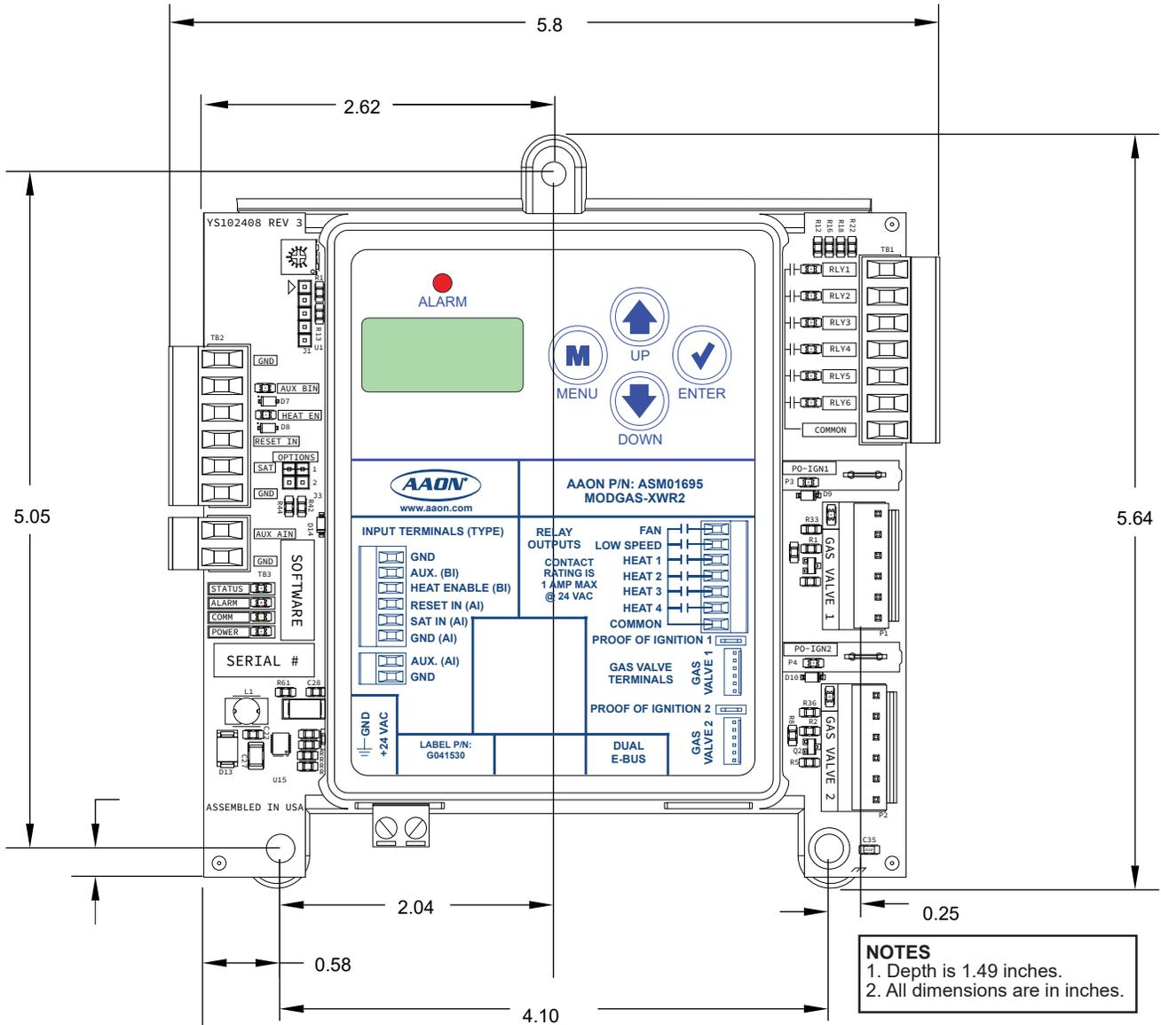
Figure 1: MODGAS-XWR2 Module Dimensions
