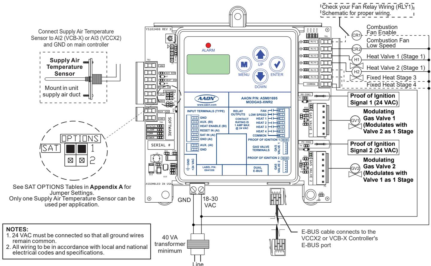
Figure 10: Communications Wiring - One Modulating Valve, Two Ignitors, One Stage
