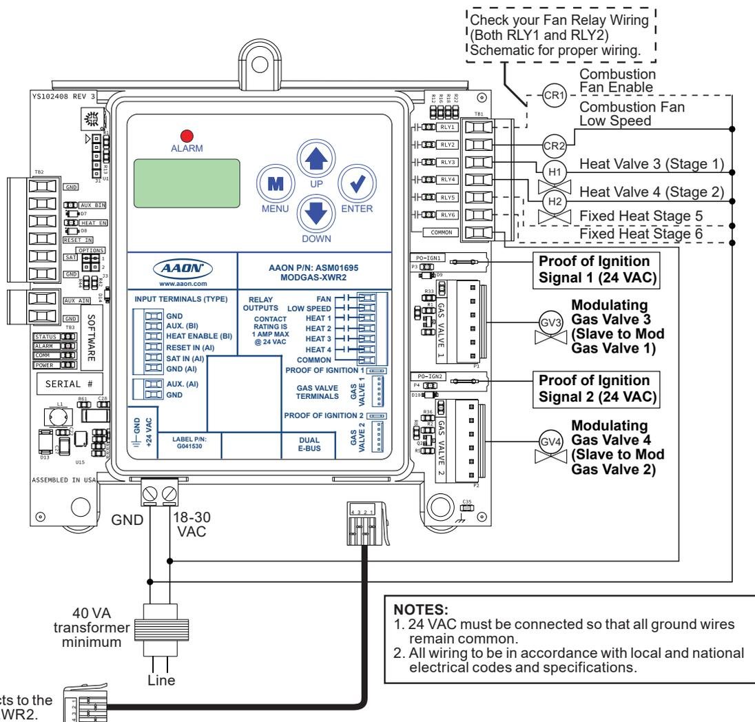
**Figure 4: Stand-Alone Wiring - Secondary Board 2V2IGN2S**
