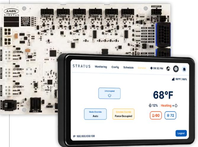
To fully realize the potential of EXTREME SERIES, we created Stratus — a complete rethinking of AAON controls. Stratus simplifies installation and maintenance with intuitive touchscreen controls, streamlined startup, directive troubleshooting, and full remote monitoring. Built as an extensible platform, Stratus is designed to grow with advancing technology, offering future-ready performance analytics.
