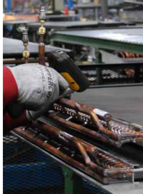
Condenser coil being scanned prior to leak testing. The results of this test, pass or fail, are stored electronically for further analysis to ensure quality control.
