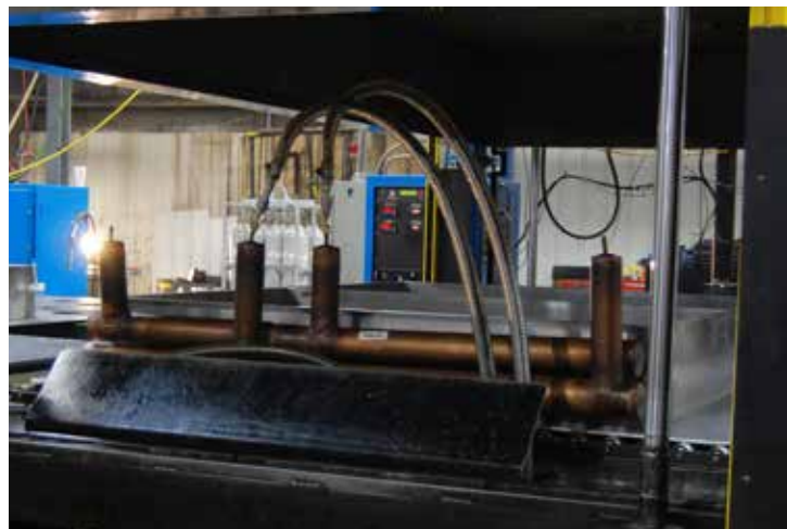
Leak test chamber where coils go through gross leak and trace gas leak testing.
